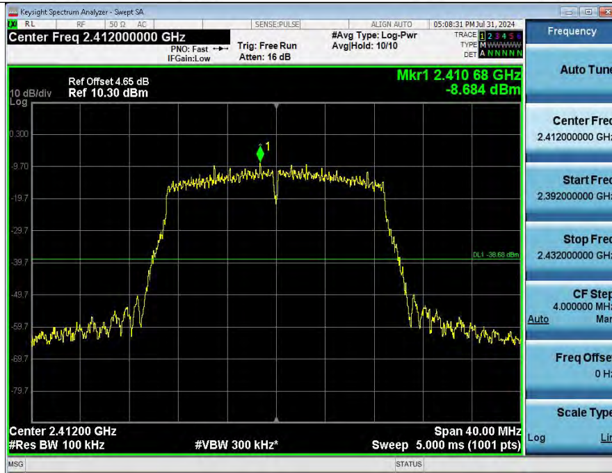
1 Reference Level NVNT_ANT2_802_11n(HT20)_2412
