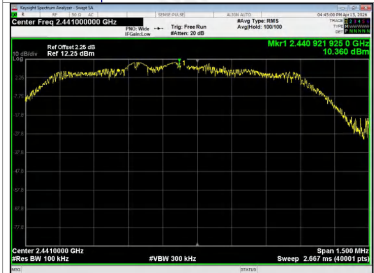
Tx. Spurious NVNT 3-DH1 2441MHz Ref
