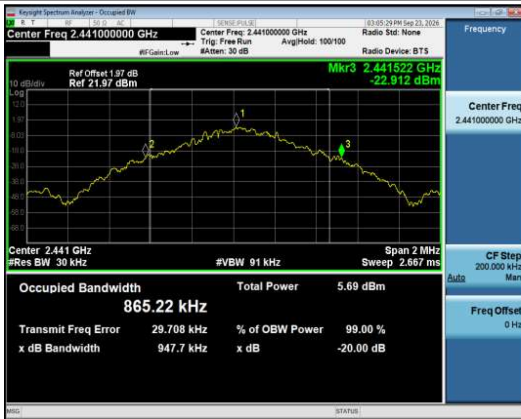
-20dB Bandwidth NVNT 1-DH5 2441MHz Ant1
