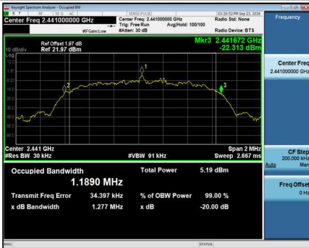
-20dB Bandwidth NVNT 3-DH5 2441MHz Ant1
