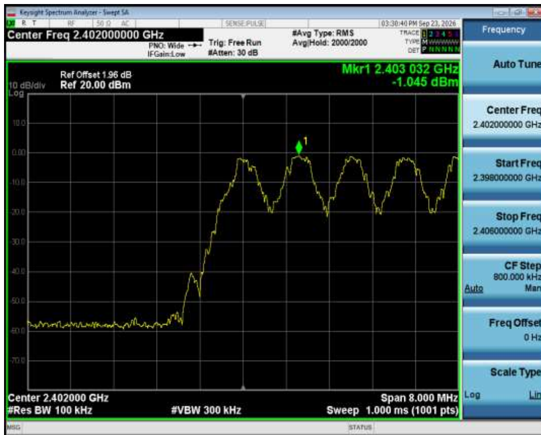
Band Edge(Hopping) NVNT 1-DH5 2402MHz Ant1 Hopping Ref
