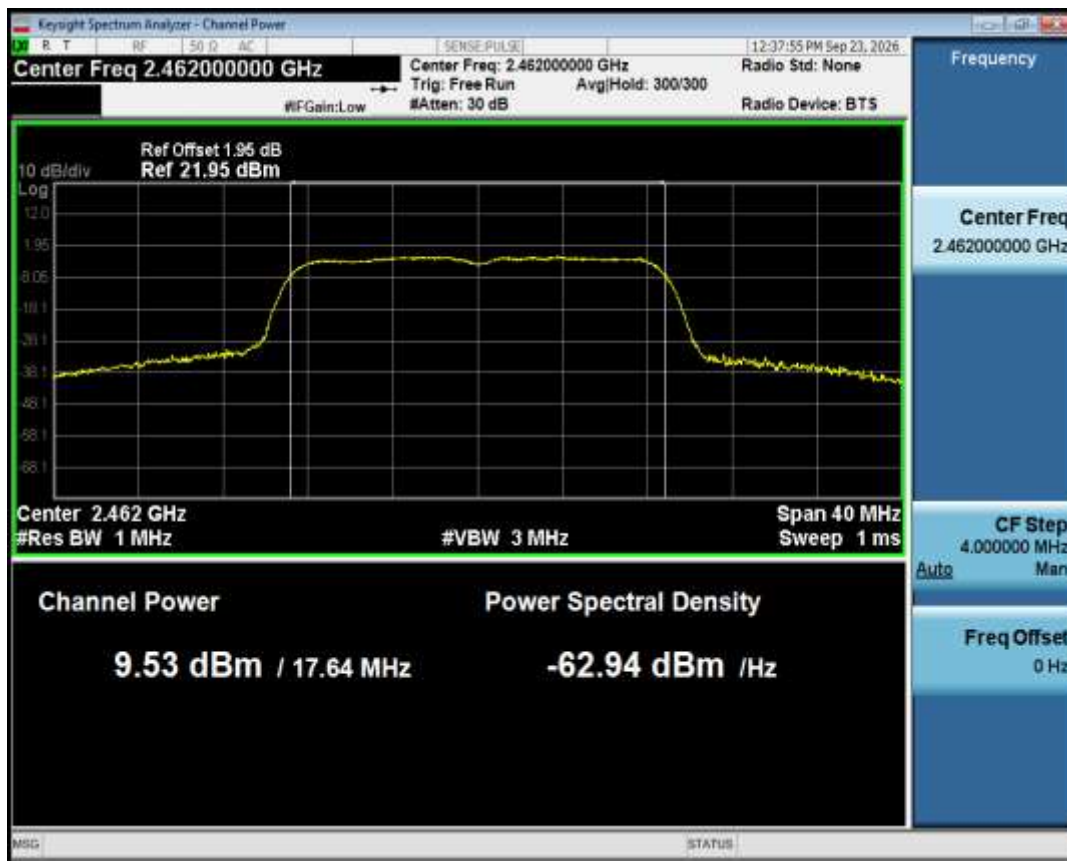
Average Power NVNT n20 2462MHz Ant1
