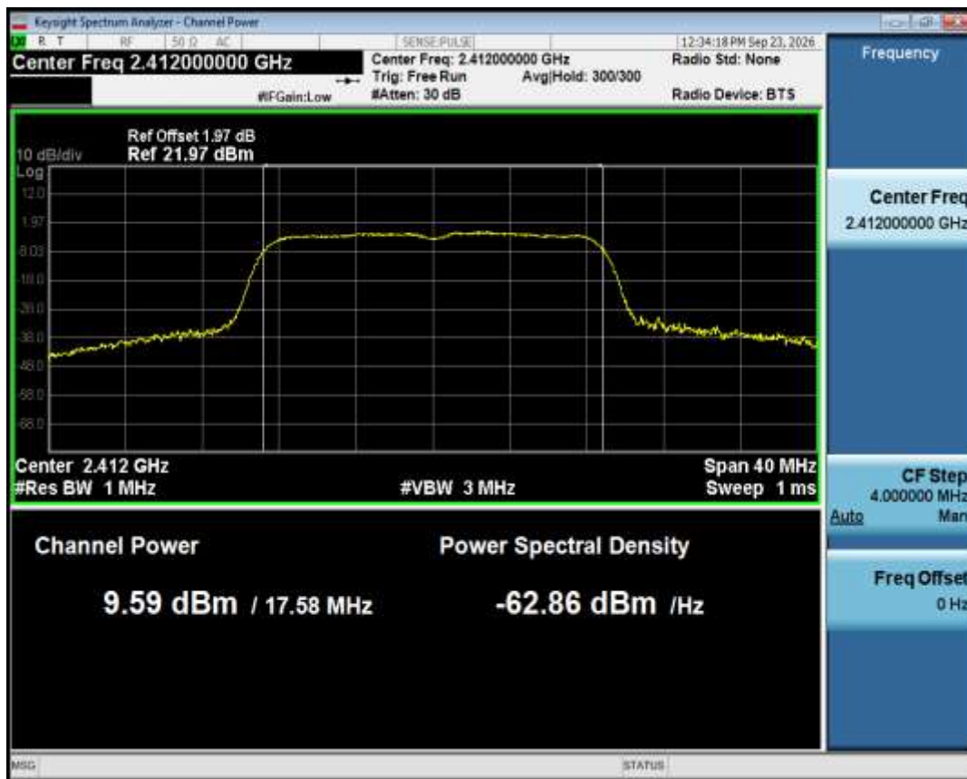
Average Power NVNT n20 2412MHz Ant1
