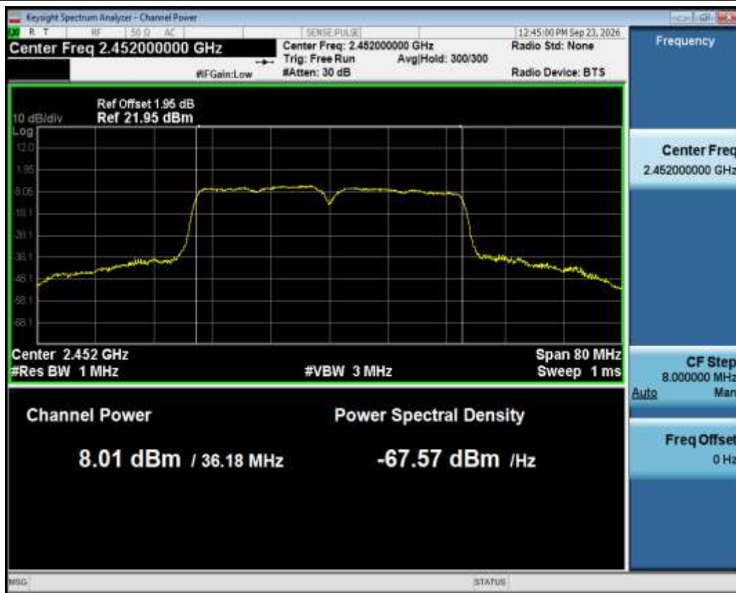
Average Power NVNT n40 2452MHz Ant1
