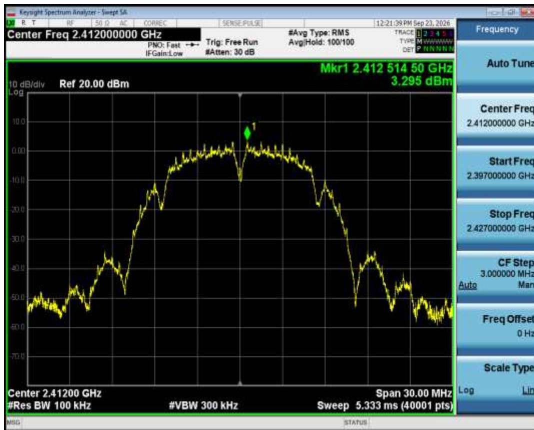
Tx. Spurious NVNT b 2412MHz Ant1 Ref
