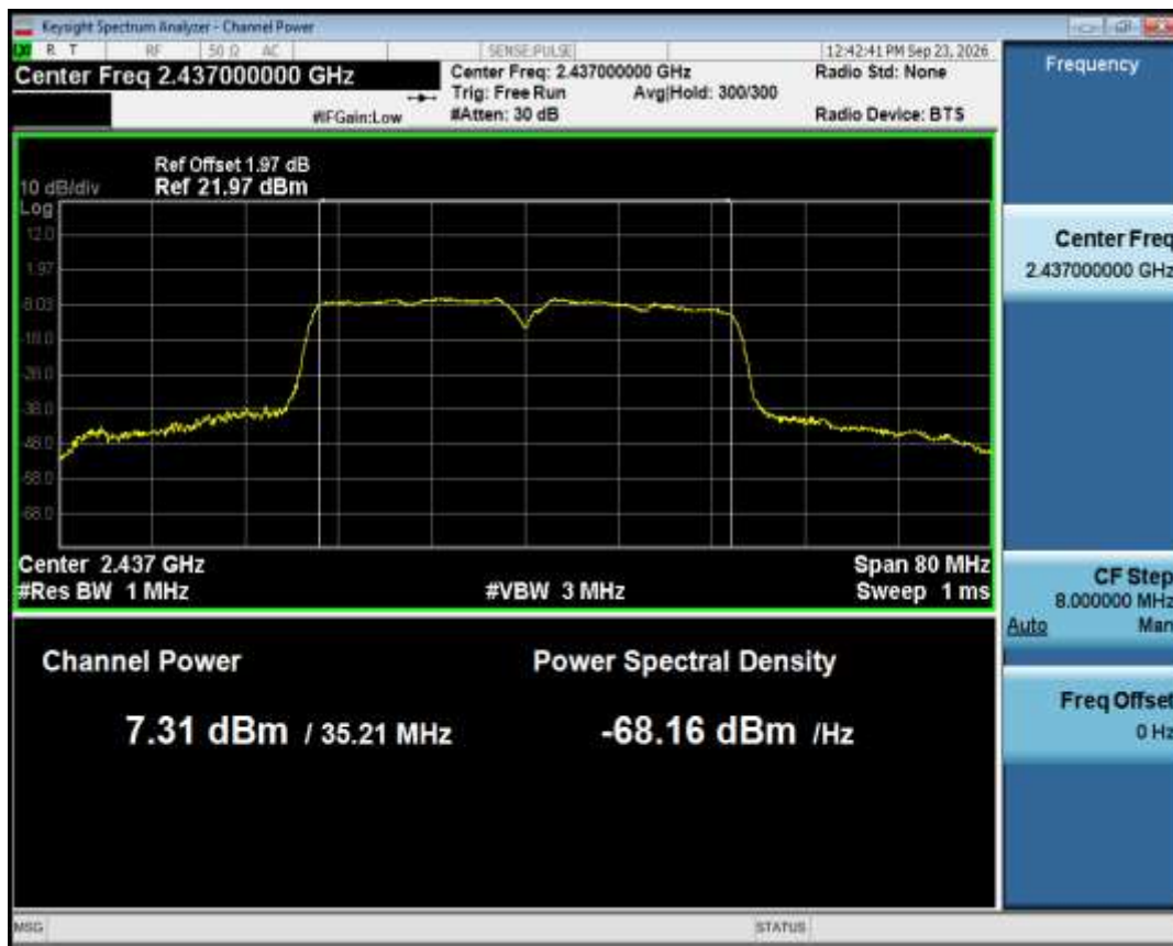
Average Power NVNT n40 2437MHz Ant1
