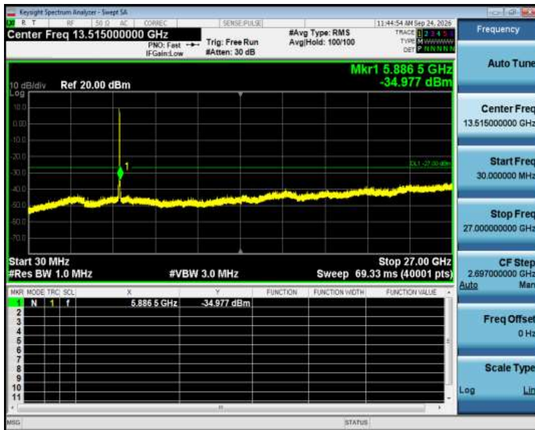
Tx. Spurious NVNT ac20 5825MHz Ant1 Emission
