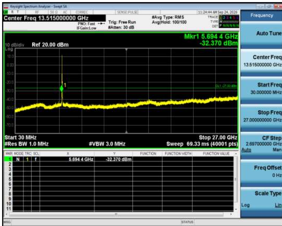
Tx. Spurious NVNT a 5745MHz Ant1 Emission
