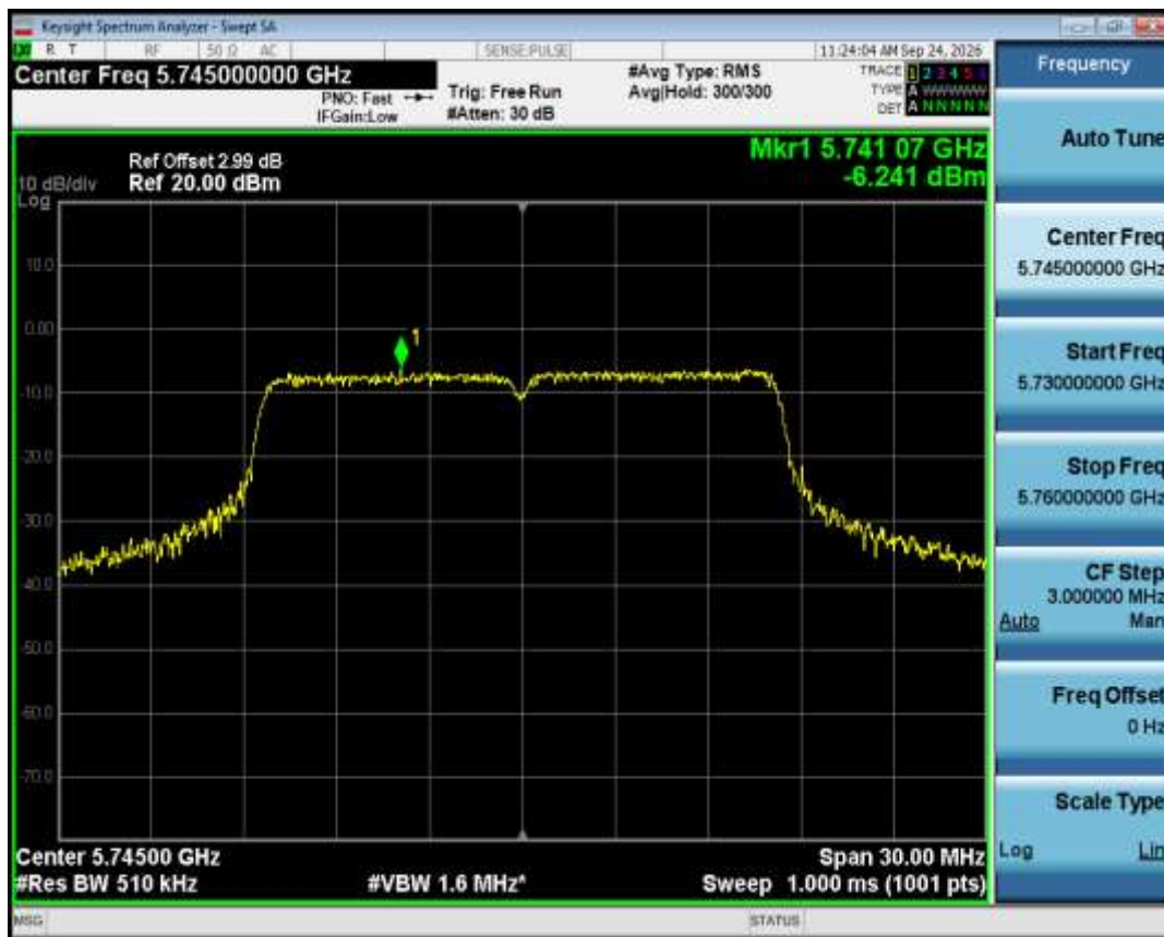
PSD NVNT a 5745MHz Ant1
