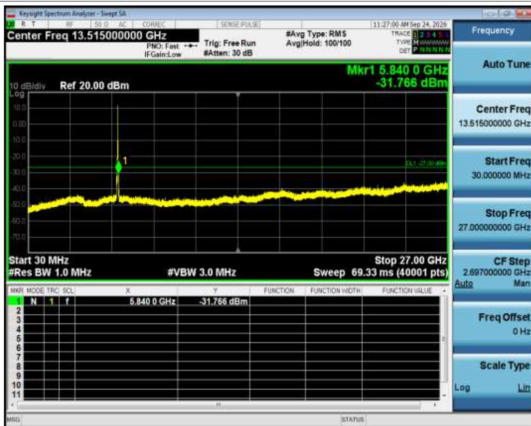
Tx. Spurious NVNT a 5785MHz Ant1 Emission
