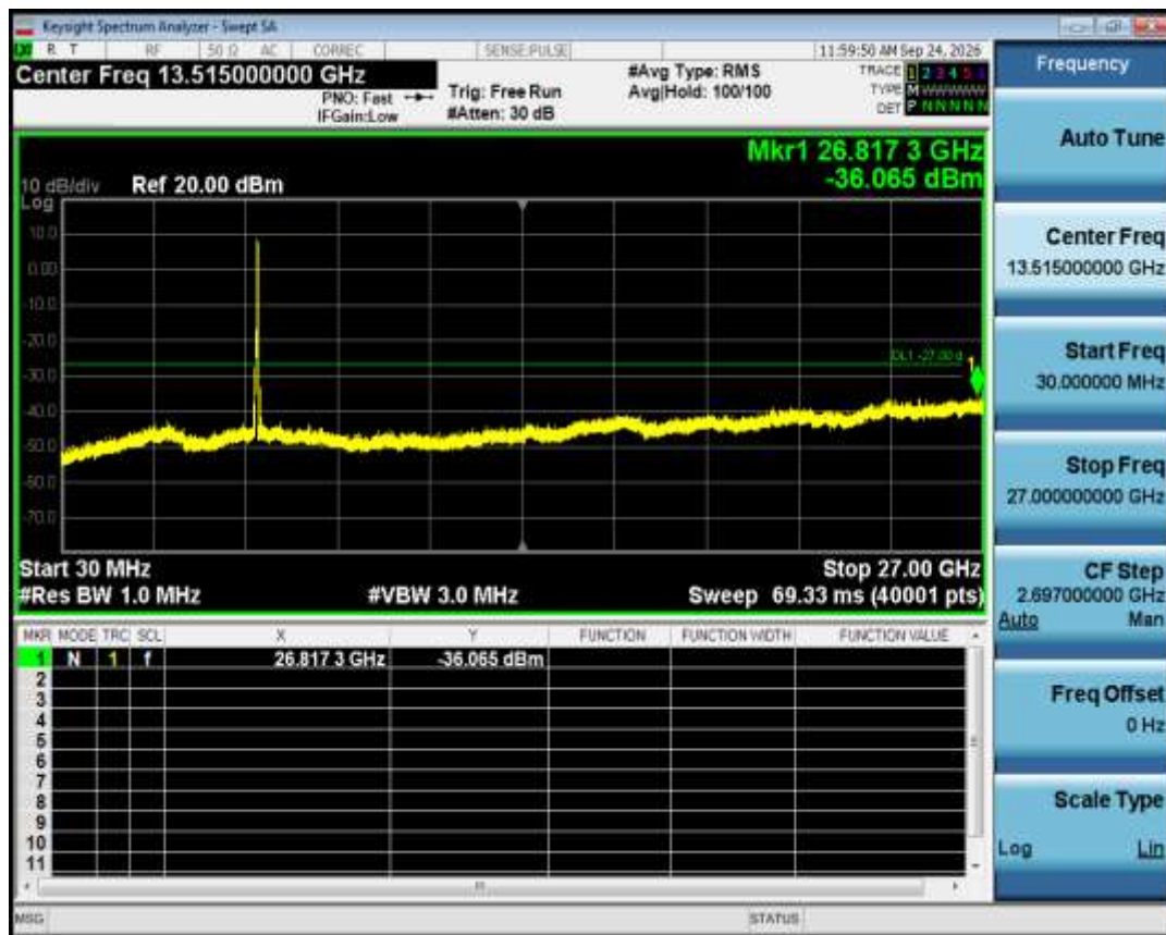
Tx. Spurious NVNT n40 5755MHz Ant1 Emission
