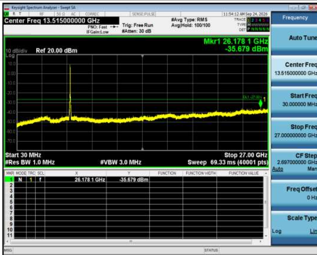
Tx. Spurious NVNT ac40 5755MHz Ant1 Emission
