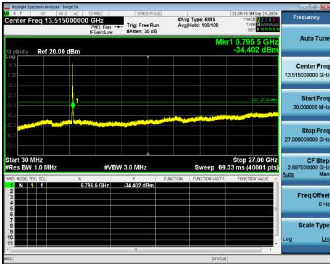
Tx. Spurious NVNT ac20 5745MHz Ant1 Emission
