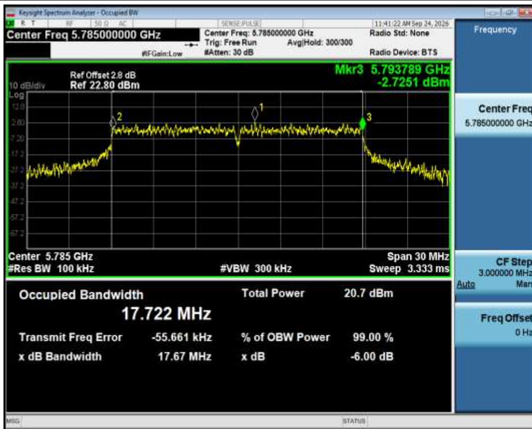
-6dB Bandwidth NVNT ac20 5785MHz Ant1
