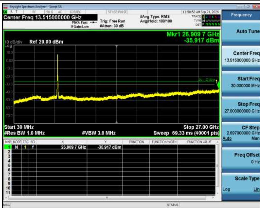
Tx. Spurious NVNT n40 5795MHz Ant1 Emission
