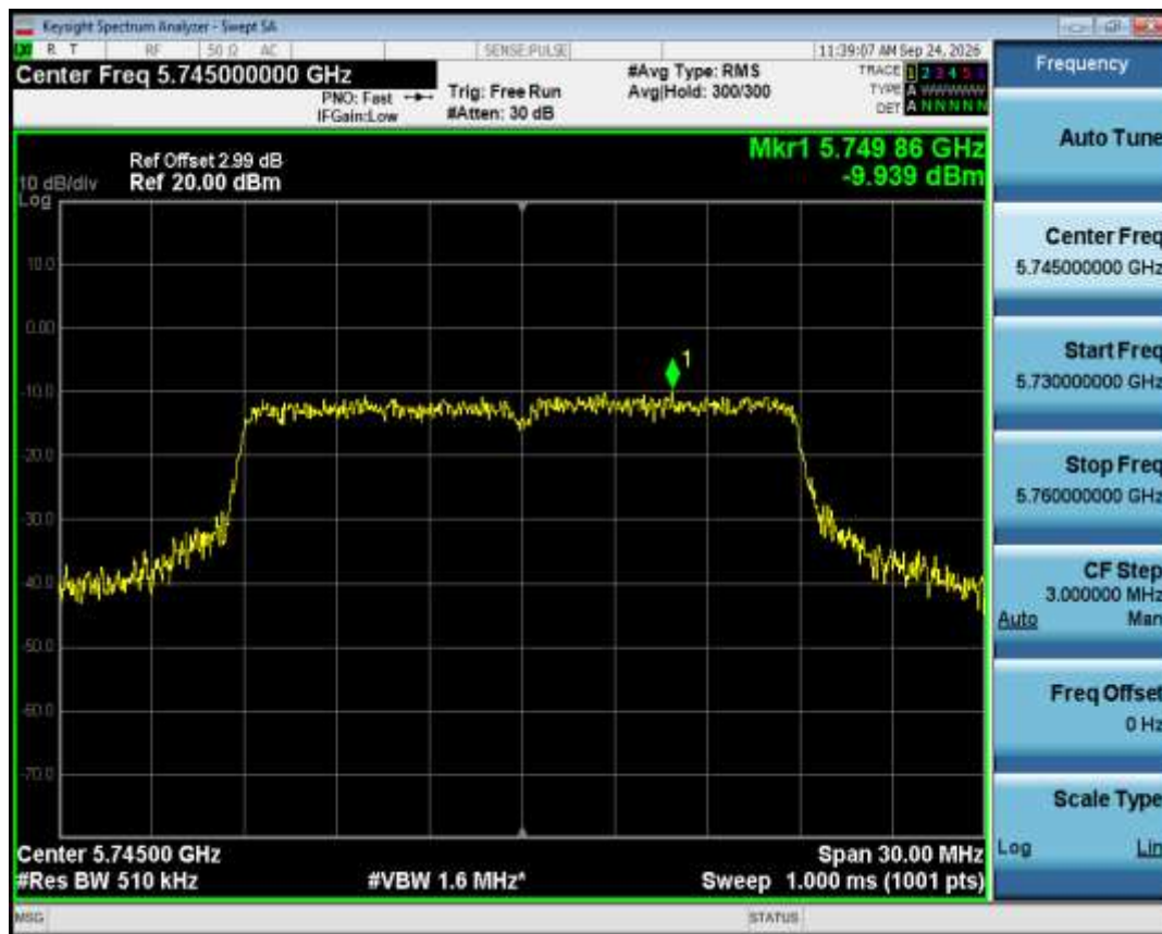
PSD NVNT ac20 5745MHz Ant1
