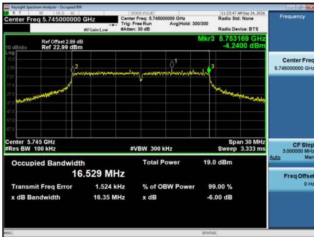
-6dB Bandwidth NVNT a 5745MHz Ant1
