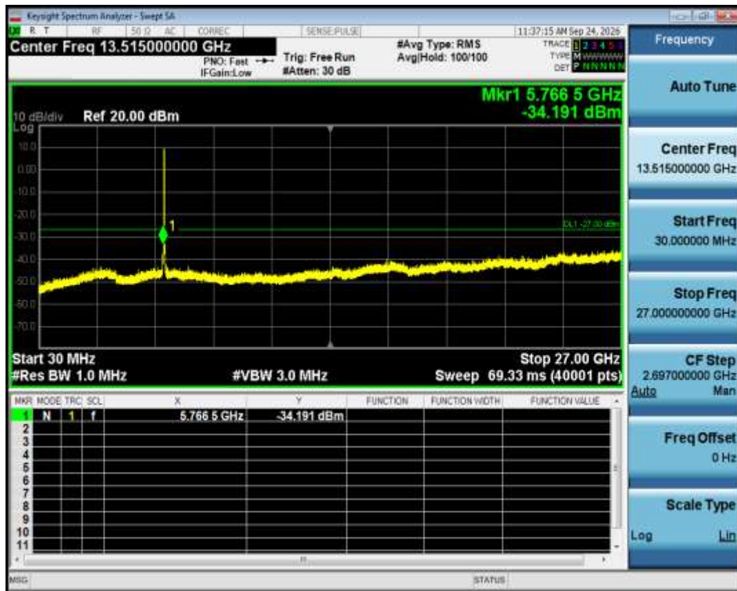
Tx. Spurious NVNT n20 5825MHz Ant1 Emission
