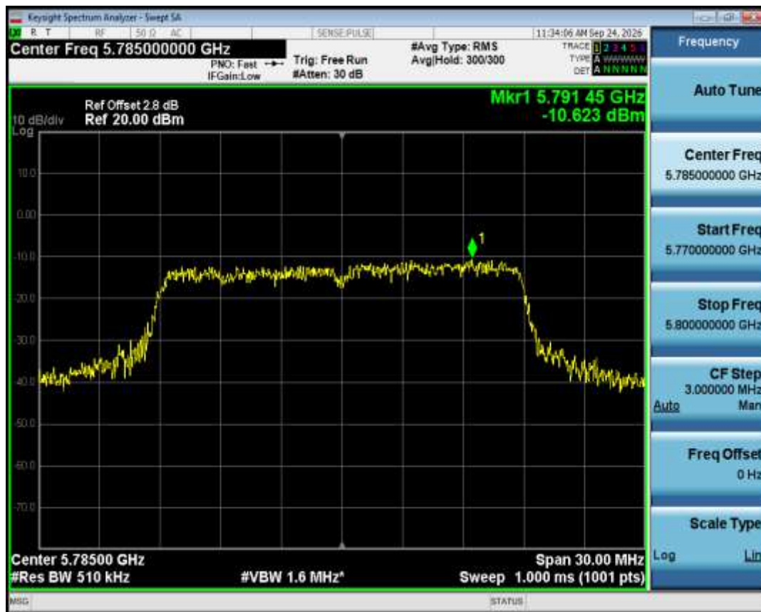
PSD NVNT n20 5785MHz Ant1
