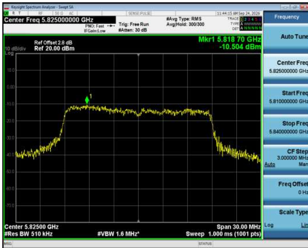
PSD NVNT ac20 5825MHz Ant1
