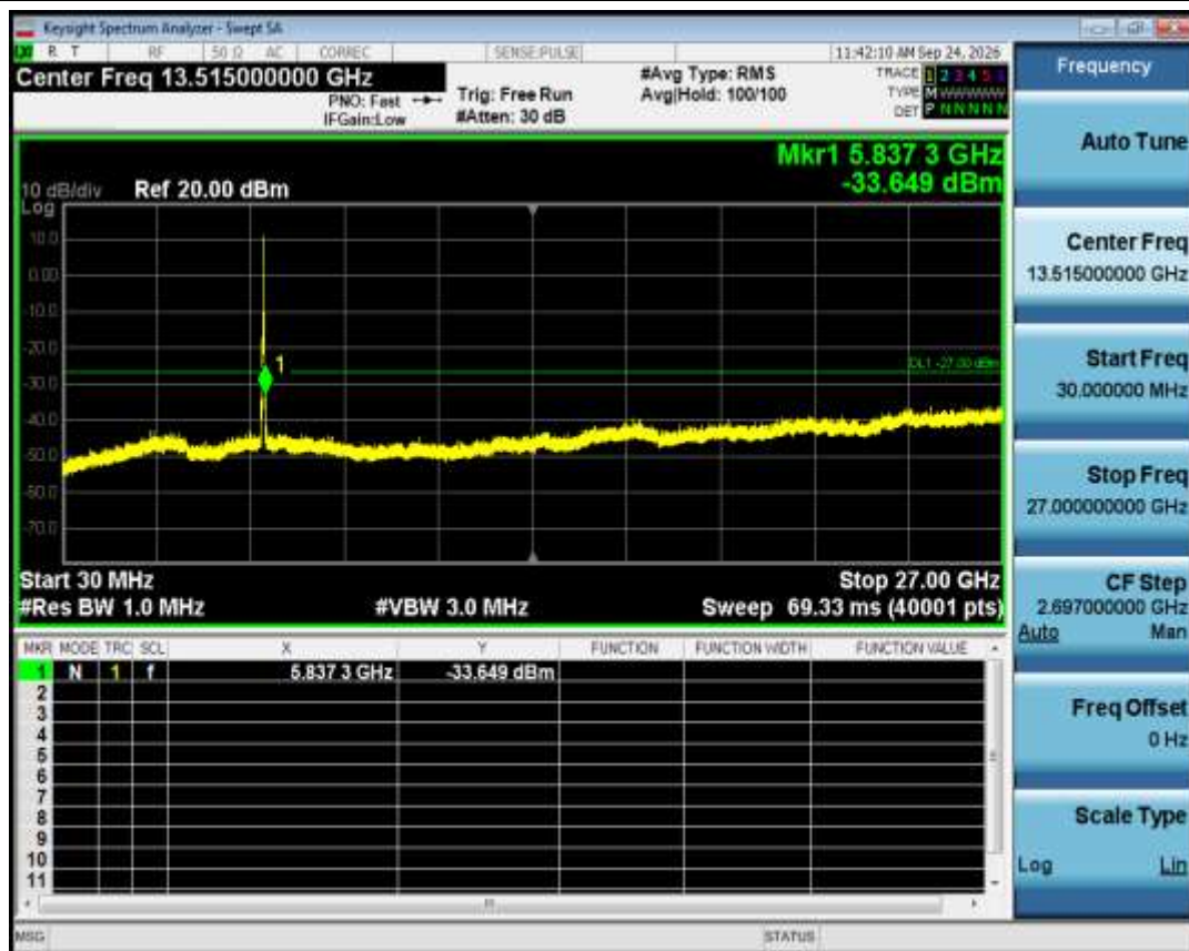
Tx. Spurious NVNT ac20 5785MHz Ant1 Emission
