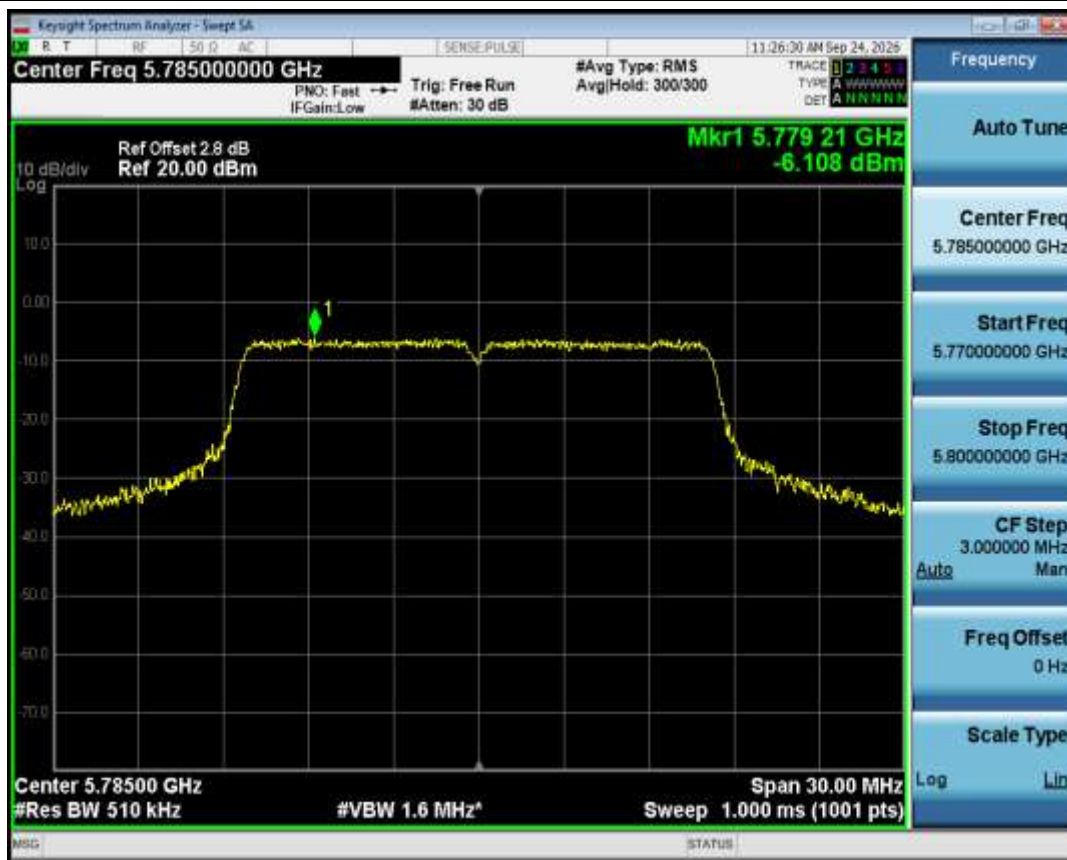
PSD NVNT a 5785MHz Ant1
