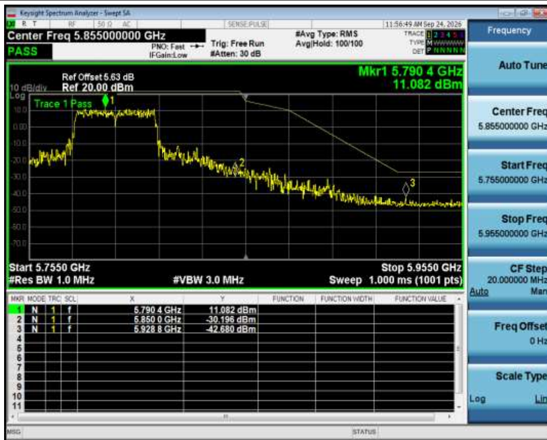
Band Edge NVNT ac40 5795MHz High Ant1
