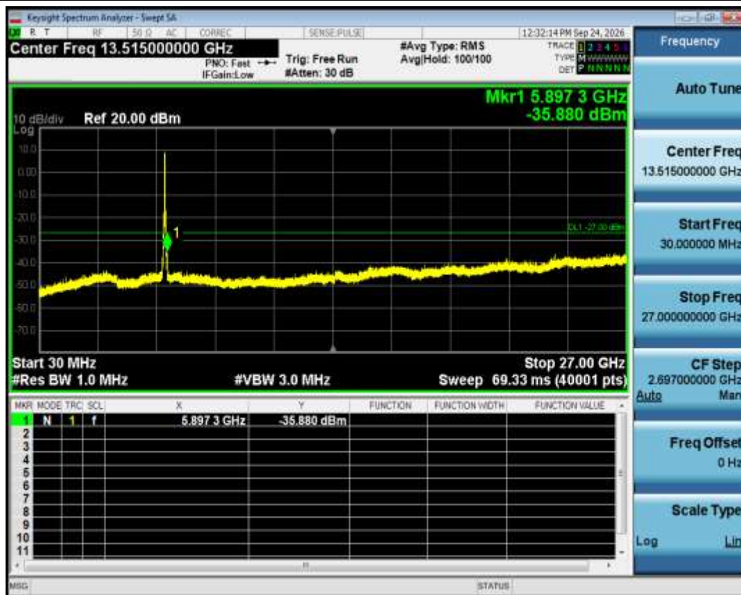
Tx. Spurious NVNT n40 5795MHz Ant1 Emission
