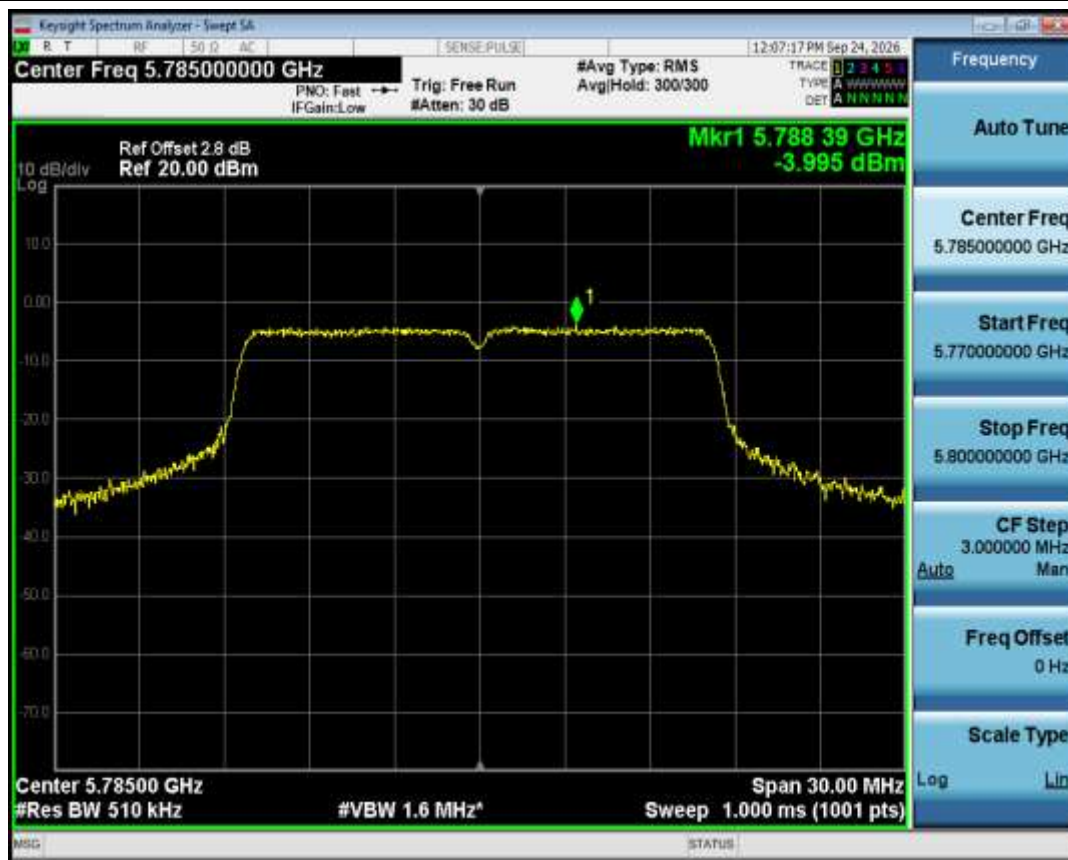
PSD NVNT a 5785MHz Ant1
