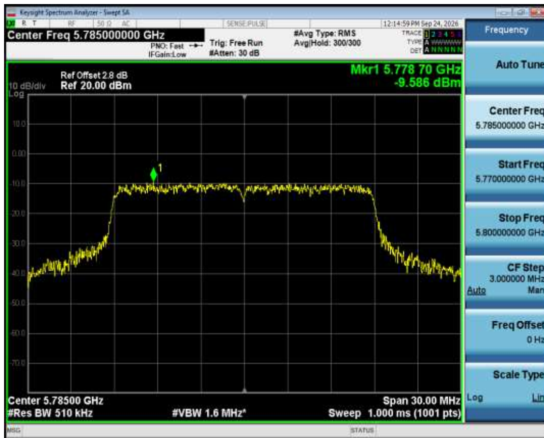
PSD NVNT n20 5785MHz Ant1
