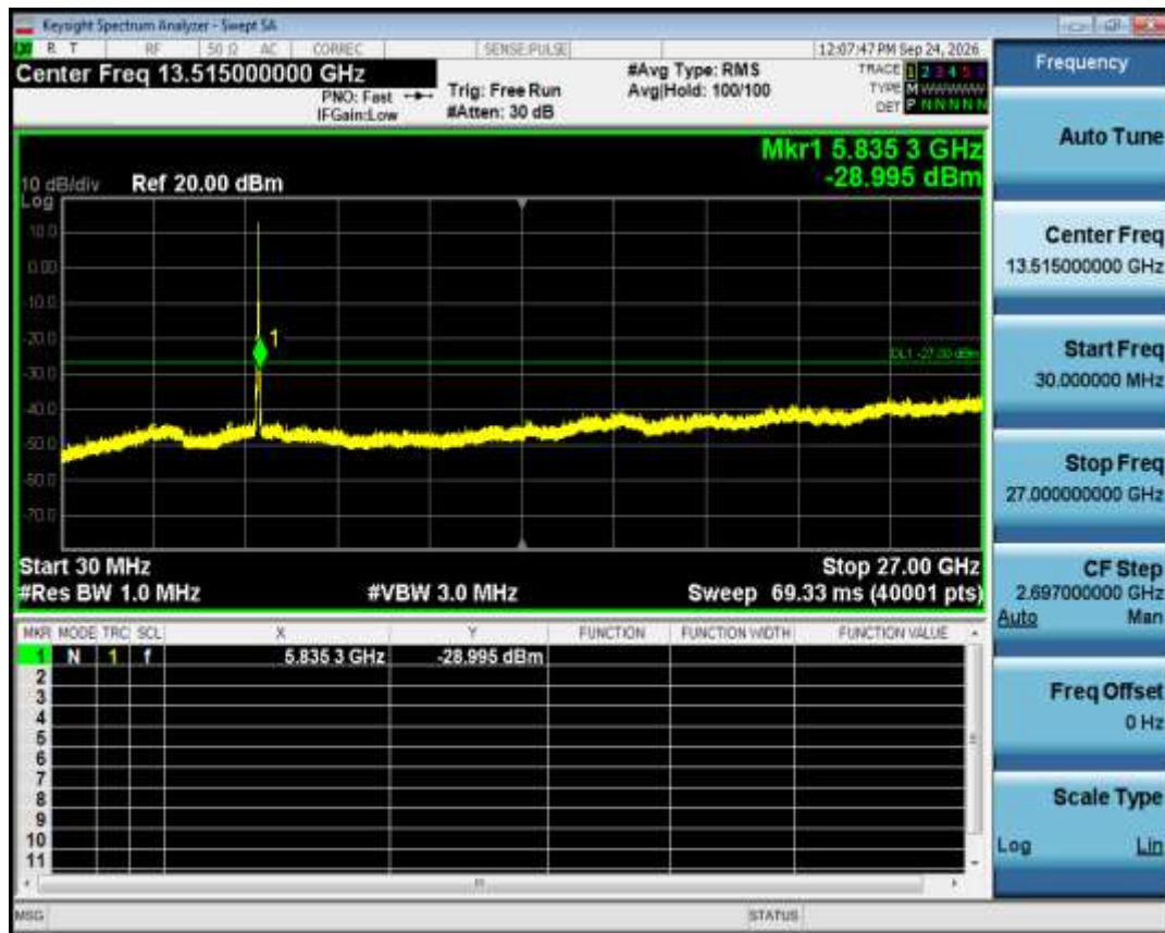
Tx. Spurious NVNT a 5785MHz Ant1 Emission
