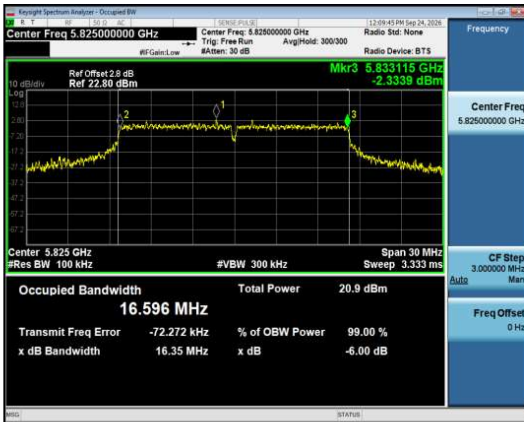
-6dB Bandwidth NVNT a 5825MHz Ant1
