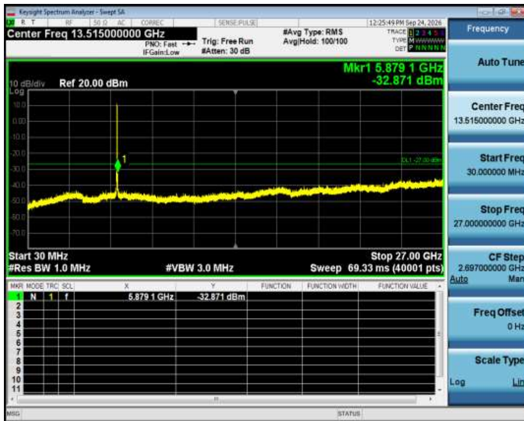
Tx. Spurious NVNT ac20 5825MHz Ant1 Emission
