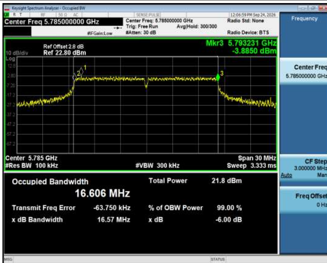
-6dB Bandwidth NVNT a 5785MHz Ant1
