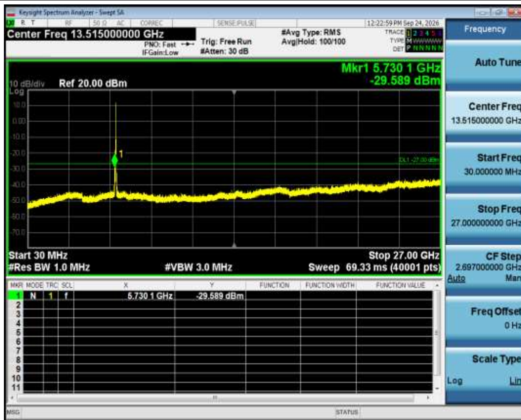
Tx. Spurious NVNT ac20 5785MHz Ant1 Emission
