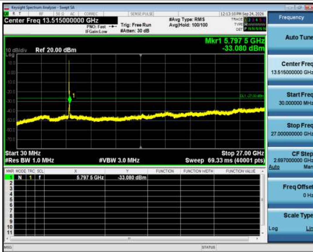
Tx. Spurious NVNT n20 5745MHz Ant1 Emission
