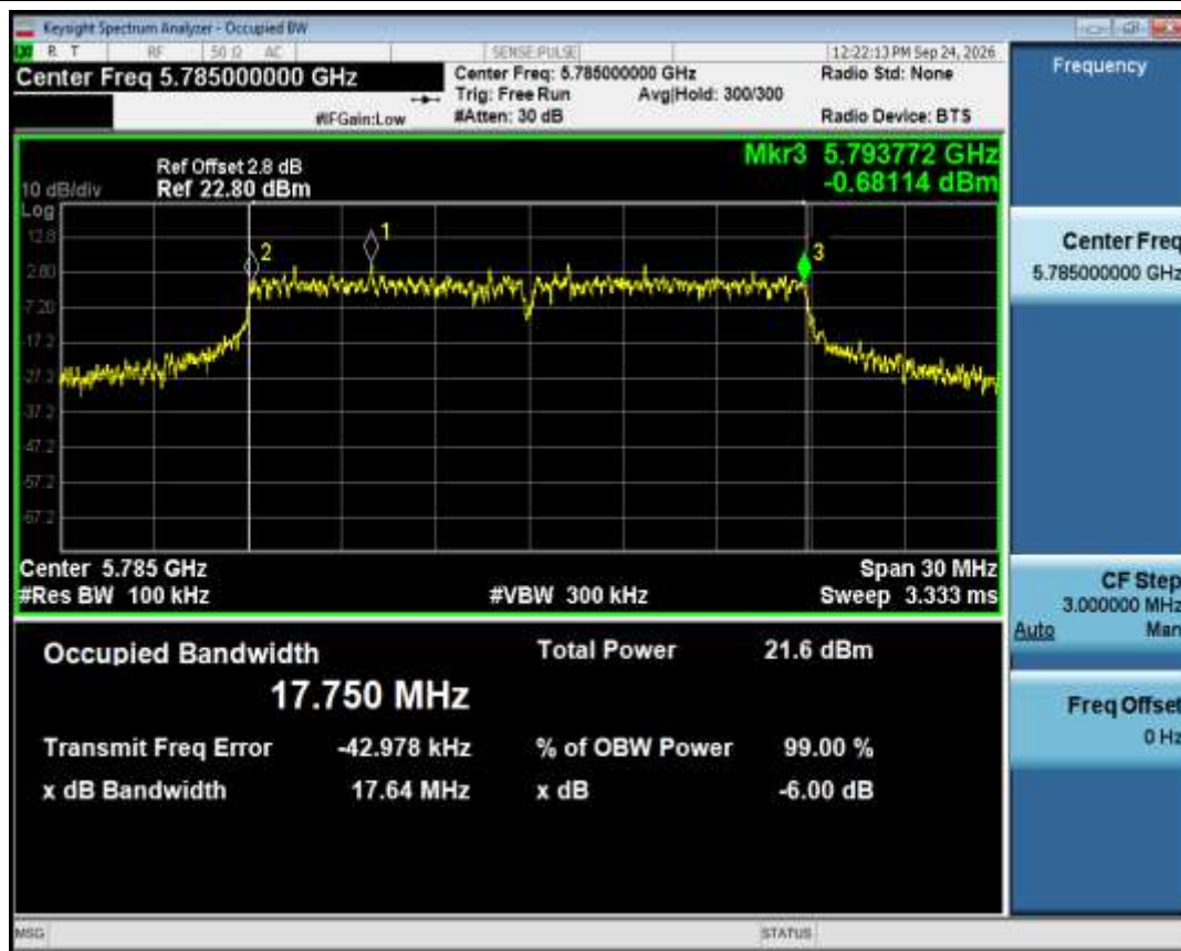
-6dB Bandwidth NVNT ac20 5785MHz Ant1
