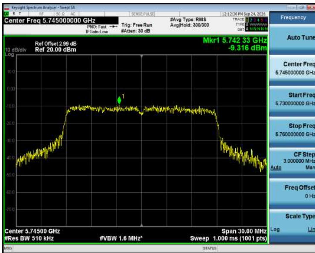
PSD NVNT n20 5745MHz Ant1
