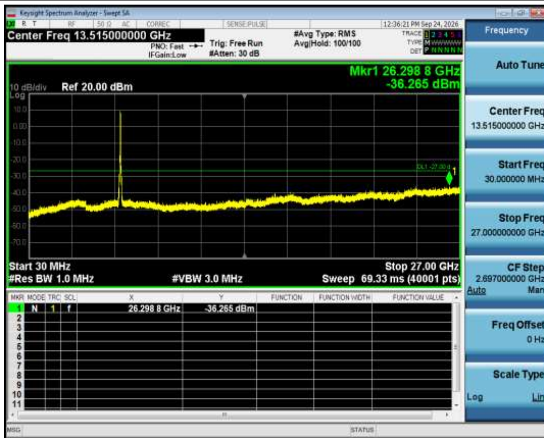
Tx. Spurious NVNT ac40 5755MHz Ant1 Emission
