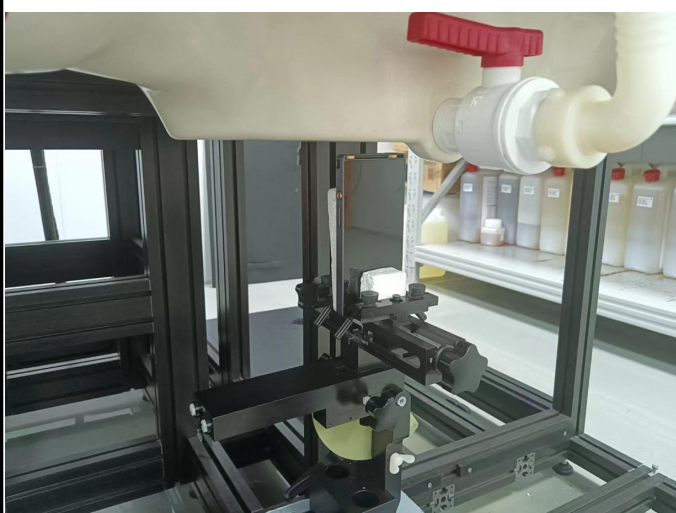
Top Side of EUT with 1.0 cm Gap
