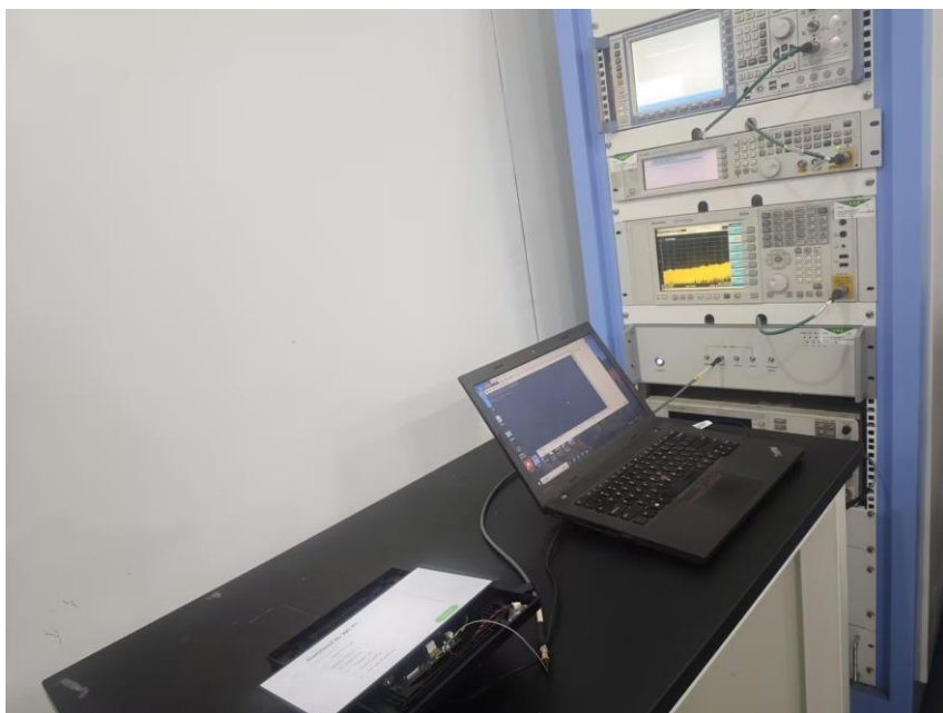
Conducted Test for WiFi
