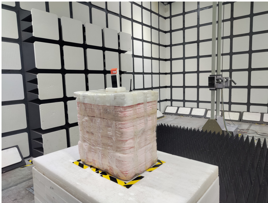
Radiated Emissions View (1-18 GHz)-TX
