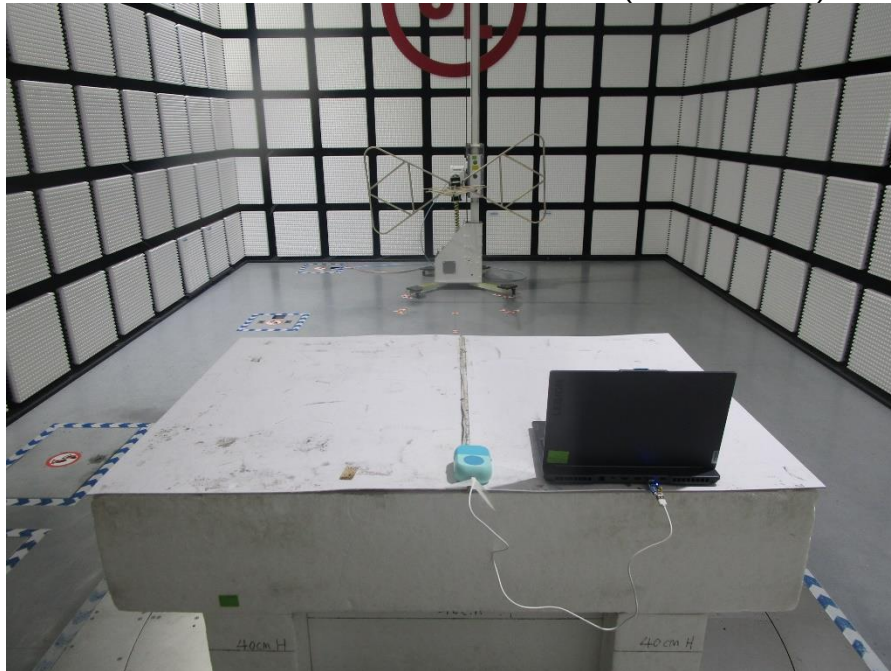
RADIATED RF MEASUREMENT SETUP (Below 30MHz)
