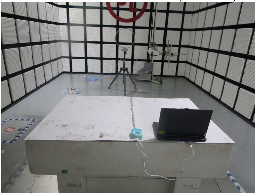
RADIATED RF MEASUREMENT SETUP (Below 30MHz)
