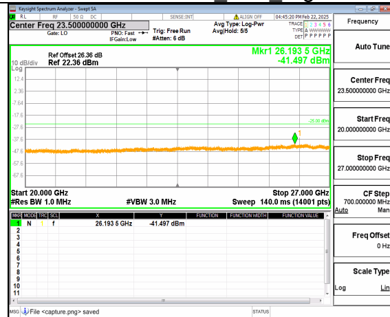
66A_n41 (20GHz-27GHz) 90M DFT-s-OFDM QPSK Outer_Full High
