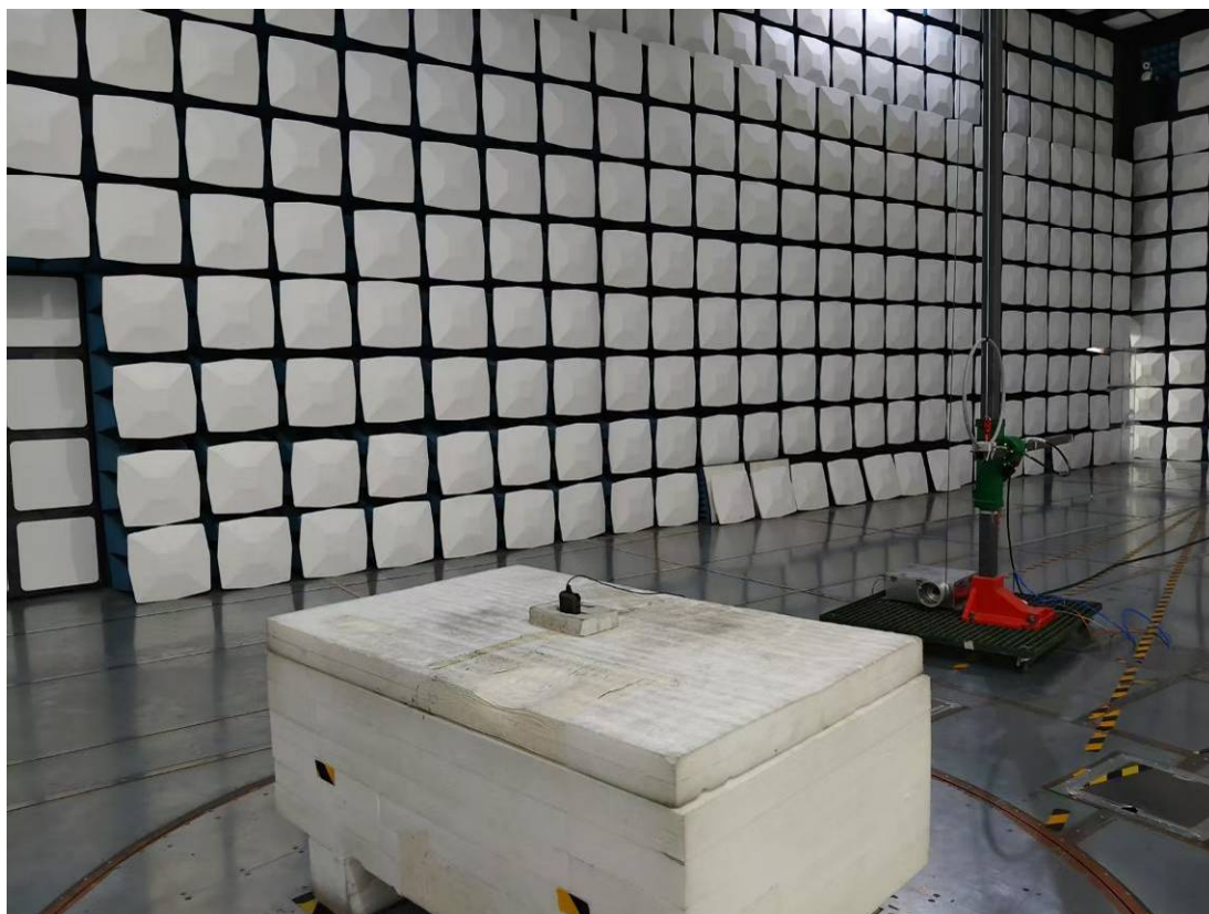
Radiated Emission 9k-30MHz Perpendicular View
