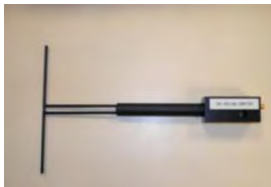
Figure 1 – MVG COMOSAR Validation Dipole
