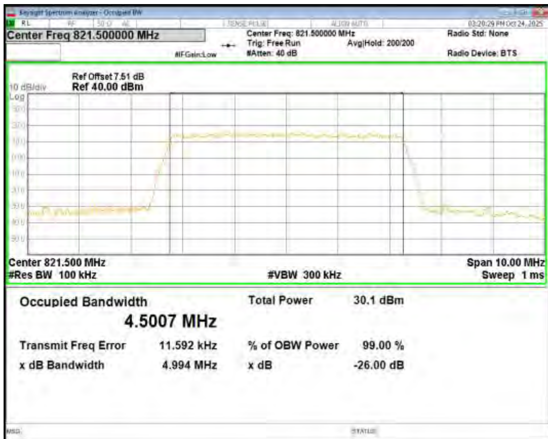
Band26(824-849) 16QAM BW=1.4MHz Channel=26797 RB Size=6 Position=#0
