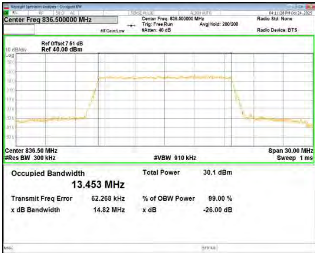
Band26(824-849) QPSK BW=15MHz Channel=26965 RB Size=75 Position=#0
