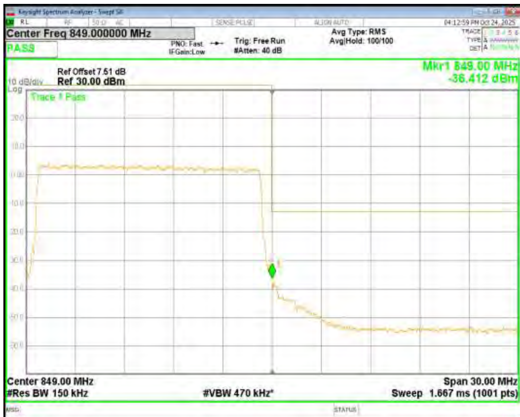
Band26(824-849) QPSK BW=3MHz Channel=26805 RB Size=15 Position=#0
