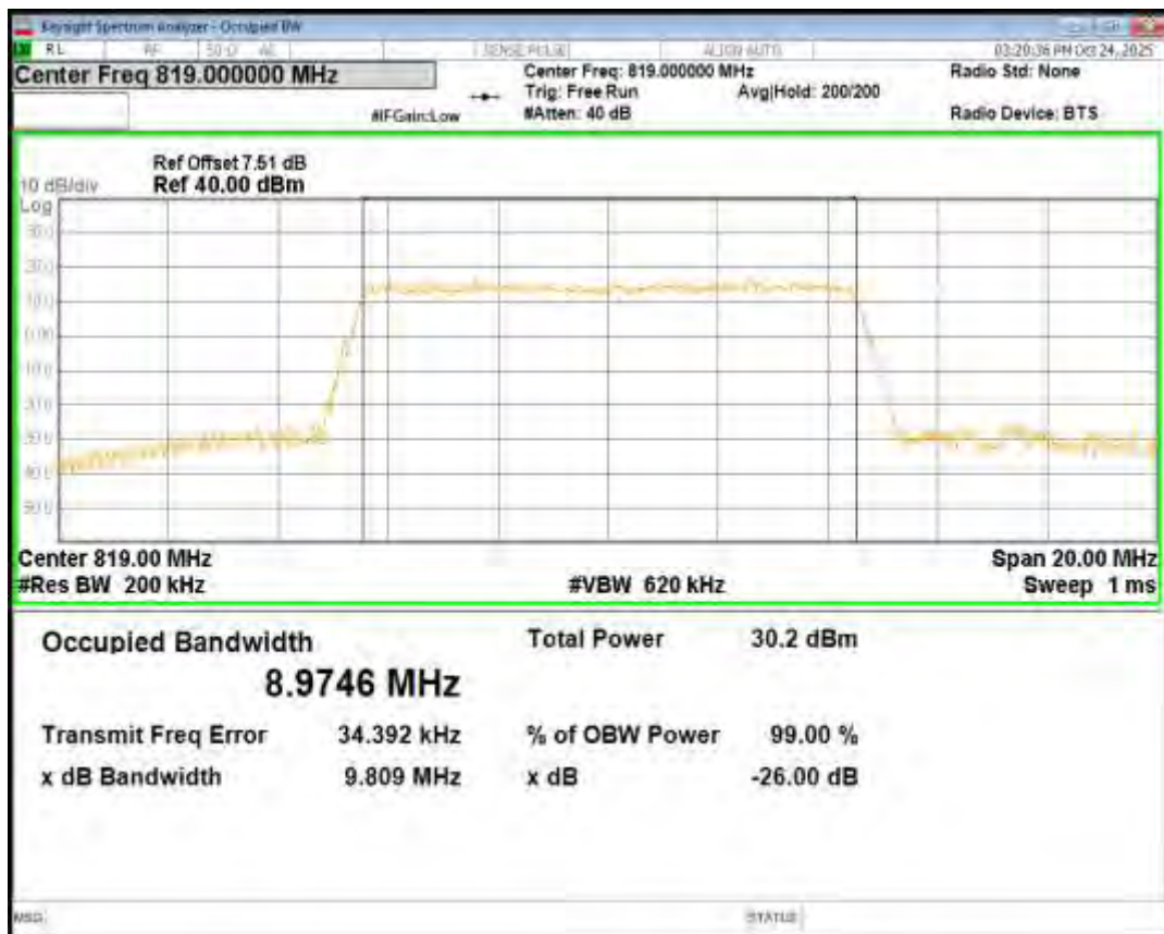
Band26(814-824) QPSK BW=3MHz Channel=26705 RB Size=15 Position=#0
