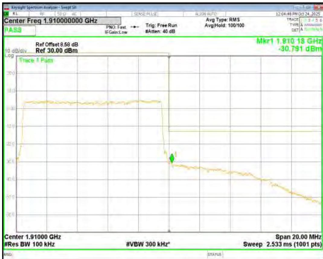
Band2 QPSK BW=15MHz Channel=18675 RB Size=75 Position=#0
