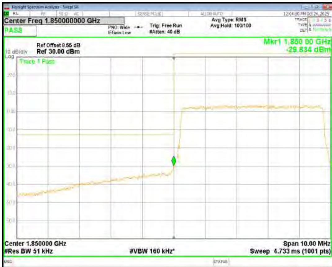
Band2 QPSK BW=1.4MHz Channel=19193 RB Size=6 Position=#0
