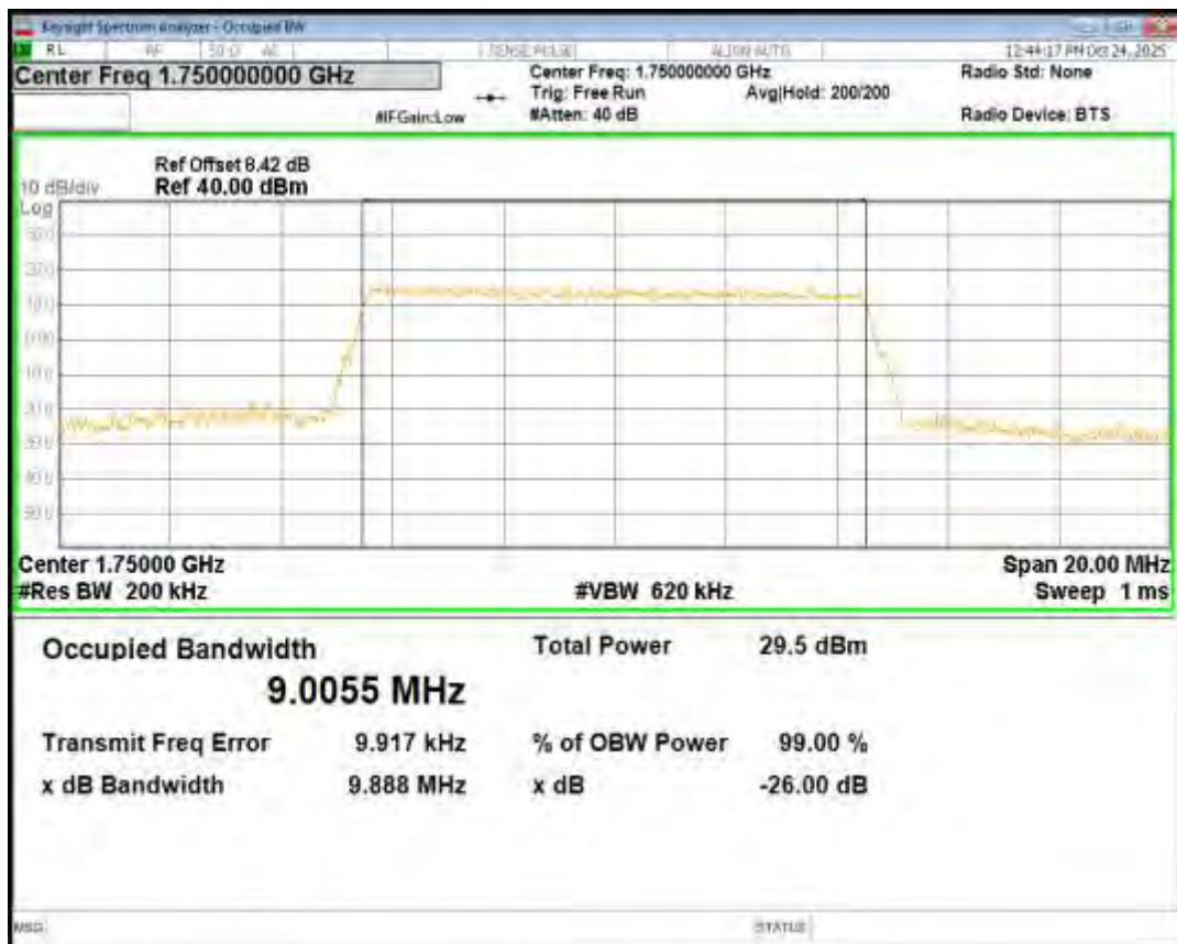
Band4 16QAM BW=15MHz Channel=20025 RB Size=75 Position=#0
