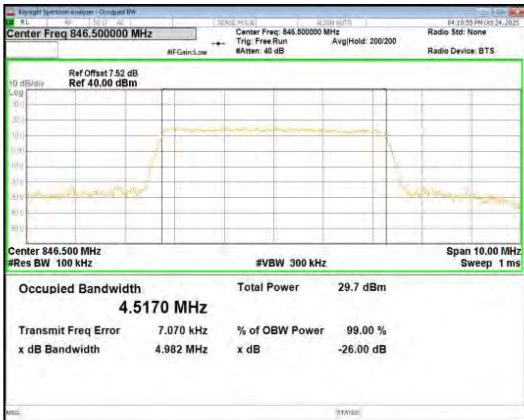
Band26(824-849) QPSK BW=1.4MHz Channel=26797 RB Size=6 Position=#0
