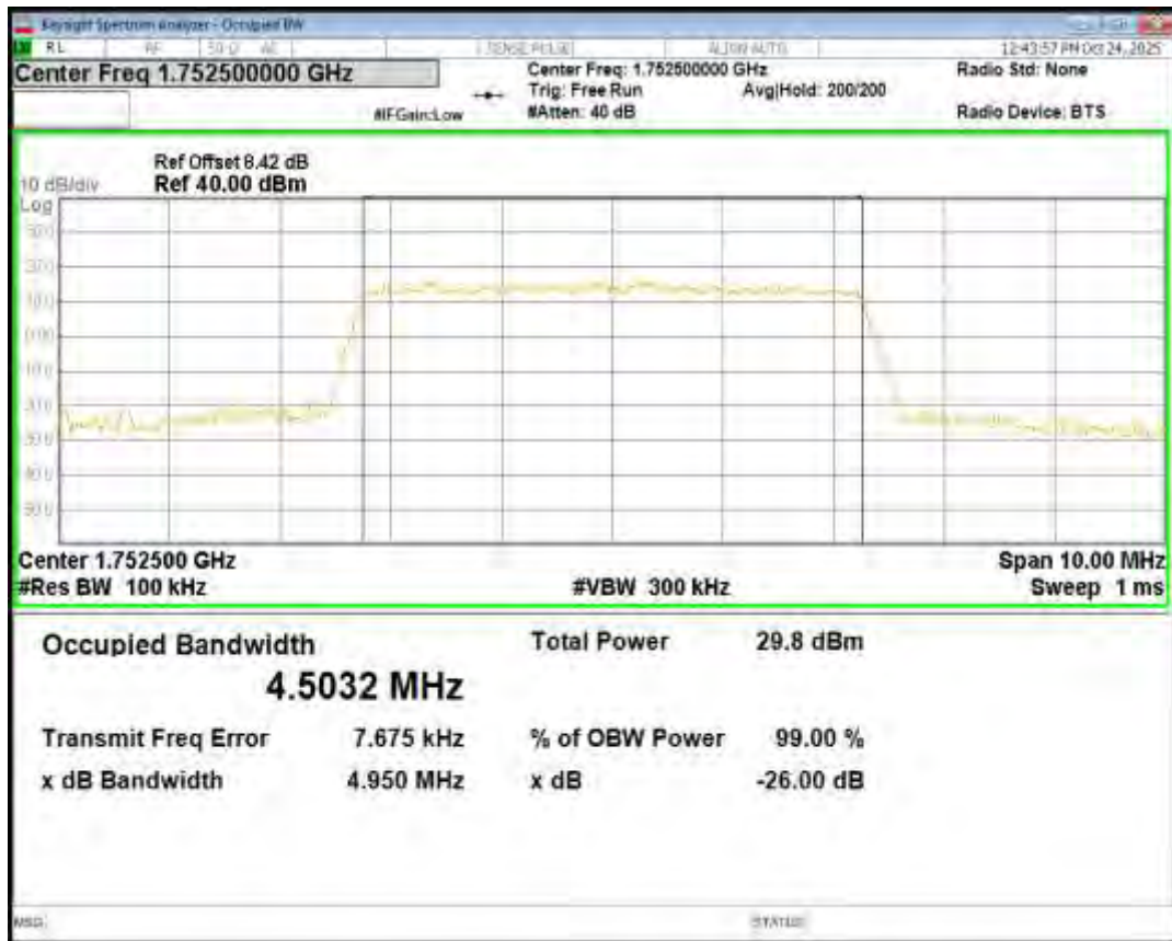
Band4 16QAM BW=5MHz Channel=19975 RB Size=25 Position=#0
