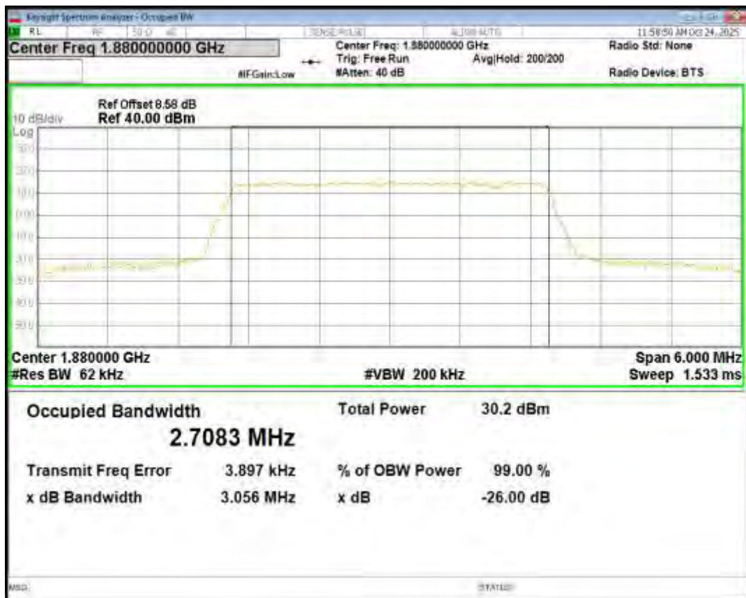
Band2 16QAM BW=3MHz Channel=19185 RB Size=15 Position=#0
