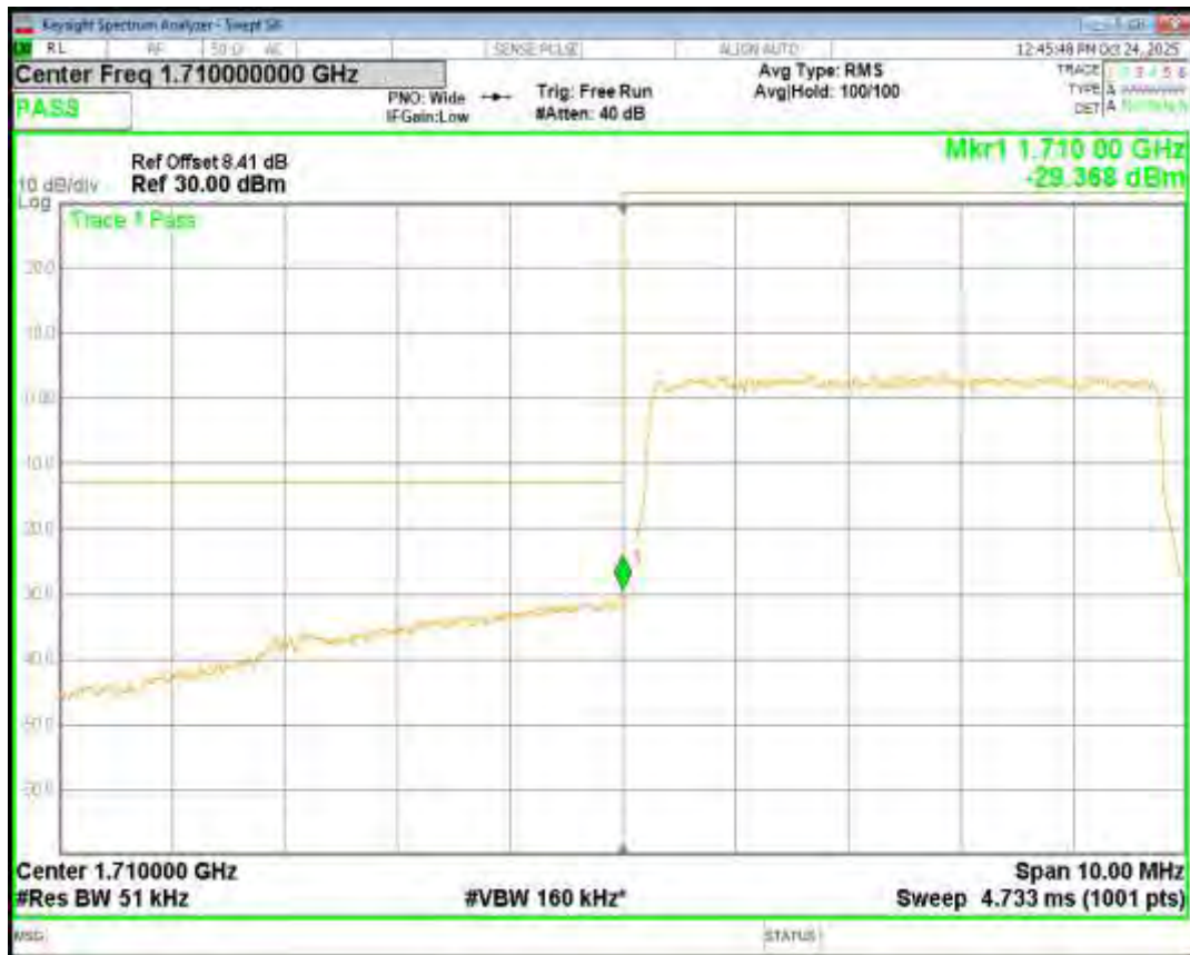
Band4 QPSK BW=1.4MHz Channel=20393 RB Size=6 Position=#0
