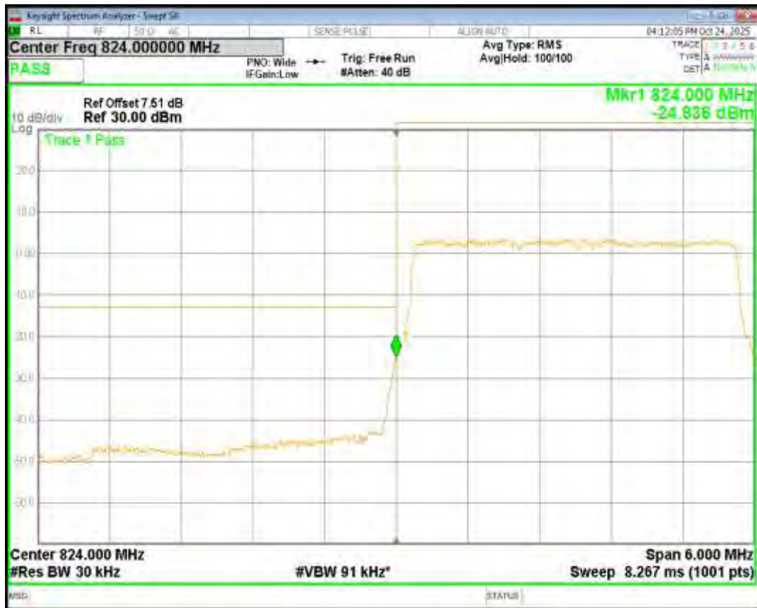
Band26(824-849) QPSK BW=3MHz Channel=27025 RB Size=15 Position=#0
