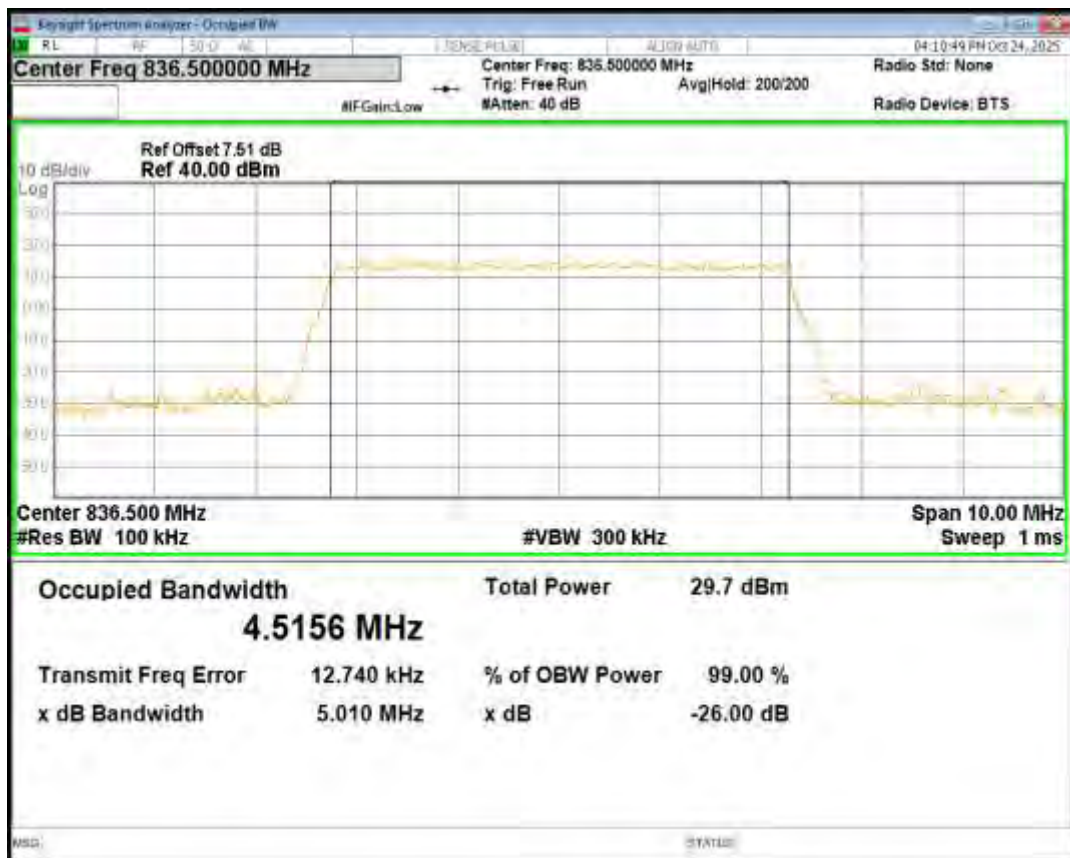
Band26(824-849) QPSK BW=1.4MHz Channel=26915 RB Size=6 Position=#0
