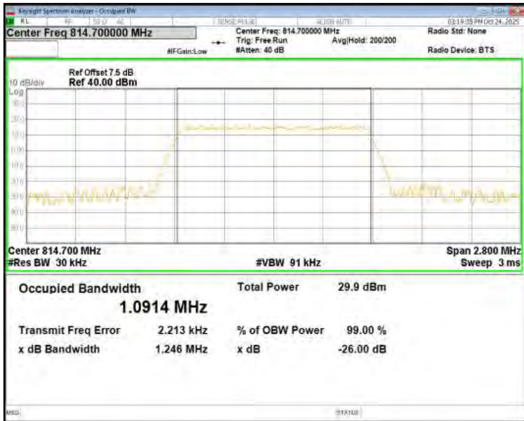
Band26(814-824) QPSK BW=10MHz Channel=26740 RB Size=50 Position=#0
