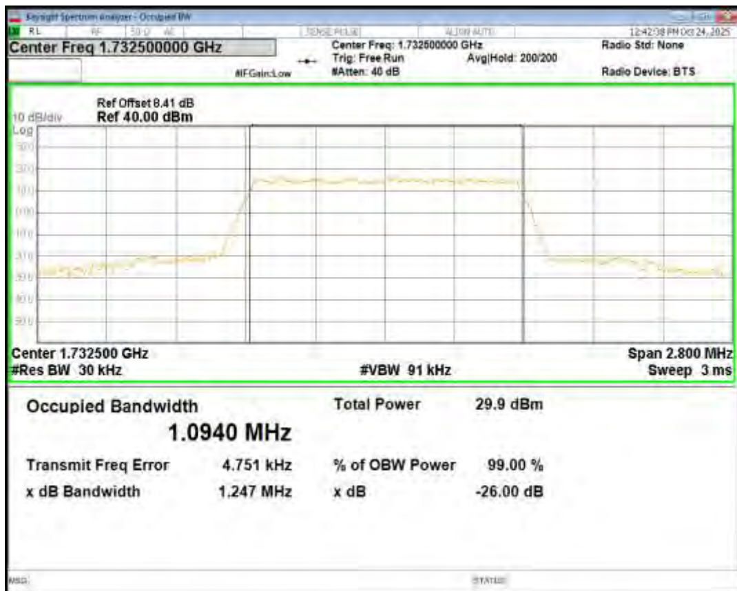
Band4 QPSK BW=1.4MHz Channel=20393 RB Size=6 Position=#0
