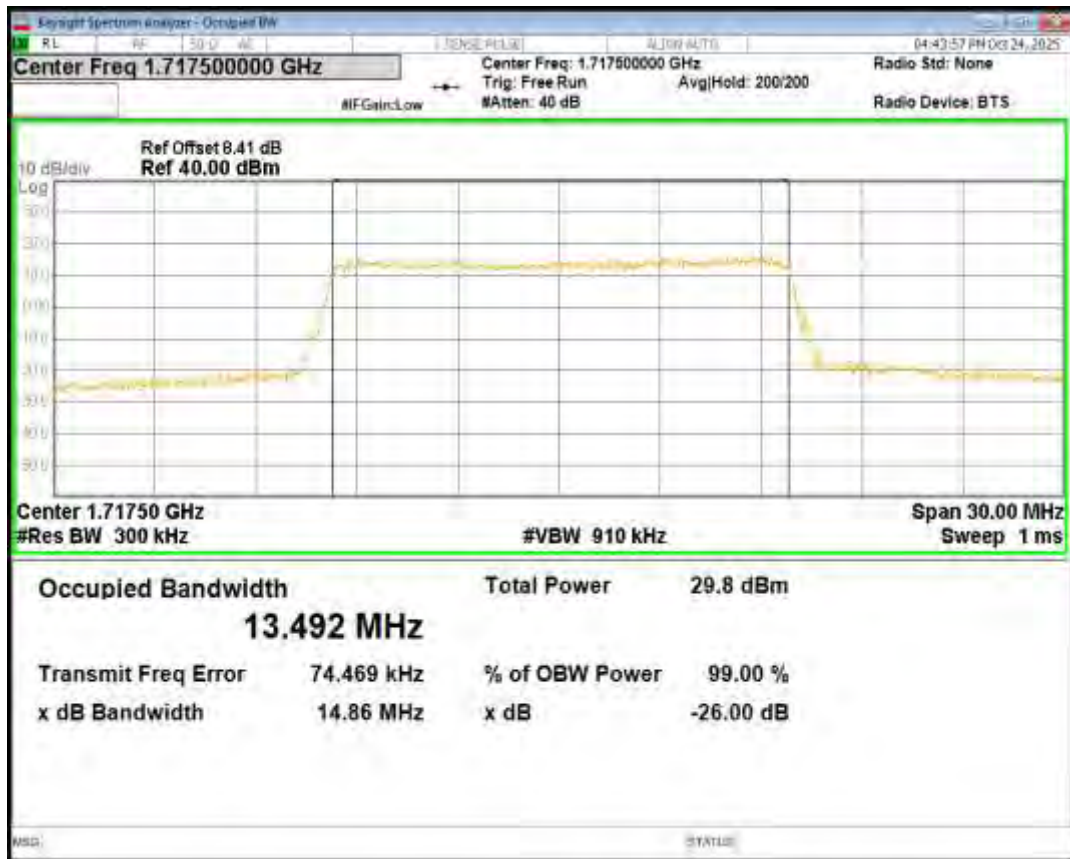
Band66 QPSK BW=15MHz Channel=132322 RB Size=75 Position=#0
