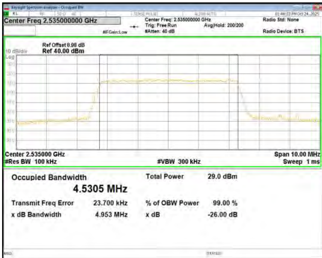
Band7 16QAM BW=5MHz Channel=21425 RB Size=25 Position=#0
