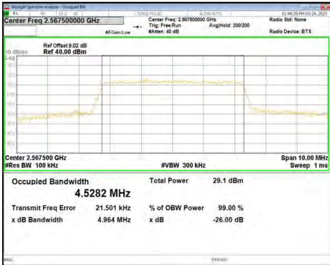
Band7 16QAM BW=5MHz Channel=20775 RB Size=25 Position=#0
