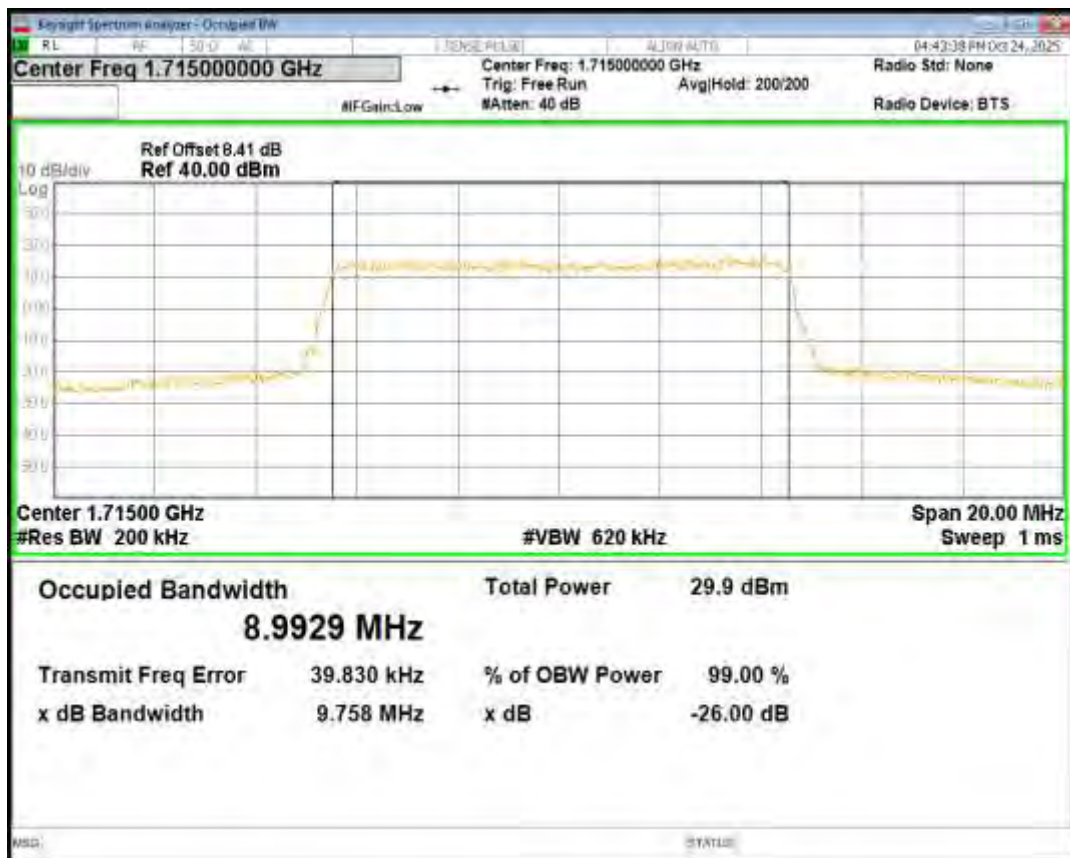
Band66 QPSK BW=10MHz Channel=132322 RB Size=50 Position=#0
