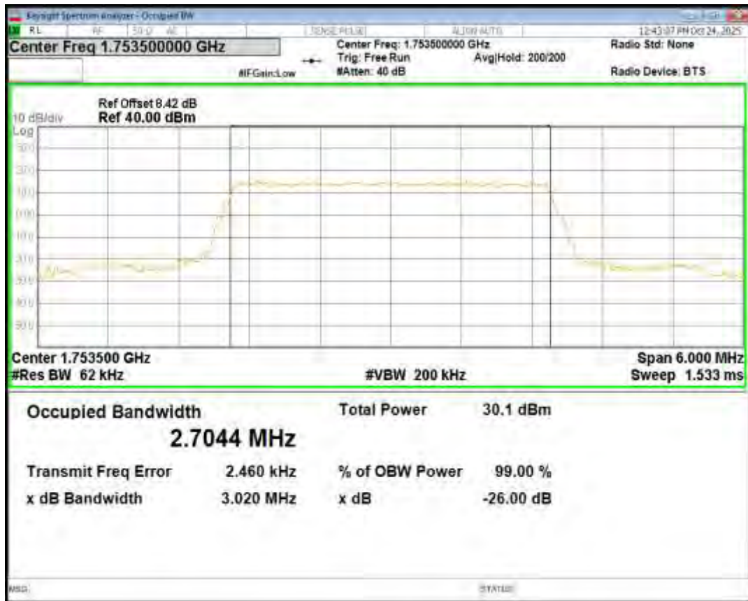
Band4 16QAM BW=5MHz Channel=20175 RB Size=25 Position=#0
