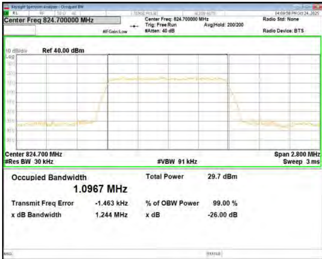
Band26(824-849) QPSK BW=1.4MHz Channel=27033 RB Size=6 Position=#0
