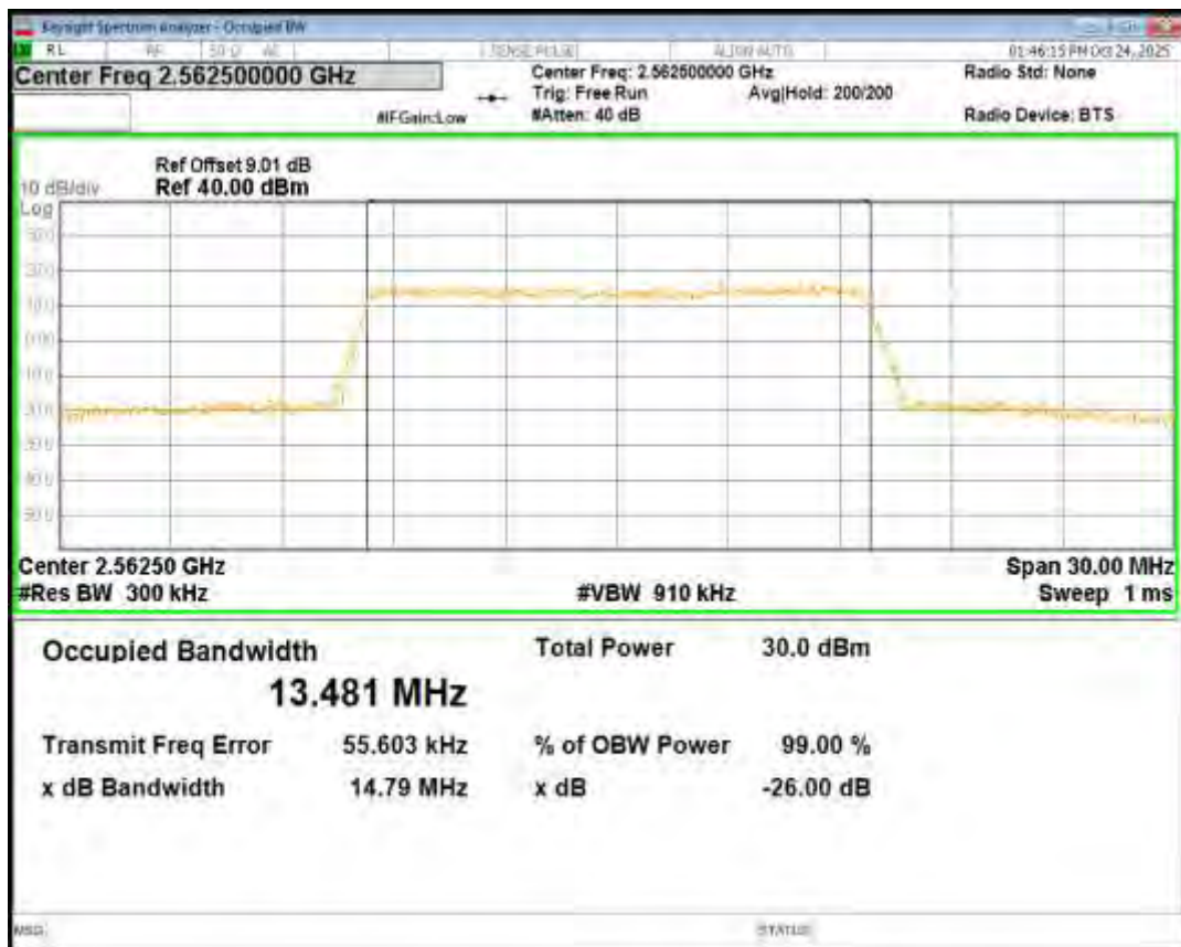
Band7 QPSK BW=20MHz Channel=20850 RB Size=100 Position=#0
