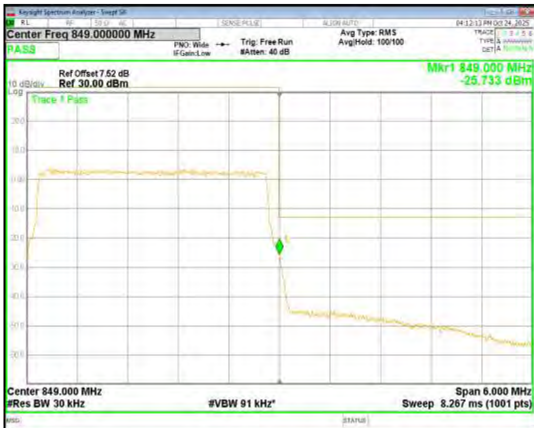
Band26(824-849) QPSK BW=5MHz Channel=26815 RB Size=25 Position=#0
