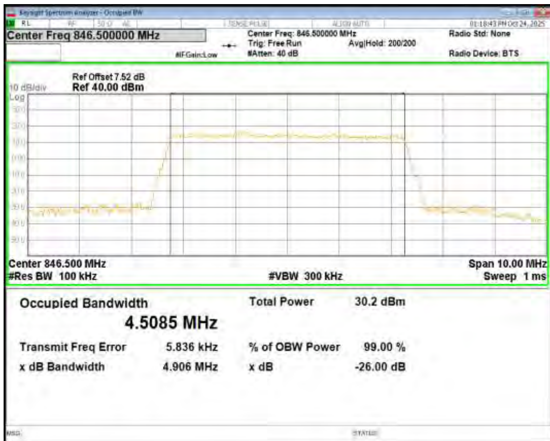
Band66 16QAM BW=1.4MHz Channel=131979 RB Size=6 Position=#0
