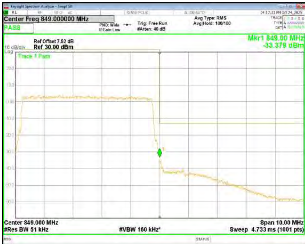
Band26(824-849) 16QAM BW=3MHz Channel=27025 RB Size=15 Position=#0
