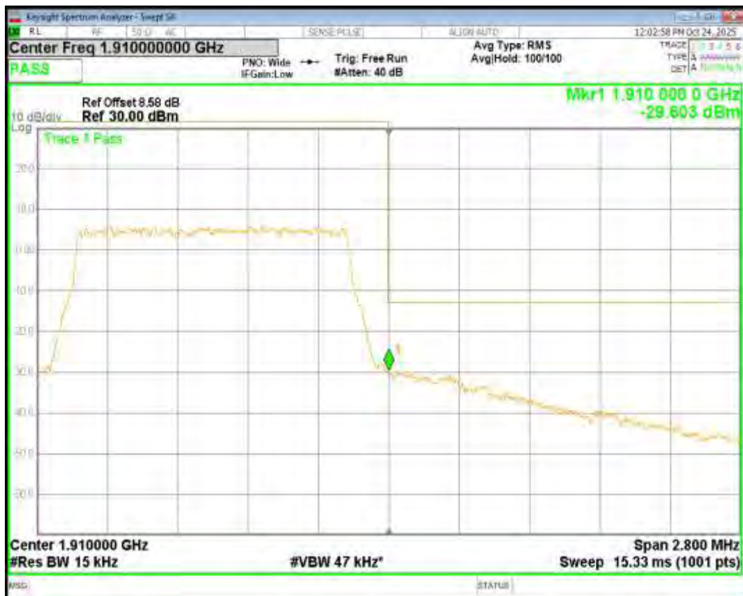
Band2 QPSK BW=10MHz Channel=18650 RB Size=50 Position=#0
