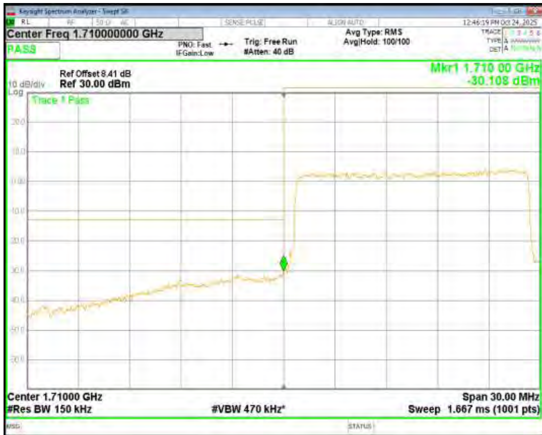
Band4 16QAM BW=15MHz Channel=20325 RB Size=75 Position=#0
