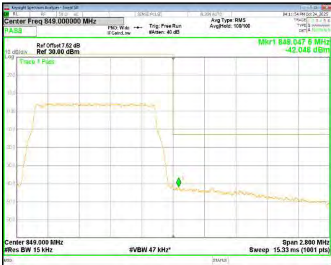
Band26(824-849) QPSK BW=10MHz Channel=26840 RB Size=50 Position=#0
