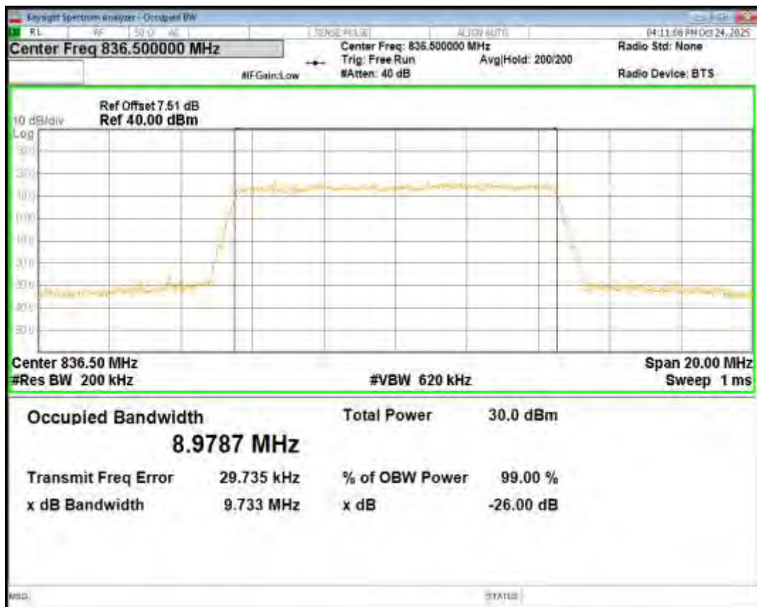
Band26(824-849) QPSK BW=10MHz Channel=26990 RB Size=50 Position=#0
