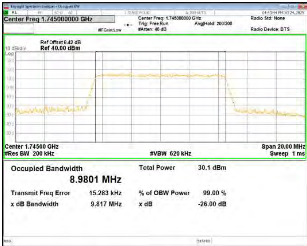
Band66 QPSK BW=10MHz Channel=132622 RB Size=50 Position=#0
