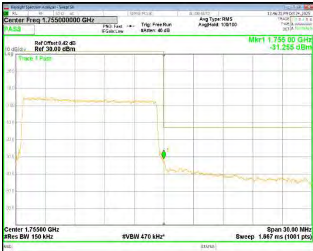
Band4 QPSK BW=20MHz Channel=20050 RB Size=100 Position=#0
