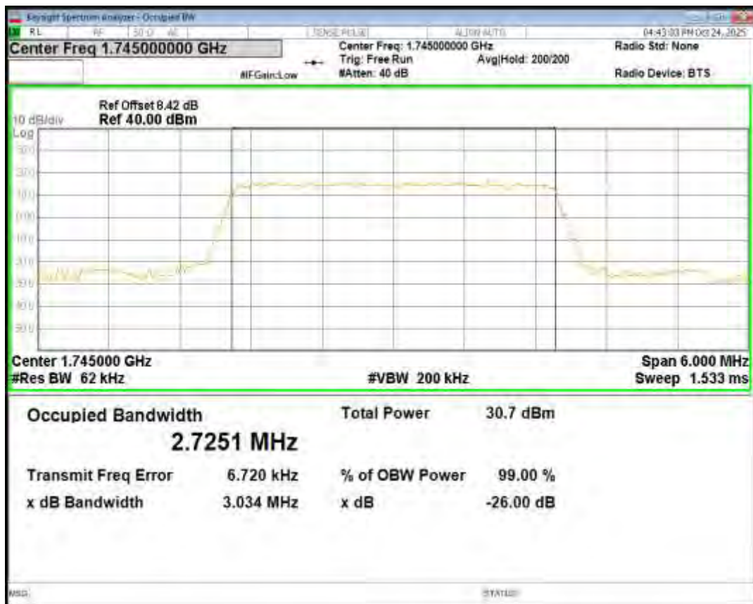
Band66 QPSK BW=3MHz Channel=132657 RB Size=15 Position=#0
