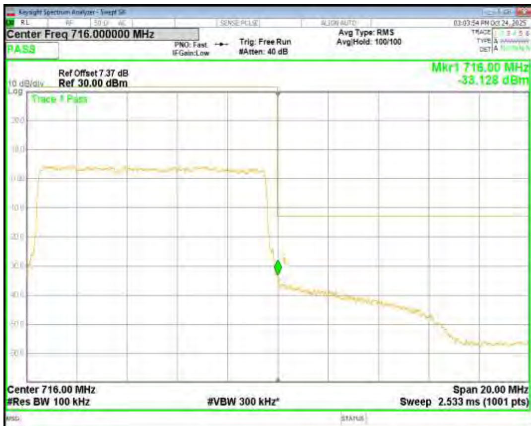
Band17 QPSK BW=5MHz Channel=23755 RB Size=25 Position=#0
