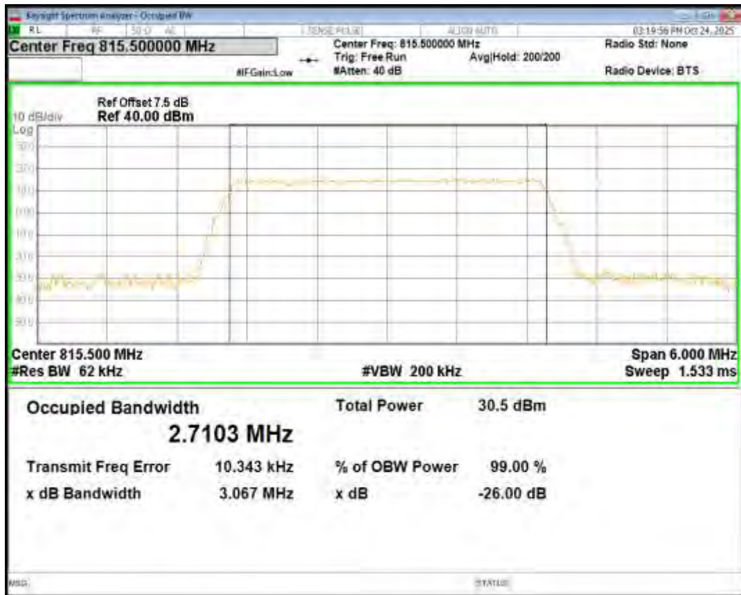
Band26(814-824) QPSK BW=3MHz Channel=26740 RB Size=15 Position=#0
