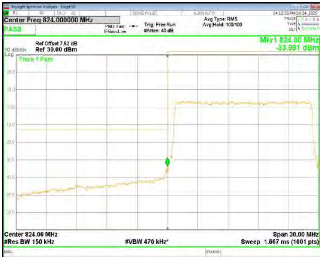
Band26(824-849) 16QAM BW=15MHz Channel=26965 RB Size=75 Position=#0
