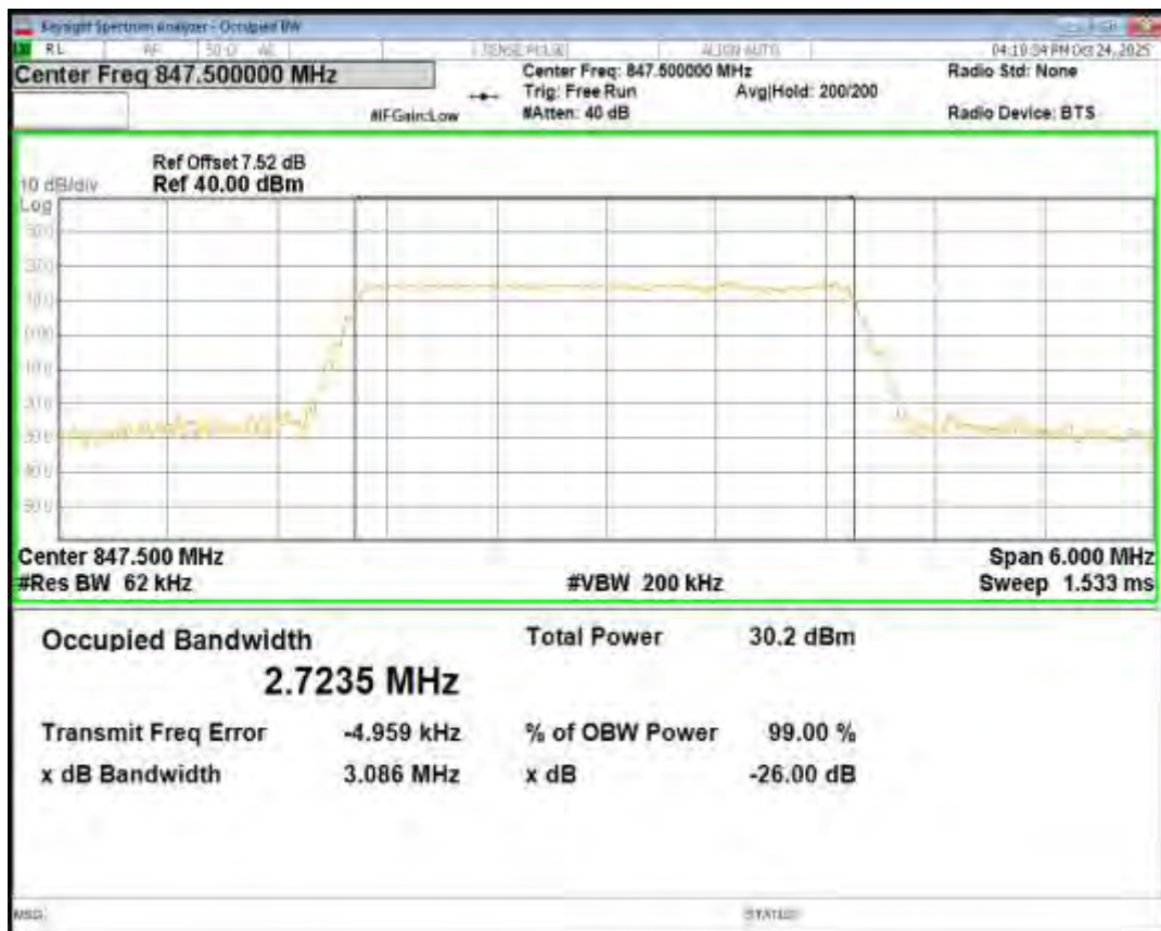
Band26(824-849) 16QAM BW=5MHz Channel=26815 RB Size=25 Position=#0
