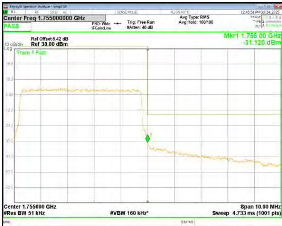
Band5 16QAM BW=1.4MHz Channel=20407 RB Size=6 Position=#0
