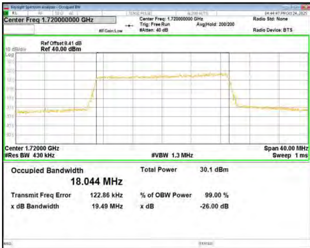
Band66 QPSK BW=20MHz Channel=132322 RB Size=100 Position=#0
