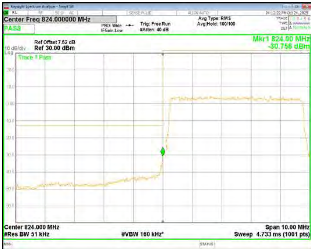
Band26(824-849) QPSK BW=5MHz Channel=27015 RB Size=25 Position=#0
