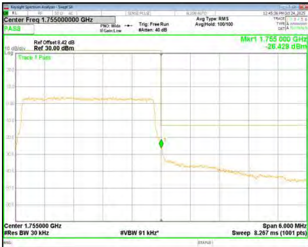
Band4 QPSK BW=5MHz Channel=19975 RB Size=25 Position=#0
