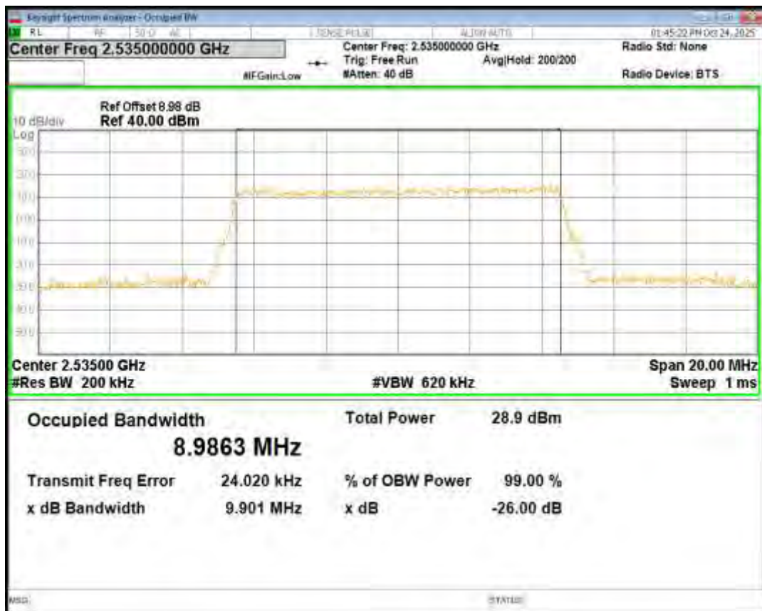
Band7 16QAM BW=10MHz Channel=21400 RB Size=50 Position=#0
