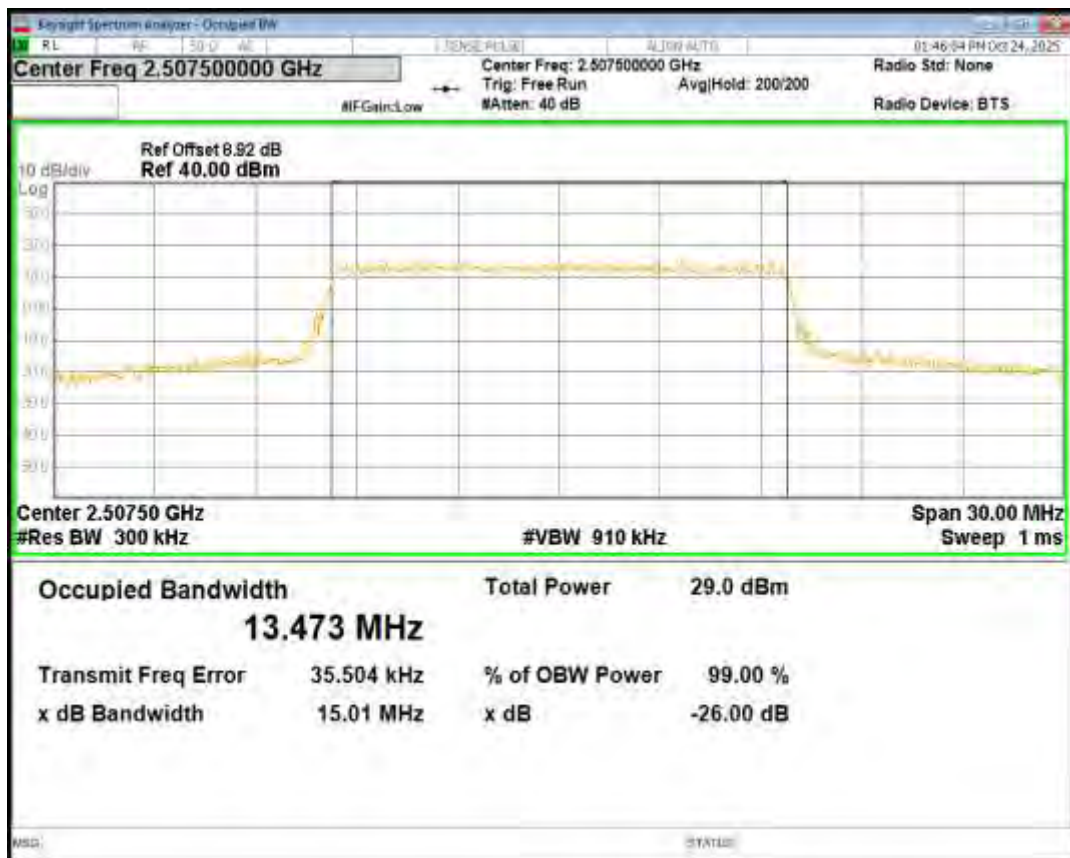
Band7 16QAM BW=15MHz Channel=21100 RB Size=75 Position=#0
