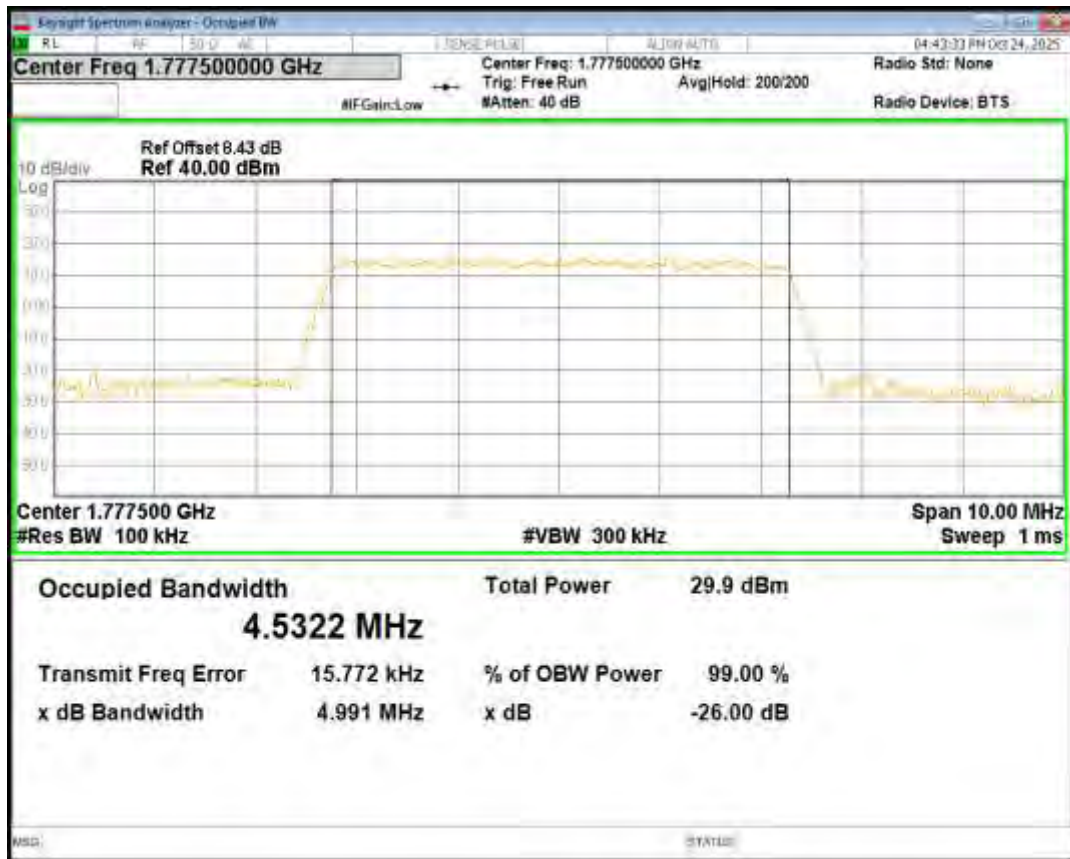
Band66 16QAM BW=5MHz Channel=131997 RB Size=25 Position=#0
