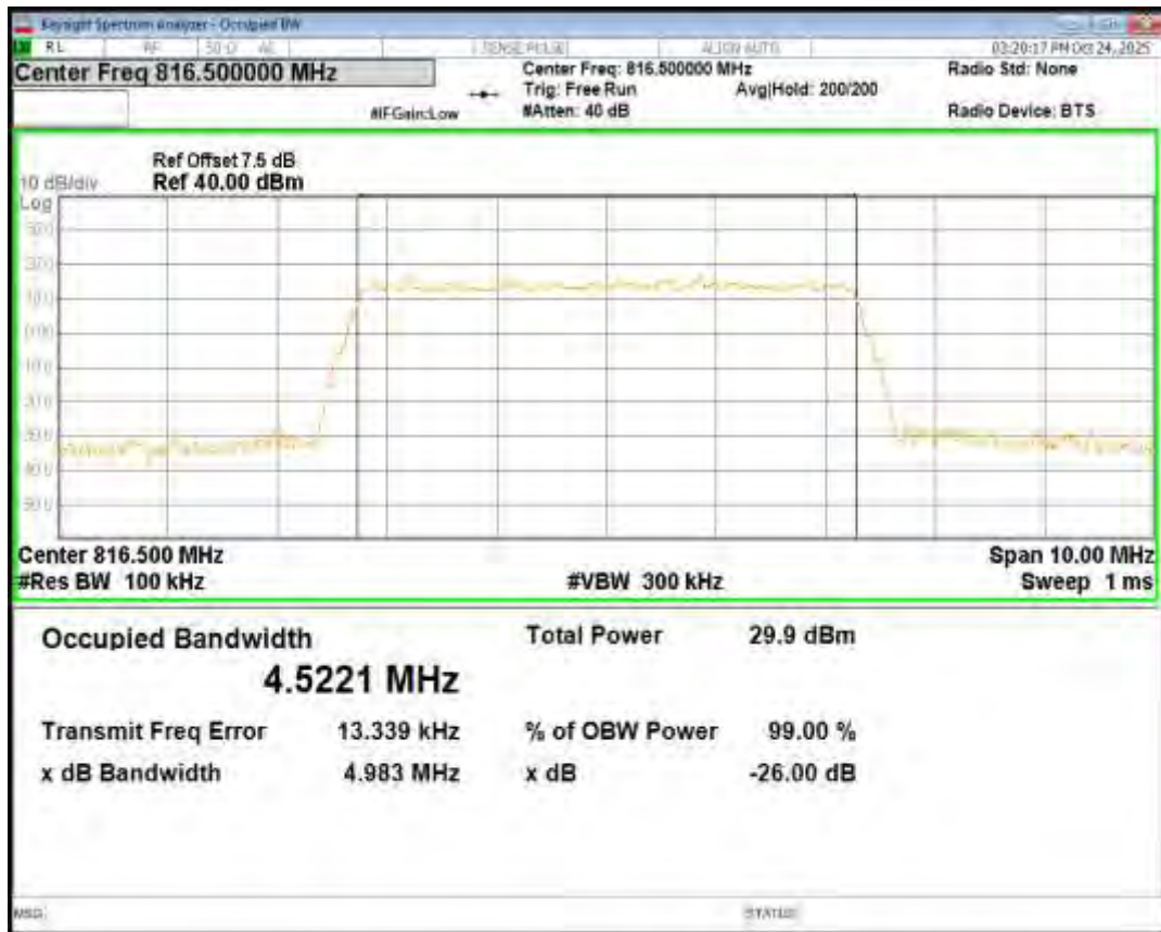
Band26(814-824) QPSK BW=5MHz Channel=26765 RB Size=25 Position=#0
