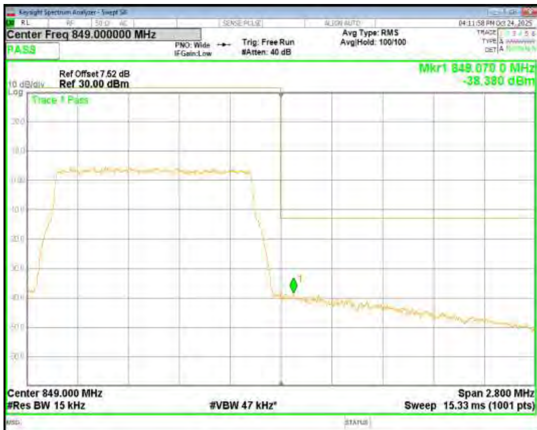
Band26(824-849) 16QAM BW=10MHz Channel=26840 RB Size=50 Position=#0
