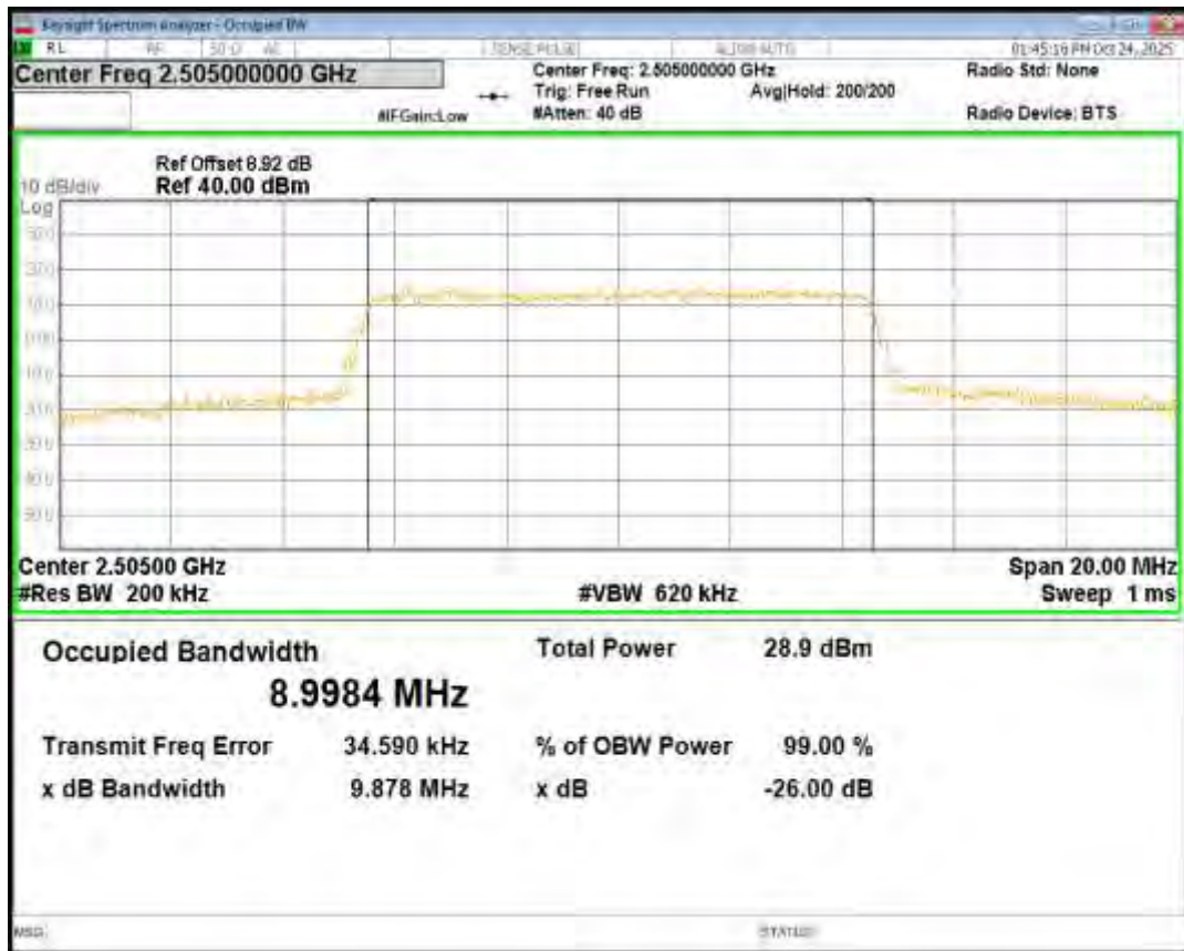
Band7 16QAM BW=10MHz Channel=21100 RB Size=50 Position=#0
