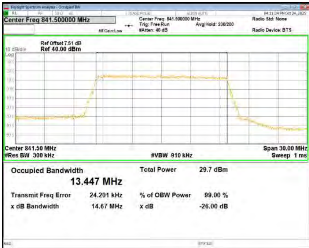
Band26(824-849) QPSK BW=3MHz Channel=26805 RB Size=15 Position=#0
