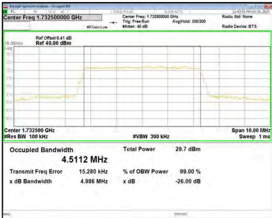
Band4 16QAM BW=5MHz Channel=20375 RB Size=25 Position=#0
