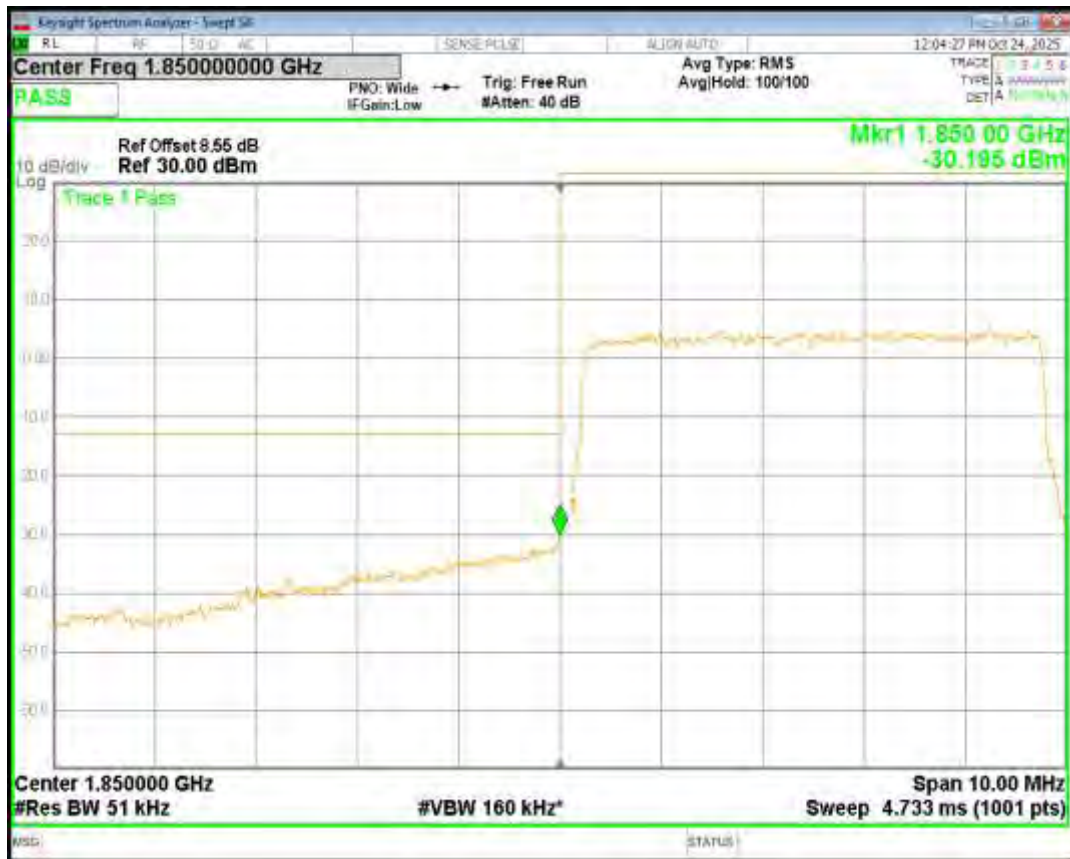
Band2 QPSK BW=5MHz Channel=19175 RB Size=25 Position=#0
