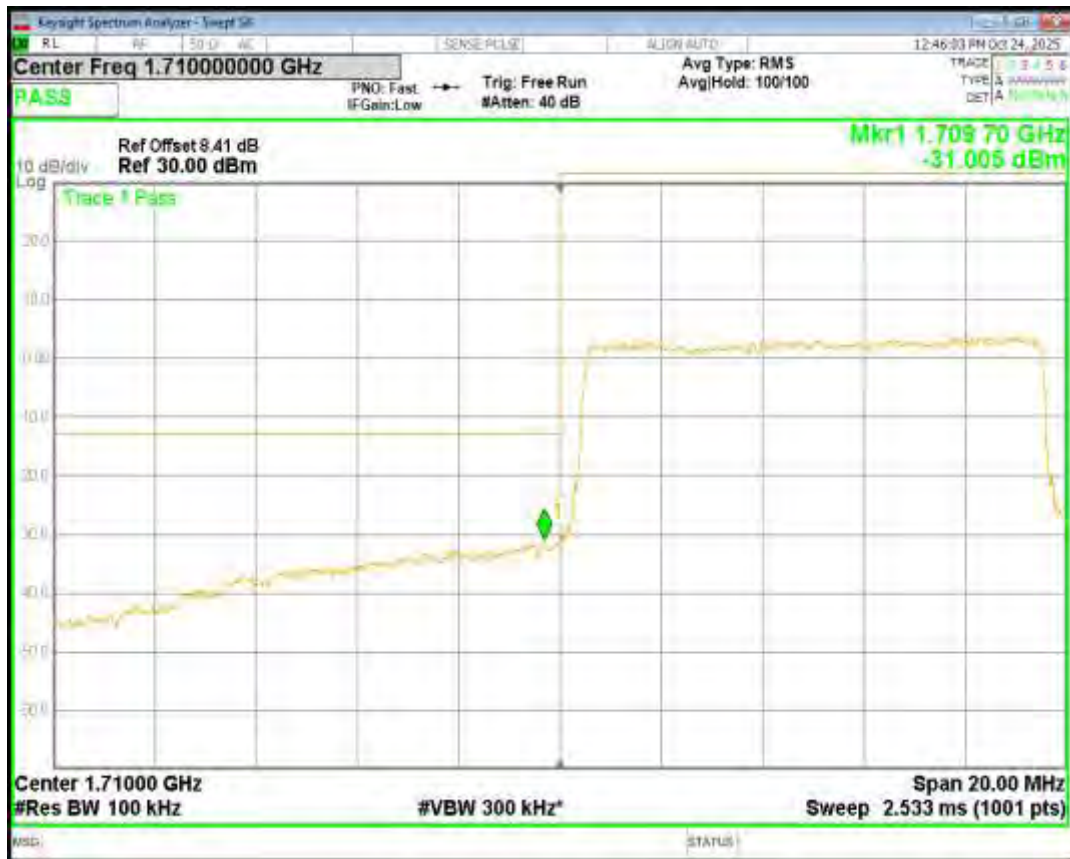
Band4 16QAM BW=10MHz Channel=20350 RB Size=50 Position=#0
