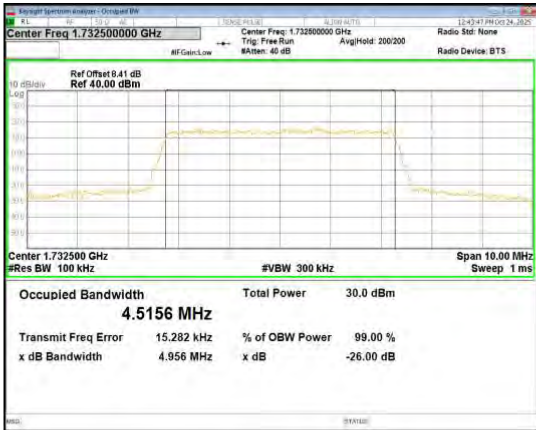
Band4 QPSK BW=5MHz Channel=20375 RB Size=25 Position=#0
