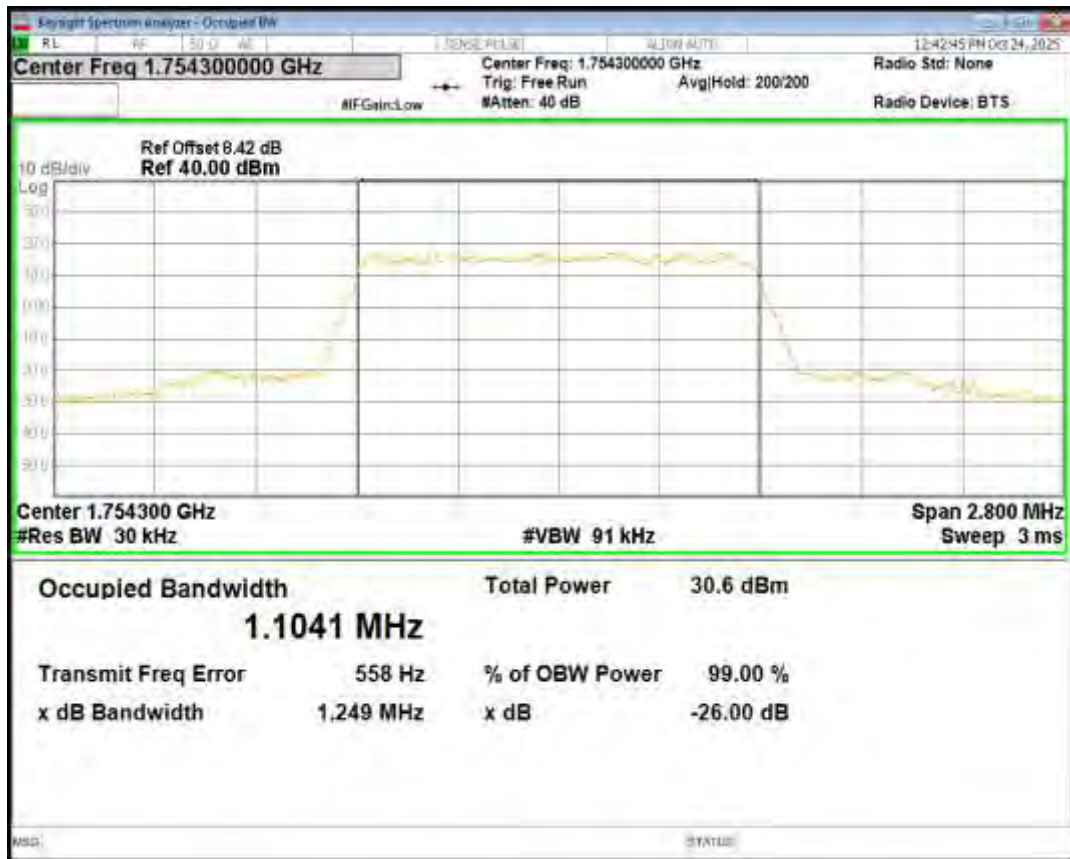
Band4 QPSK BW=10MHz Channel=20000 RB Size=50 Position=#0
