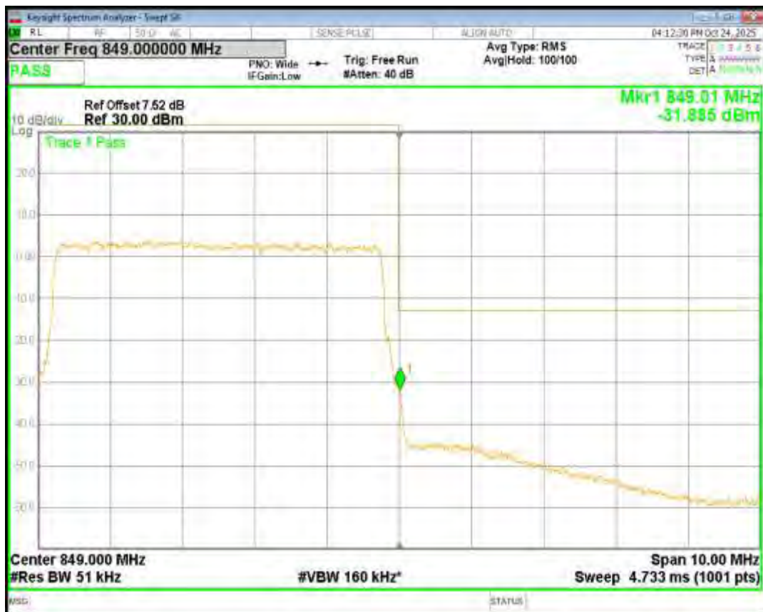
Band4 16QAM BW=1.4MHz Channel=19957 RB Size=6 Position=#0
