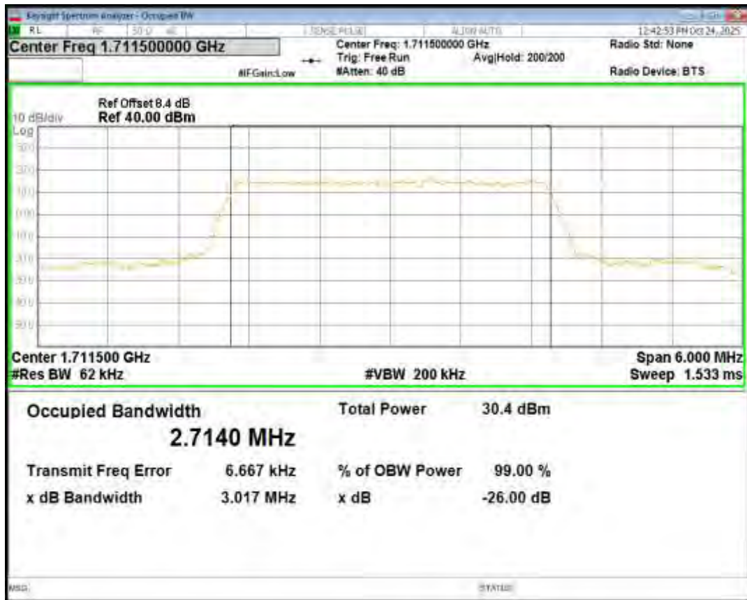
Band4 QPSK BW=20MHz Channel=20300 RB Size=100 Position=#0
