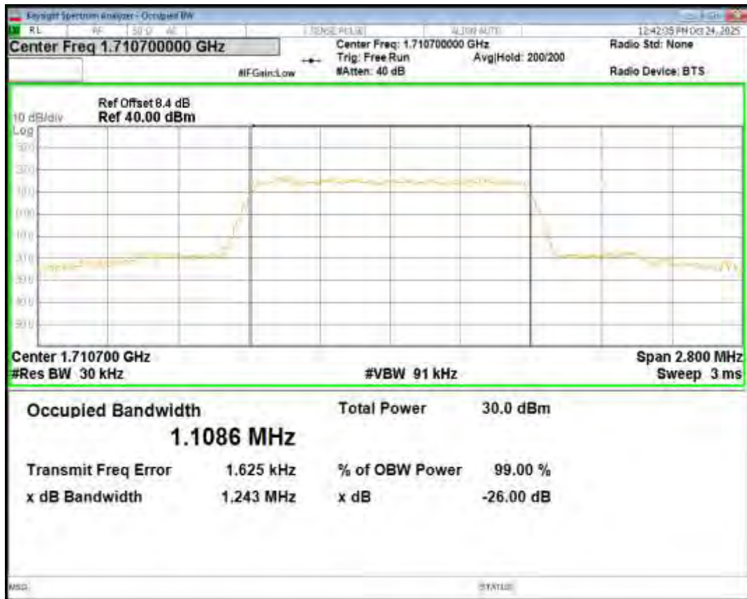
Band4 16QAM BW=1.4MHz Channel=20175 RB Size=6 Position=#0
