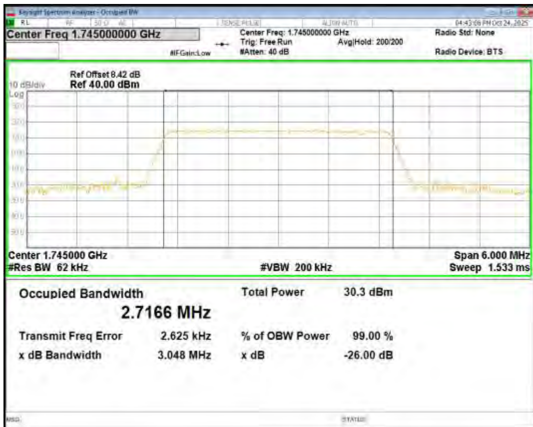
Band66 16QAM BW=3MHz Channel=132657 RB Size=15 Position=#0
