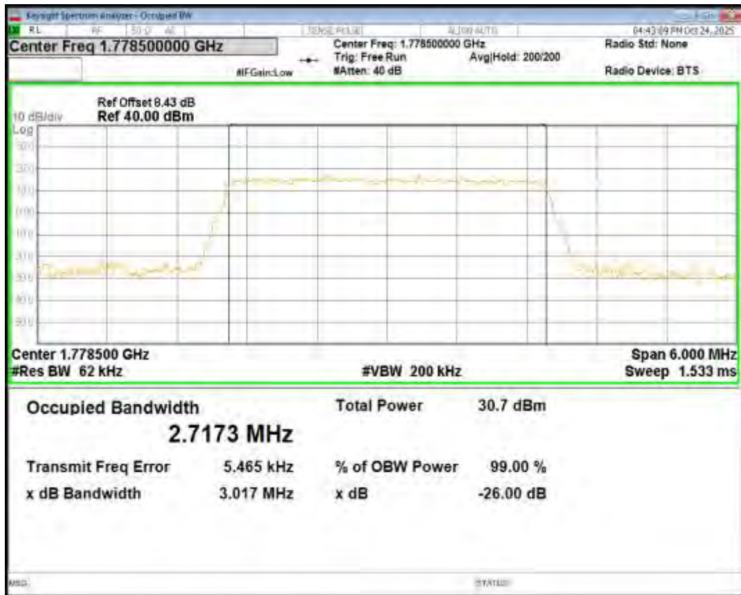
Band66 QPSK BW=5MHz Channel=132647 RB Size=25 Position=#0
