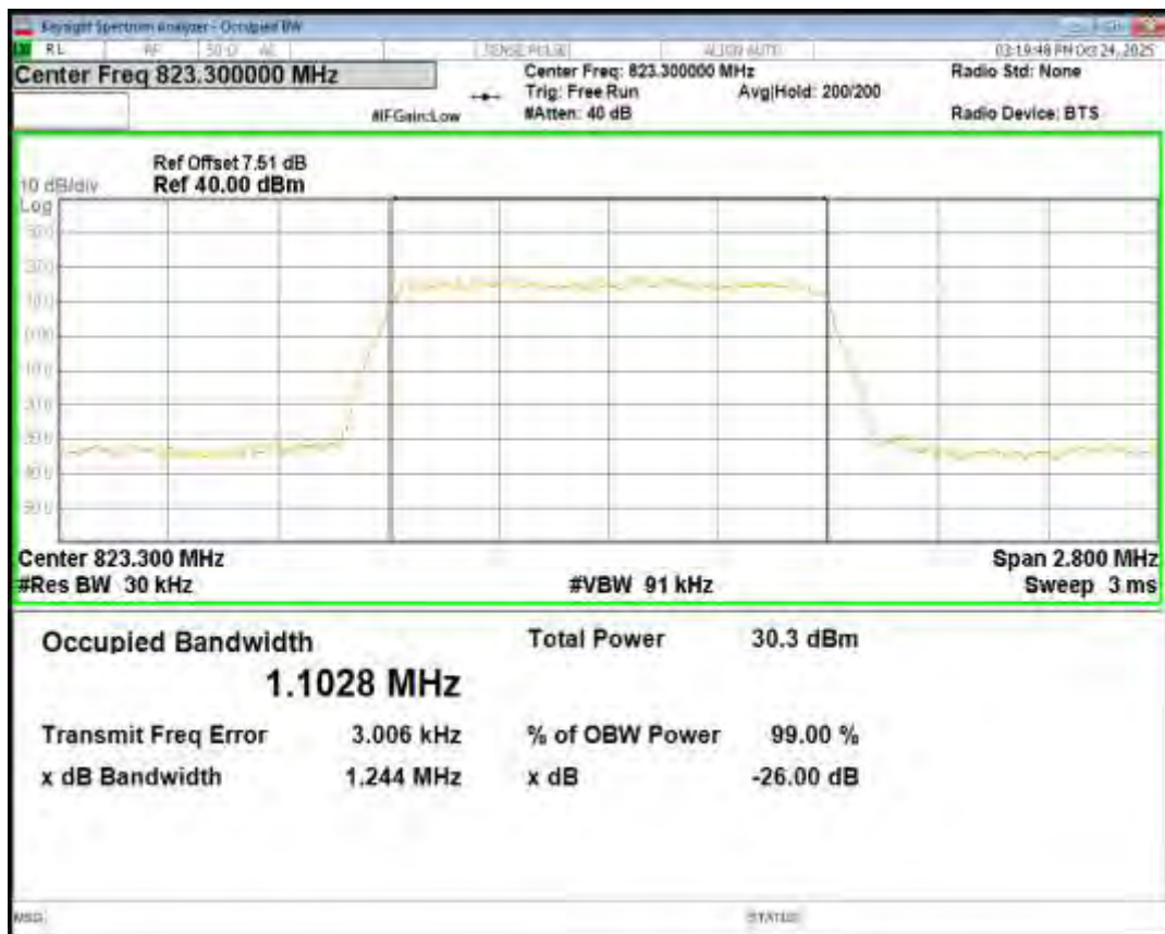
Band26(814-824) QPSK BW=1.4MHz Channel=26740 RB Size=6 Position=#0
