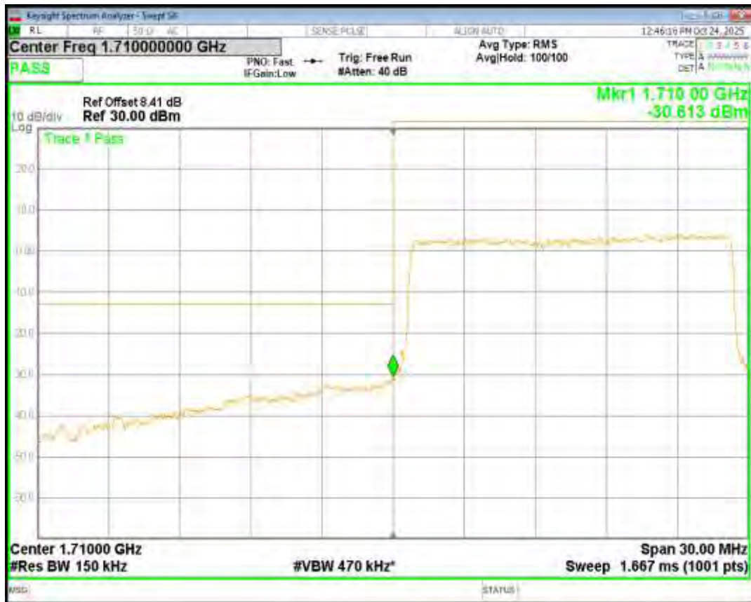
Band4 QPSK BW=15MHz Channel=20325 RB Size=75 Position=#0
