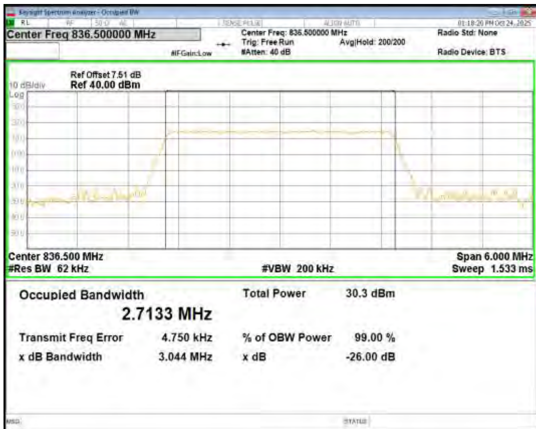
Band5 16QAM BW=3MHz Channel=20635 RB Size=15 Position=#0
