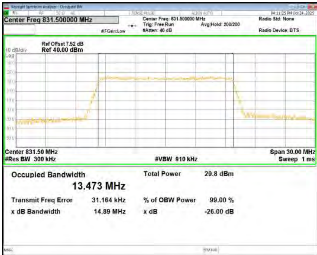
Band26(824-849) 16QAM BW=15MHz Channel=26915 RB Size=75 Position=#0
