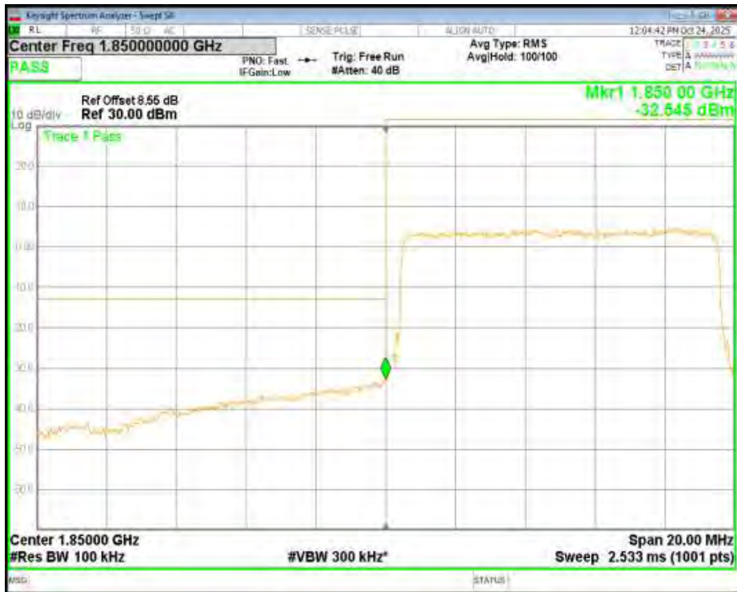
Band2 QPSK BW=10MHz Channel=19150 RB Size=50 Position=#0
