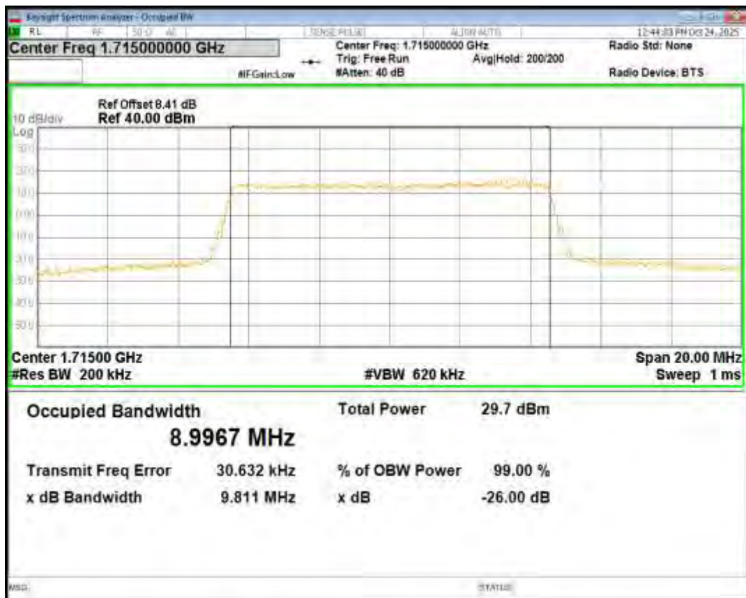
Band4 QPSK BW=10MHz Channel=20175 RB Size=50 Position=#0
