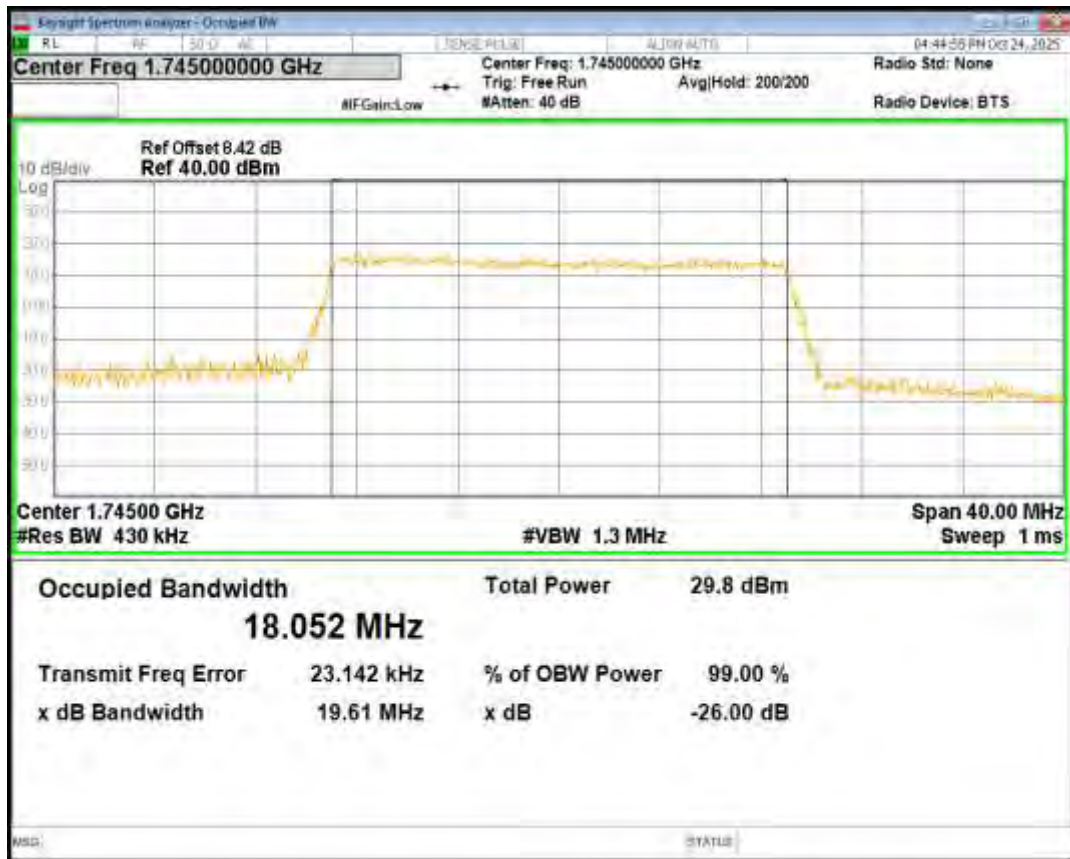
Band66 16QAM BW=20MHz Channel=132572 RB Size=100 Position=#0
