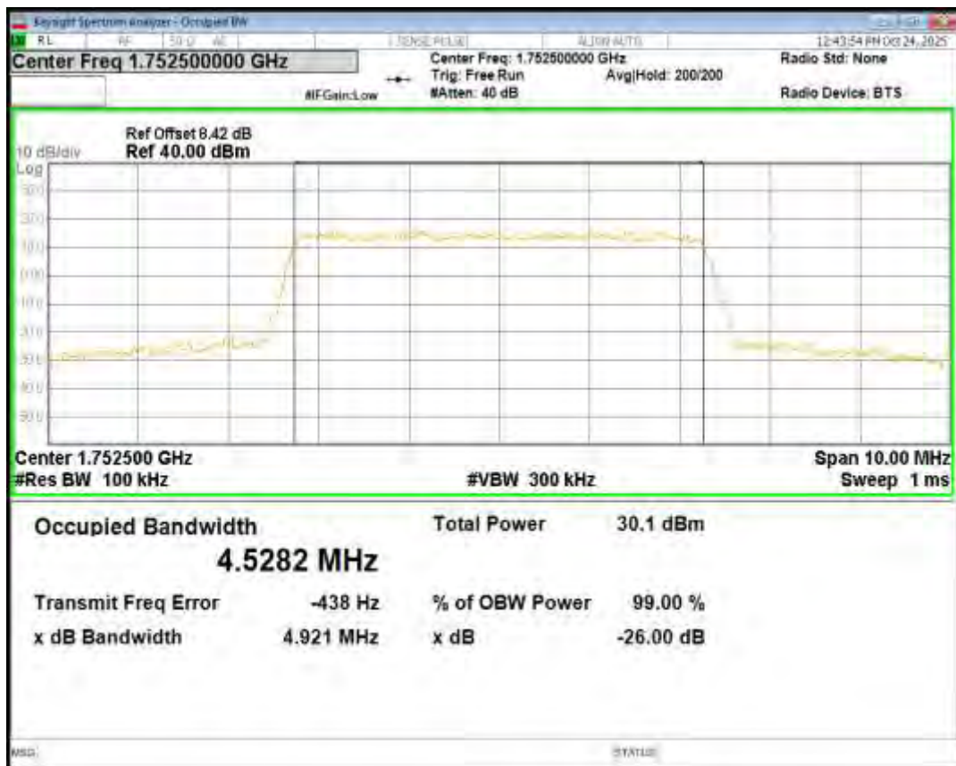
Band5 16QAM BW=1.4MHz Channel=20407 RB Size=6 Position=#0
