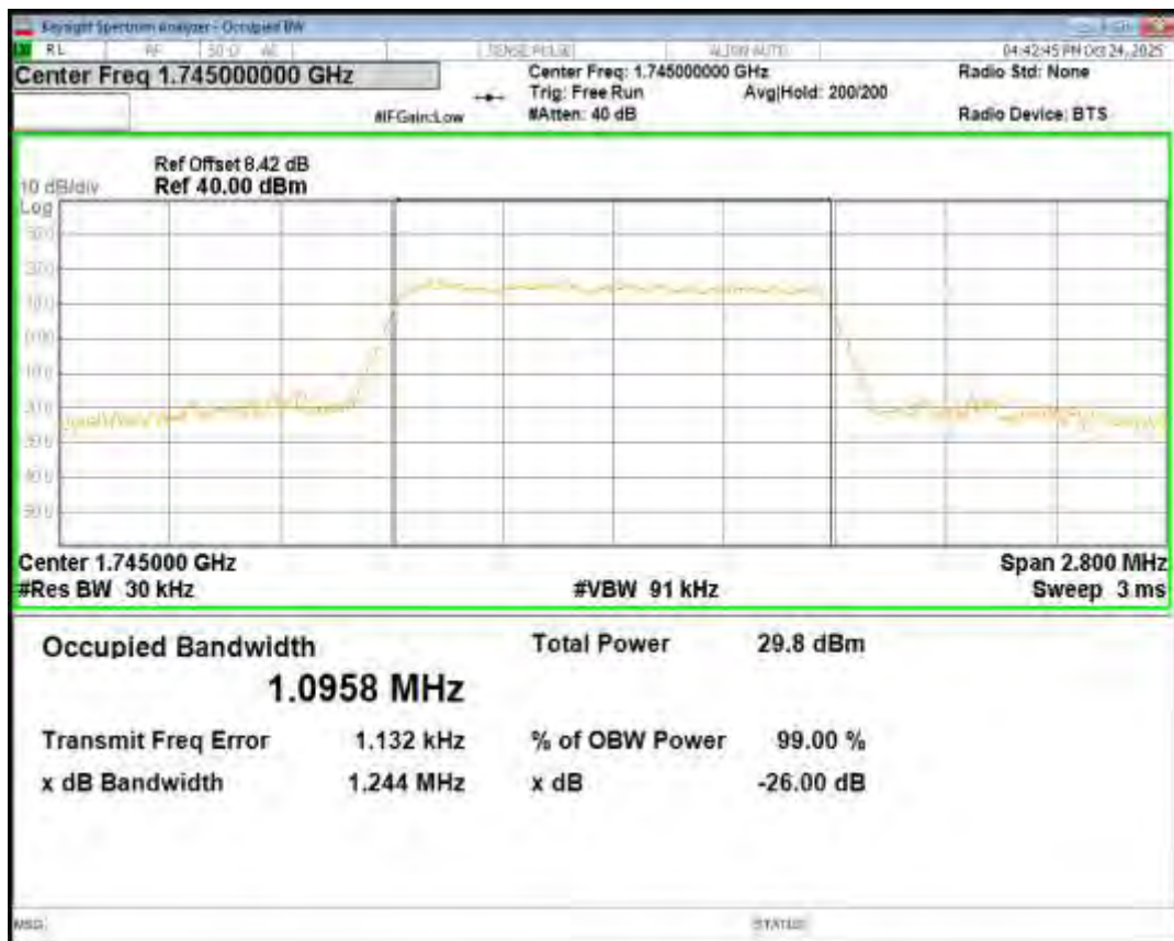
Band66 16QAM BW=1.4MHz Channel=132665 RB Size=6 Position=#0
