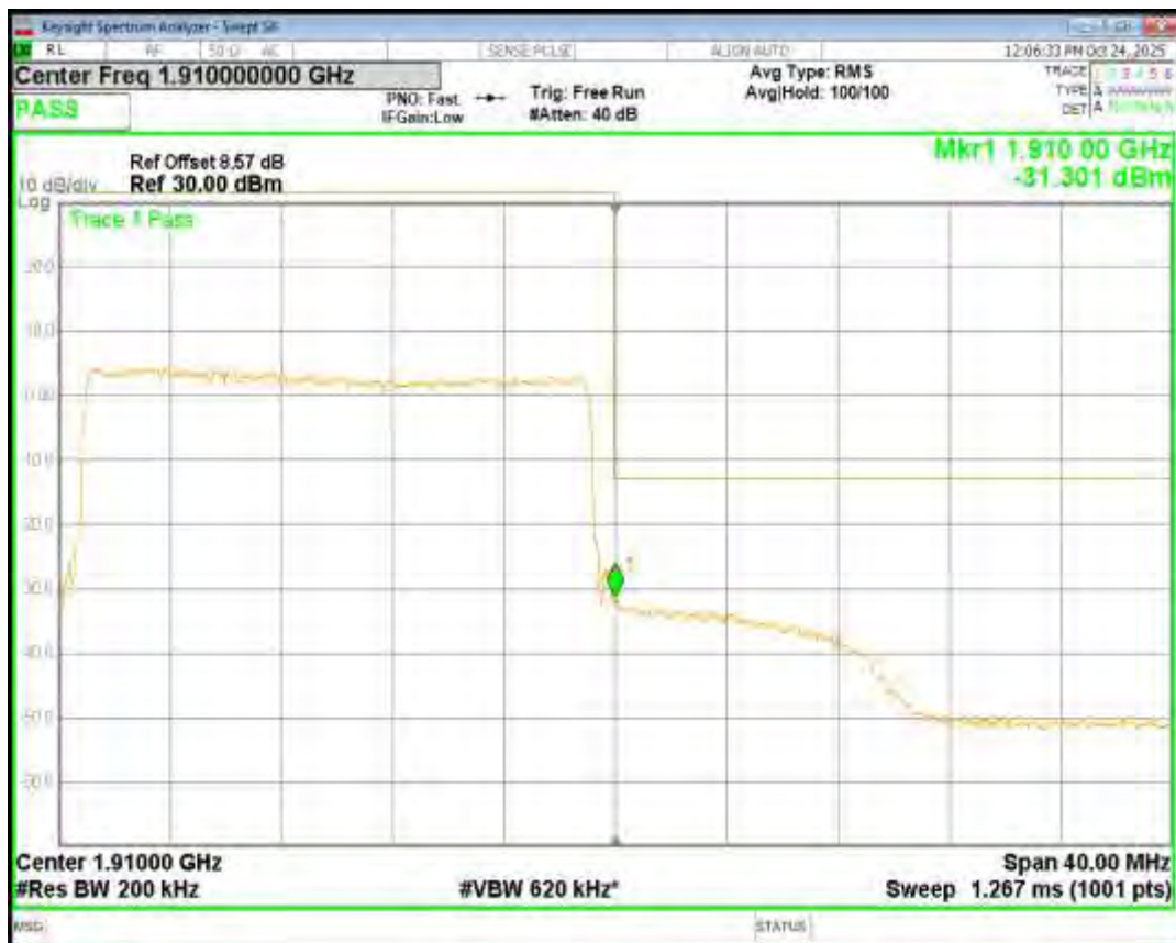
Band2 16QAM BW=3MHz Channel=18615 RB Size=15 Position=#0
