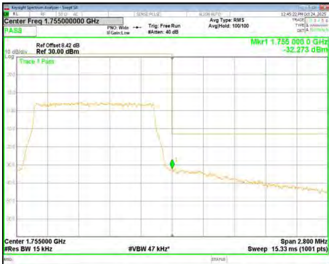
Band4 16QAM BW=10MHz Channel=20000 RB Size=50 Position=#0
