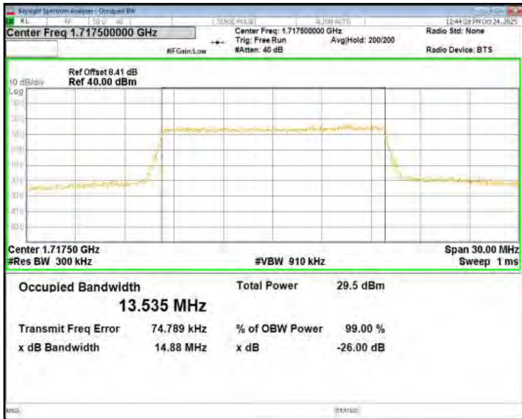
Band4 16QAM BW=15MHz Channel=20175 RB Size=75 Position=#0
