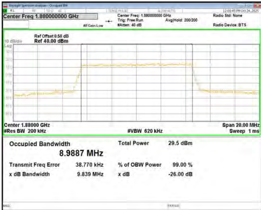
Band2 16QAM BW=10MHz Channel=19150 RB Size=50 Position=#0
