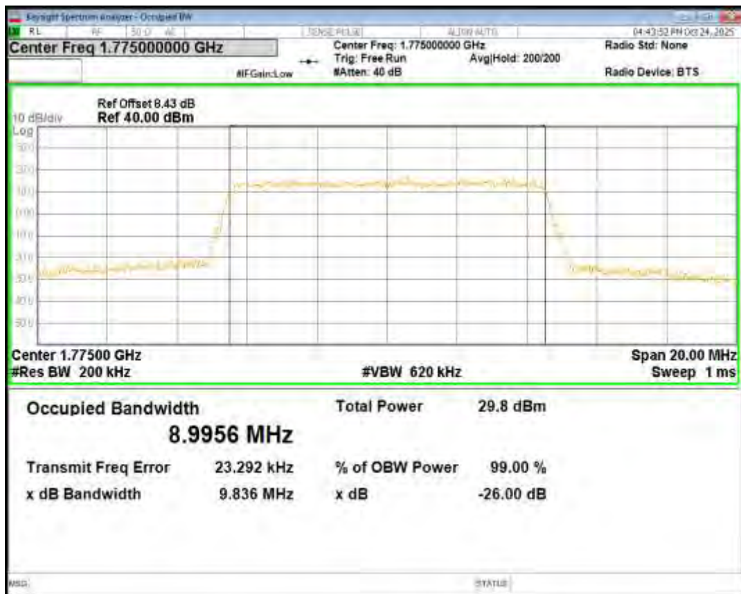
Band66 16QAM BW=15MHz Channel=132047 RB Size=75 Position=#0
