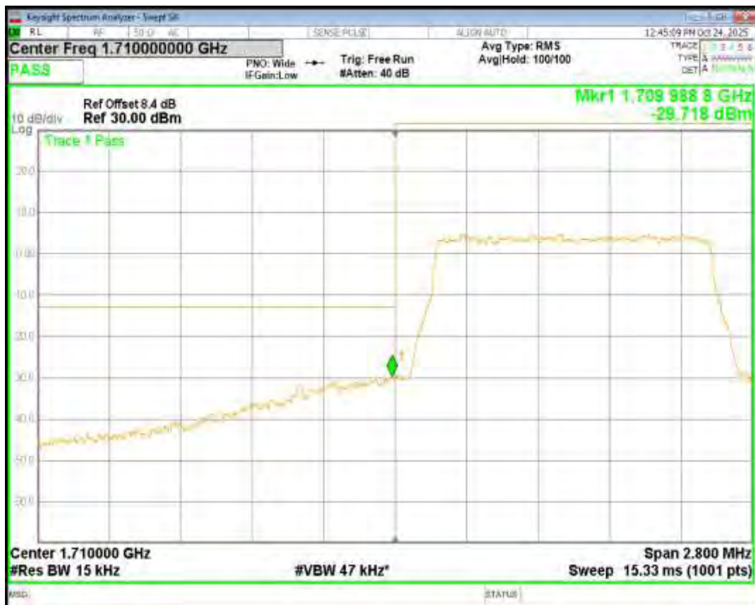
Band4 QPSK BW=10MHz Channel=20000 RB Size=50 Position=#0
