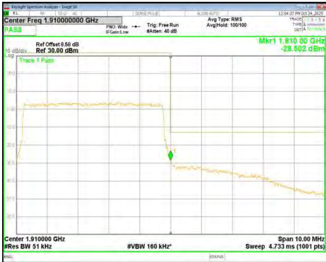
Band2 16QAM BW=3MHz Channel=19185 RB Size=15 Position=#0
