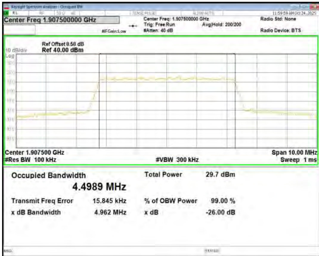
Band2 16QAM BW=5MHz Channel=18625 RB Size=25 Position=#0
