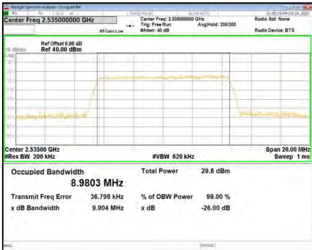
Band7 QPSK BW=10MHz Channel=21400 RB Size=50 Position=#0
