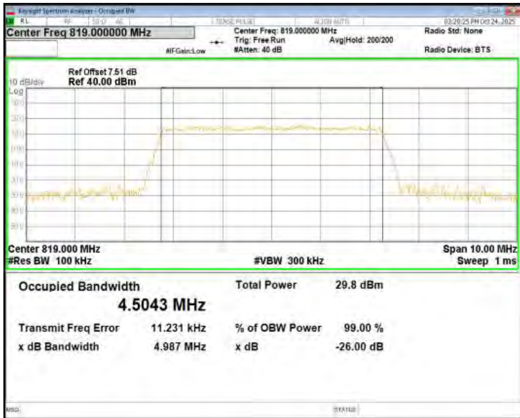
Band26(814-824) QPSK BW=1.4MHz Channel=26783 RB Size=6 Position=#0
