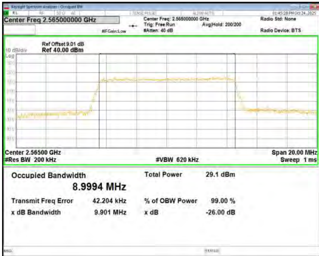
Band7 16QAM BW=15MHz Channel=20825 RB Size=75 Position=#0
