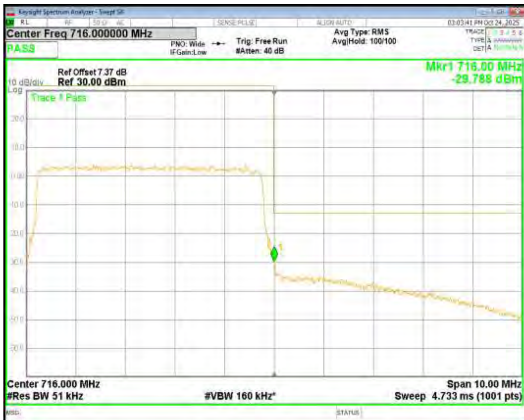
Band17 QPSK BW=10MHz Channel=23780 RB Size=50 Position=#0
