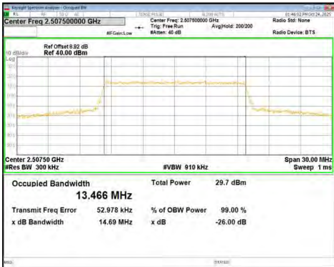
Band7 QPSK BW=15MHz Channel=21100 RB Size=75 Position=#0
