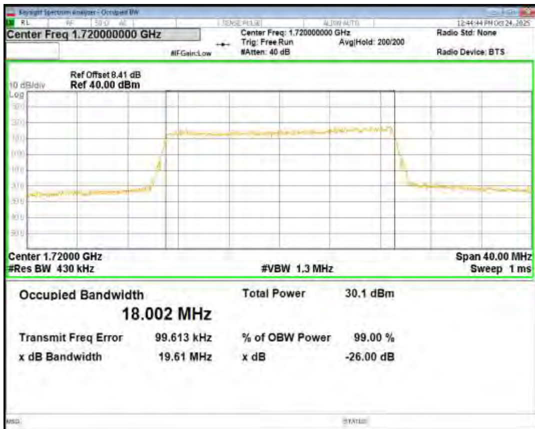
Band4 QPSK BW=20MHz Channel=20175 RB Size=100 Position=#0
