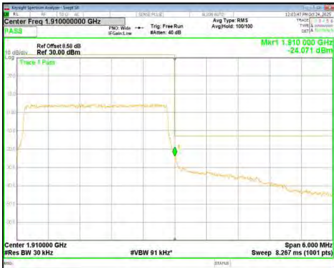
Band2 QPSK BW=5MHz Channel=18625 RB Size=25 Position=#0
