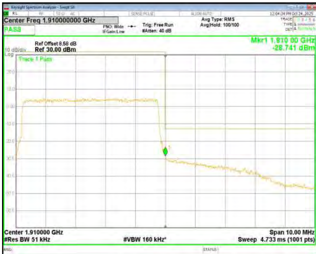
Band26(814-824) 16QAM BW=1.4MHz Channel=26697 RB Size=6 Position=#0
