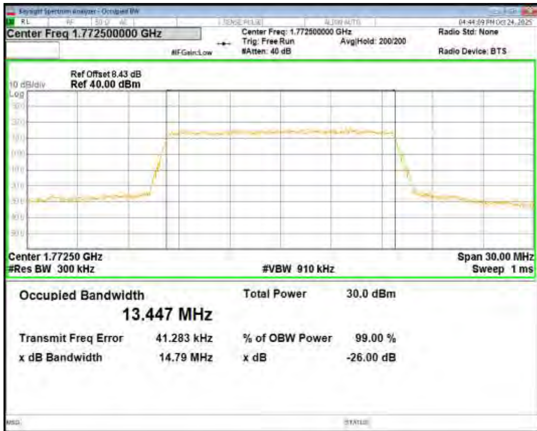
Band66 QPSK BW=20MHz Channel=132072 RB Size=100 Position=#0
