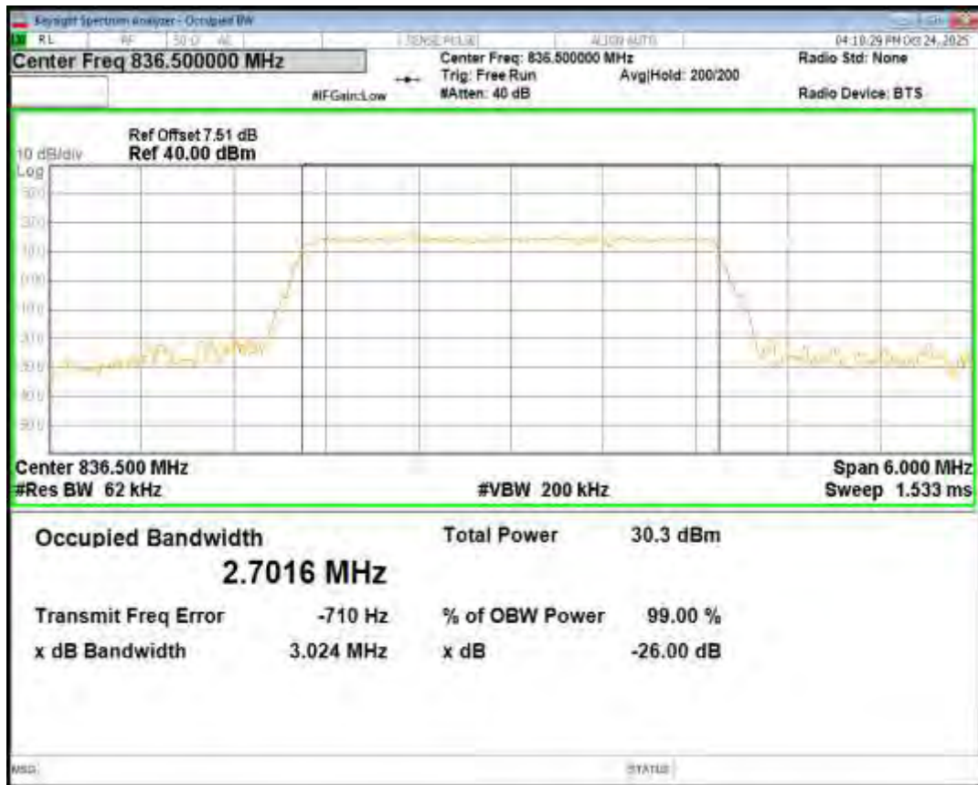
Band26(824-849) 16QAM BW=3MHz Channel=27025 RB Size=15 Position=#0
