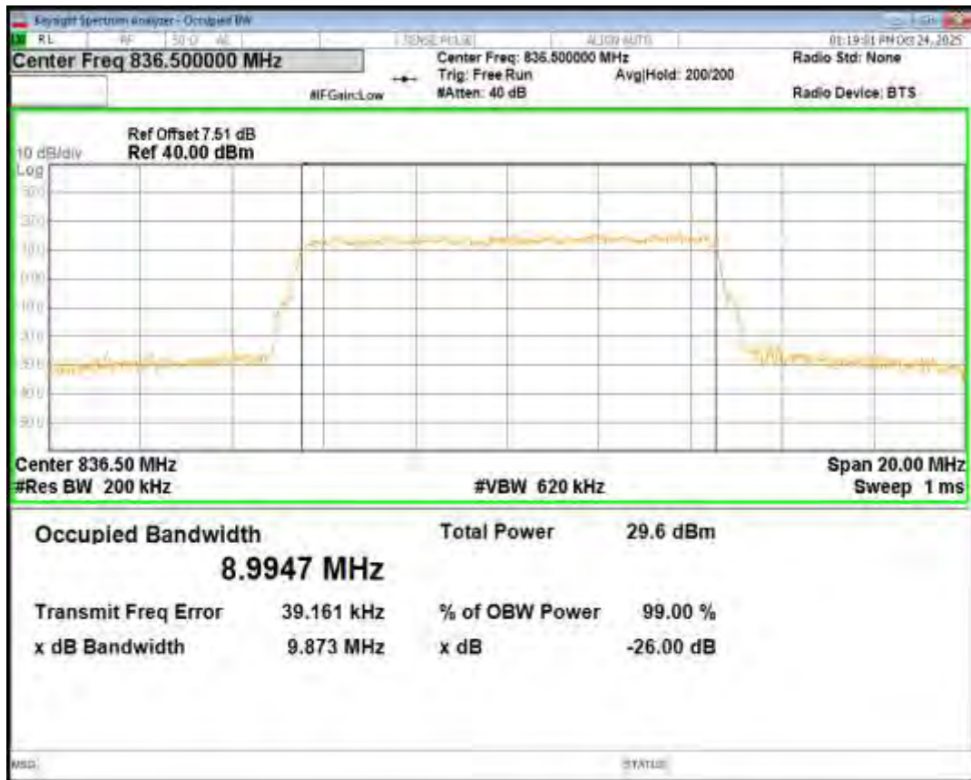
Band5 16QAM BW=10MHz Channel=20600 RB Size=50 Position=#0
