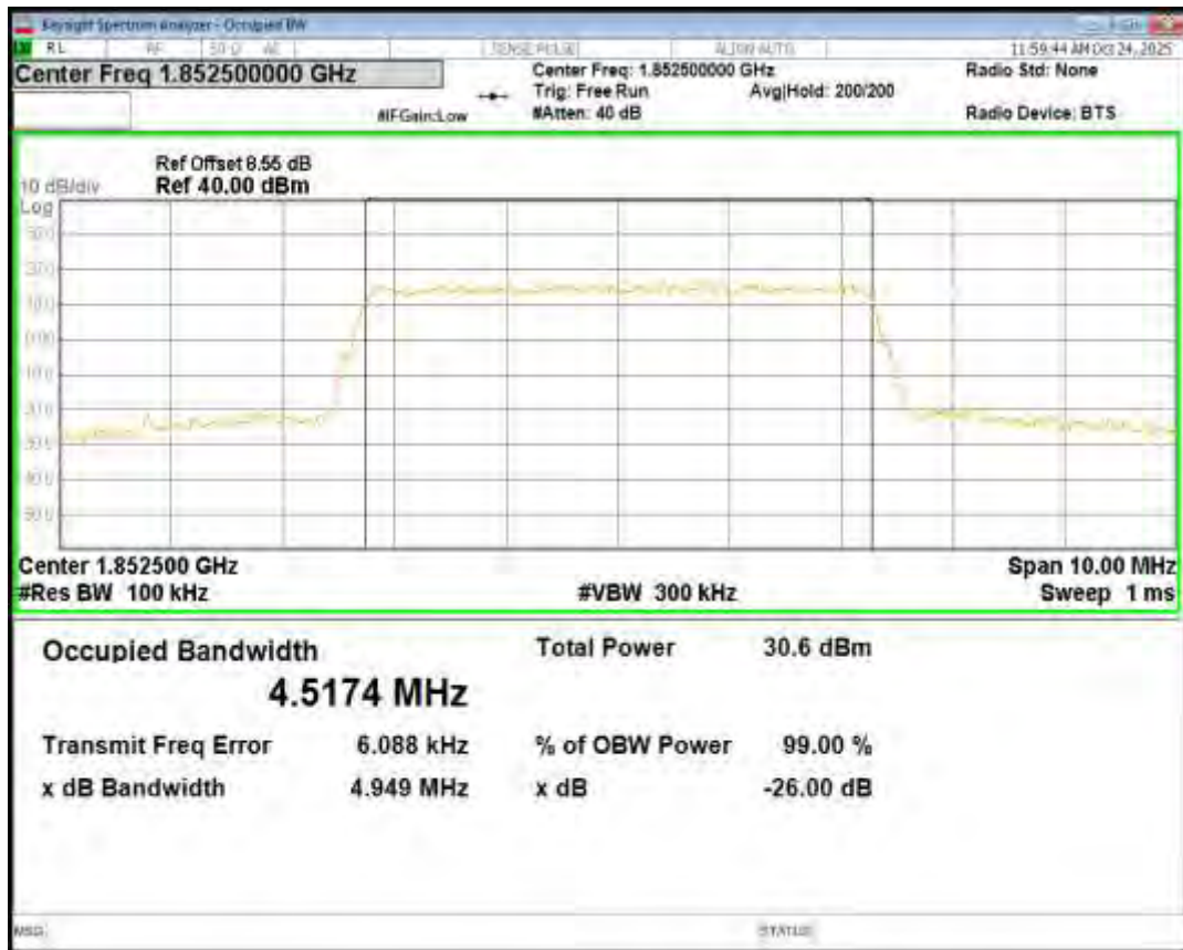
Band2 QPSK BW=5MHz Channel=19175 RB Size=25 Position=#0
