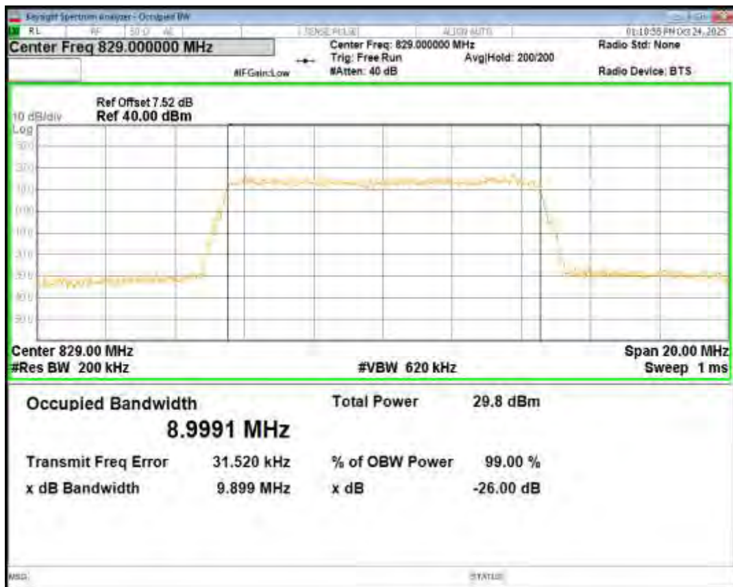
Band5 16QAM BW=10MHz Channel=20525 RB Size=50 Position=#0
