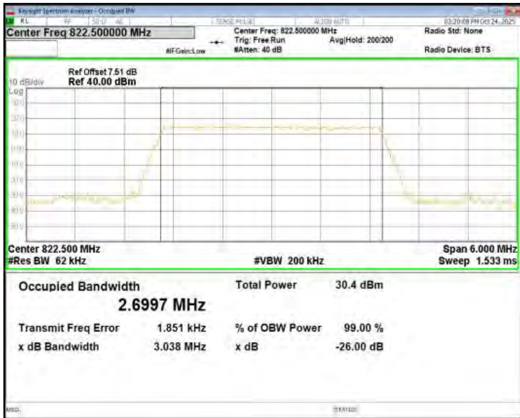
Band26(814-824) QPSK BW=5MHz Channel=26740 RB Size=25 Position=#0
