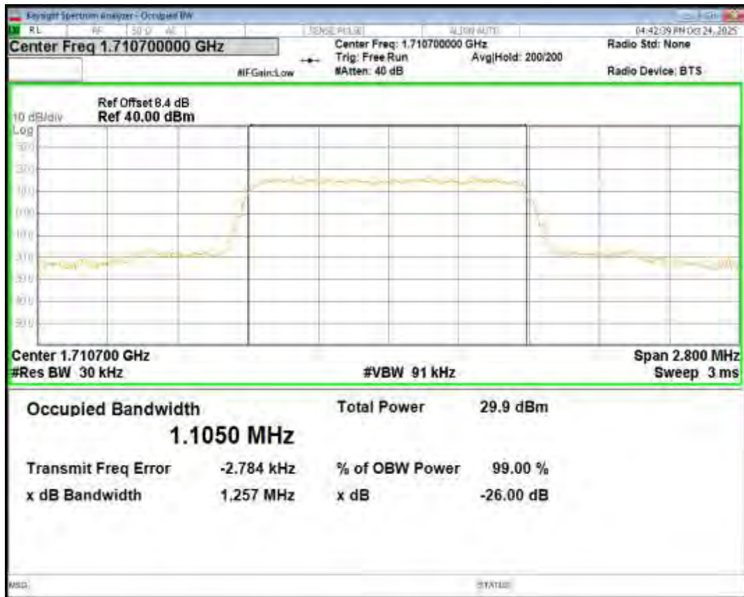
Band66 16QAM BW=1.4MHz Channel=132322 RB Size=6 Position=#0
