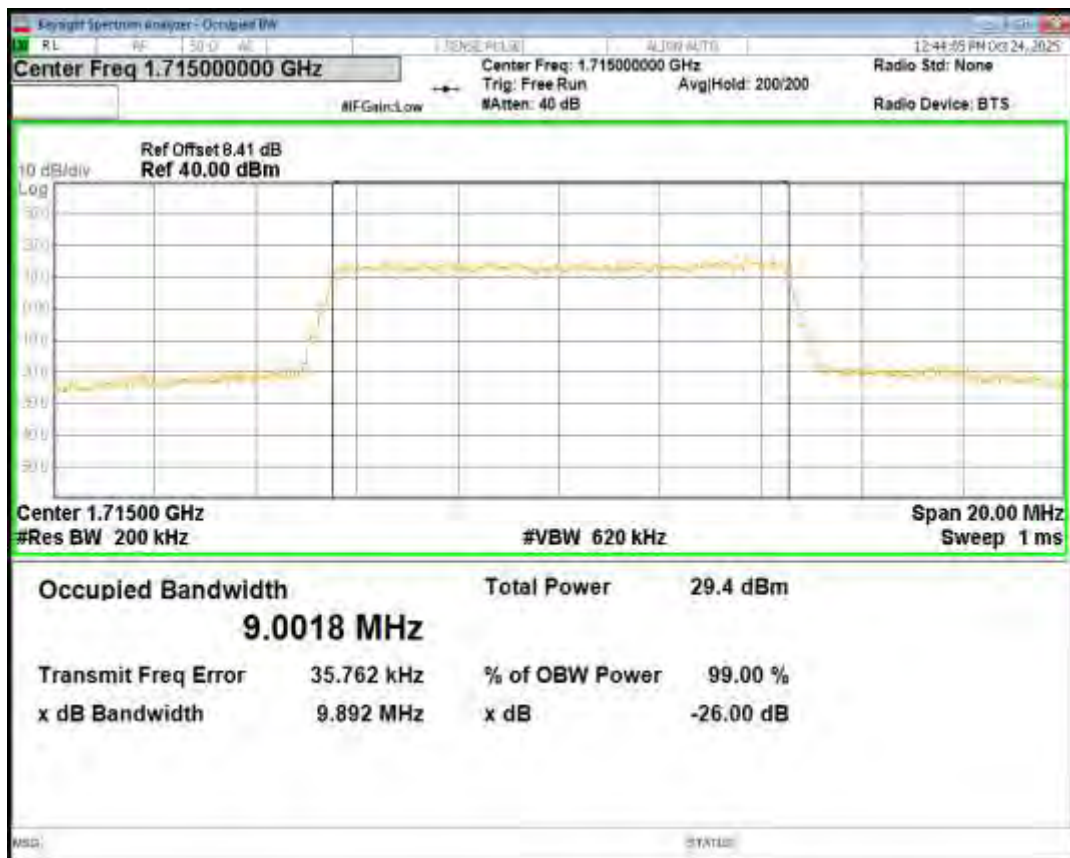
Band4 16QAM BW=10MHz Channel=20175 RB Size=50 Position=#0
