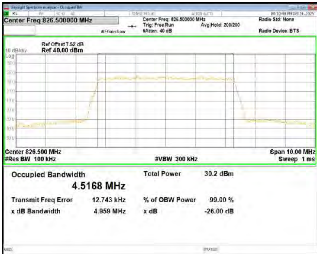
Band26(824-849) QPSK BW=5MHz Channel=26915 RB Size=25 Position=#0
