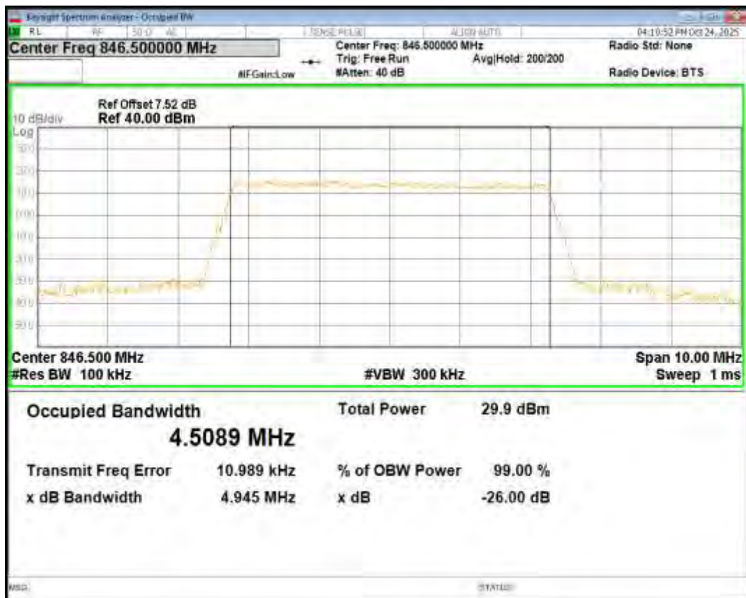
Band4 16QAM BW=1.4MHz Channel=19957 RB Size=6 Position=#0
