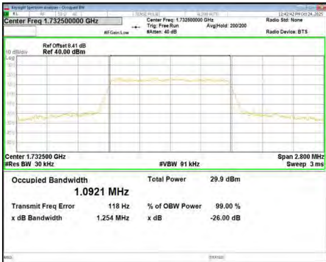
Band4 16QAM BW=1.4MHz Channel=20393 RB Size=6 Position=#0
