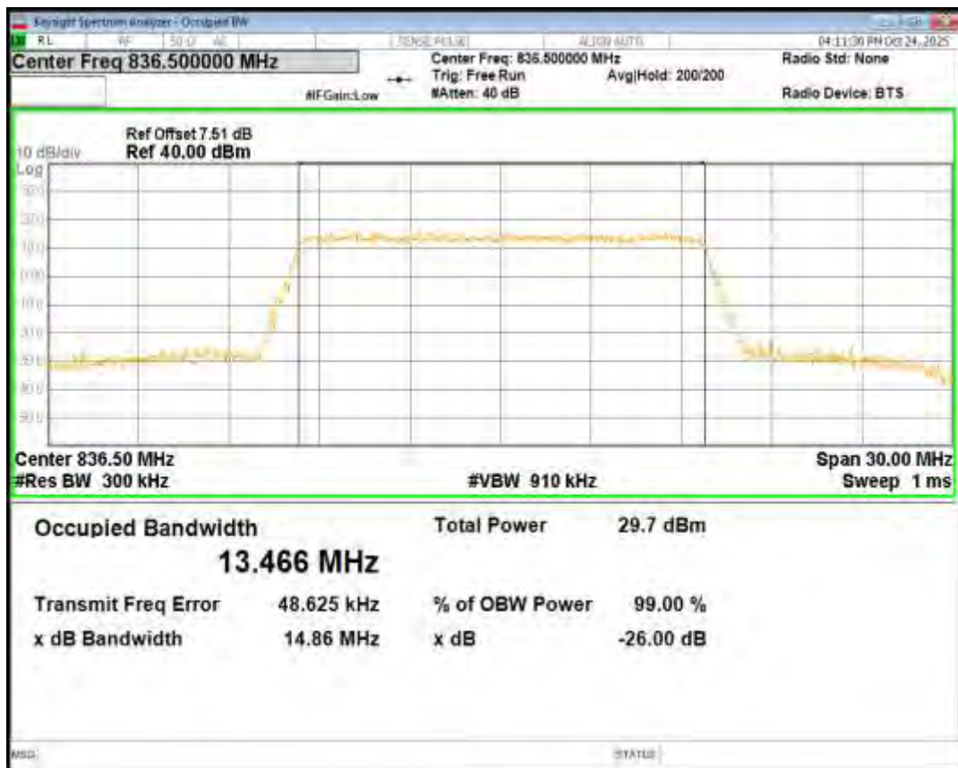
Band26(824-849) 16QAM BW=15MHz Channel=26965 RB Size=75 Position=#0
