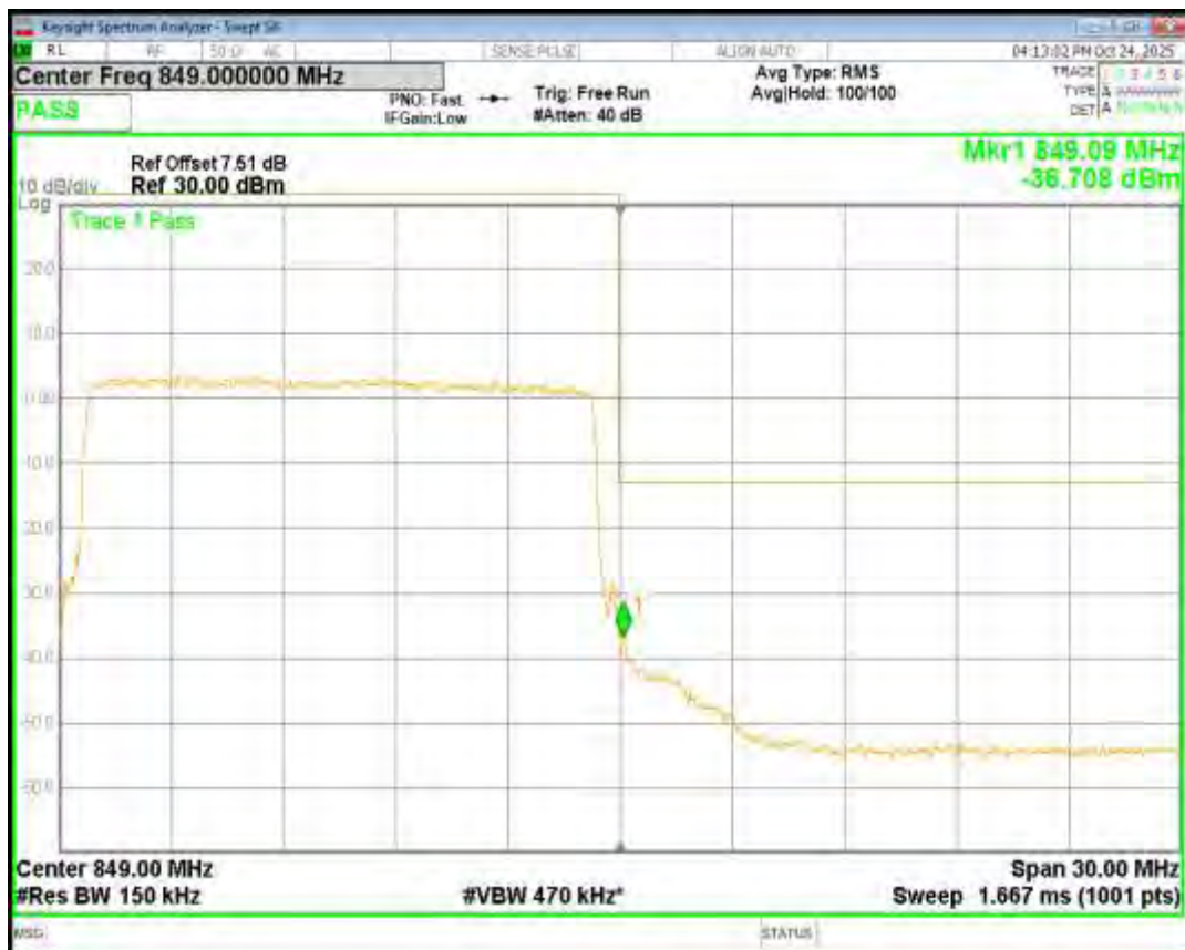
Band26(824-849) 16QAM BW=3MHz Channel=26805 RB Size=15 Position=#0
