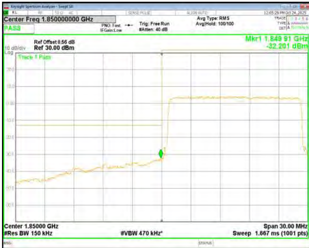
Band2 QPSK BW=15MHz Channel=19125 RB Size=75 Position=#0
