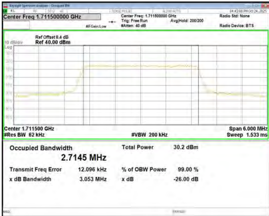
Band66 16QAM BW=3MHz Channel=132322 RB Size=15 Position=#0
