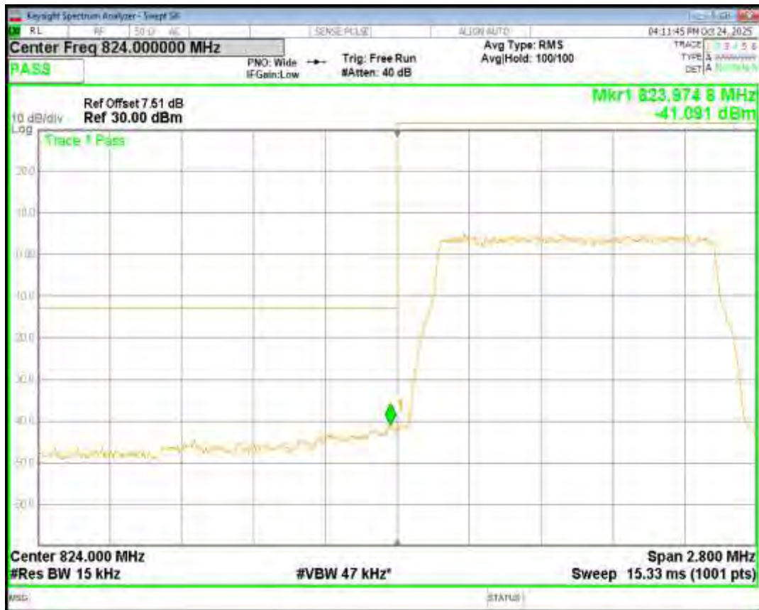
Band26(824-849) QPSK BW=1.4MHz Channel=27033 RB Size=6 Position=#0
