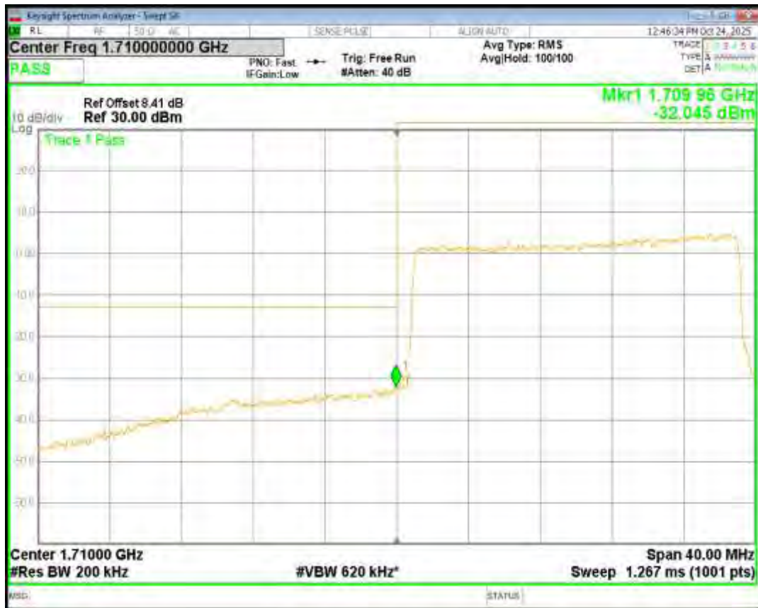
Band4 16QAM BW=20MHz Channel=20300 RB Size=100 Position=#0
