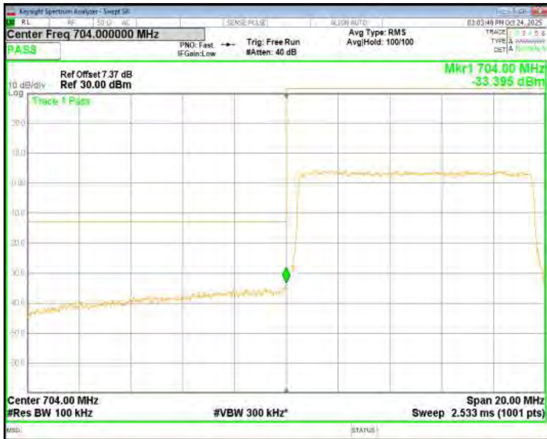
Band17 QPSK BW=10MHz Channel=23800 RB Size=50 Position=#0
