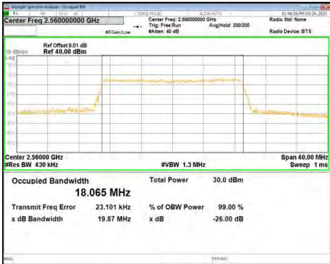
Band7 QPSK BW=5MHz Channel=20775 RB Size=25 Position=#0
