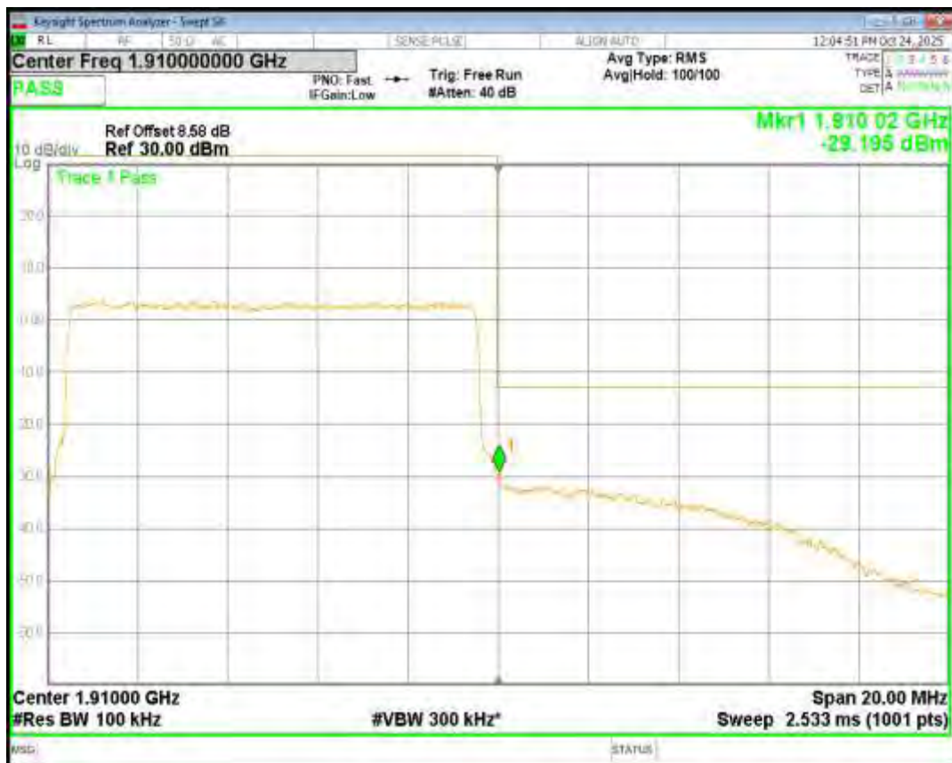
Band2 16QAM BW=15MHz Channel=18675 RB Size=75 Position=#0
