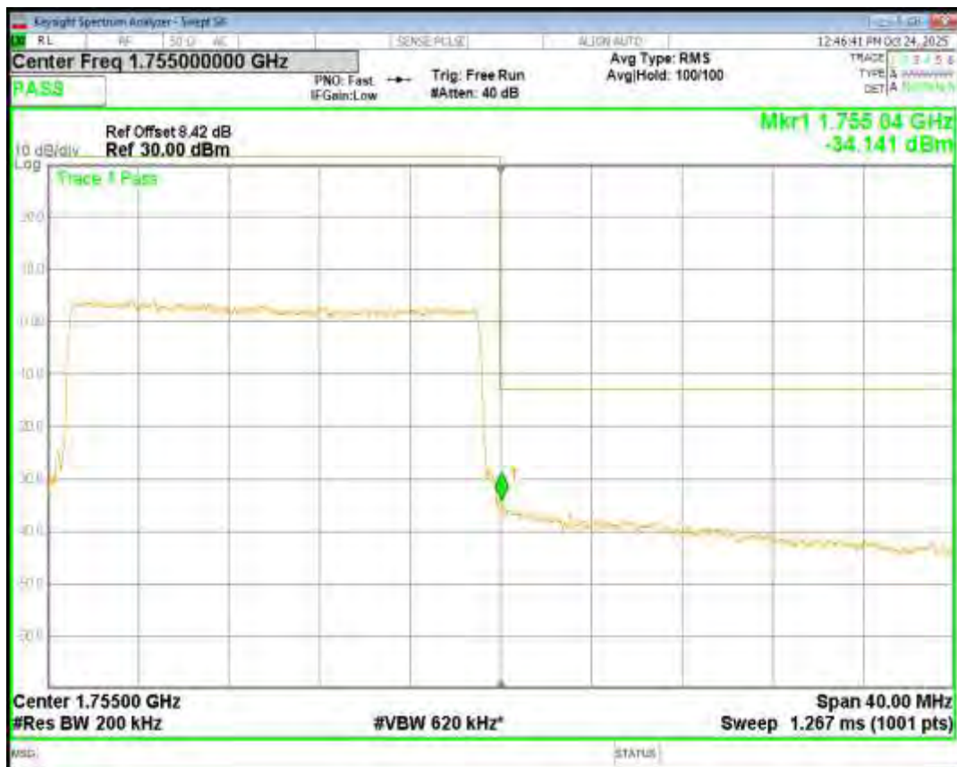
Band4 16QAM BW=3MHz Channel=19965 RB Size=15 Position=#0
