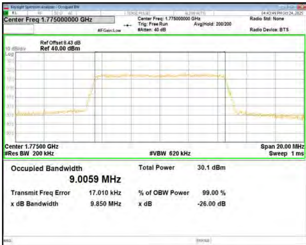
Band66 QPSK BW=15MHz Channel=132047 RB Size=75 Position=#0
