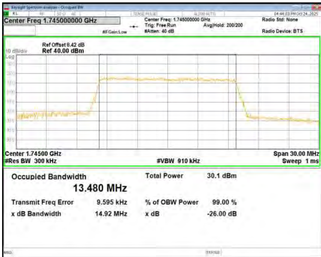
Band66 QPSK BW=15MHz Channel=132597 RB Size=75 Position=#0
