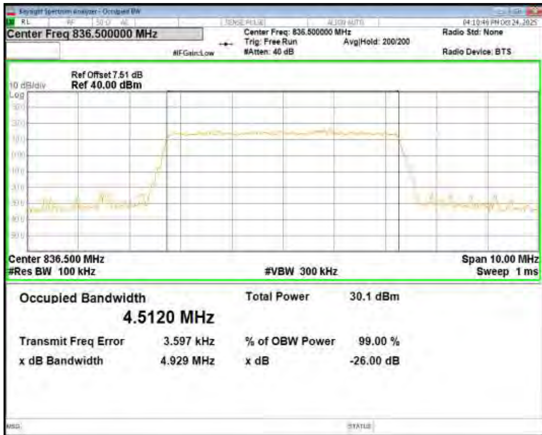
Band26(824-849) QPSK BW=5MHz Channel=27015 RB Size=25 Position=#0
