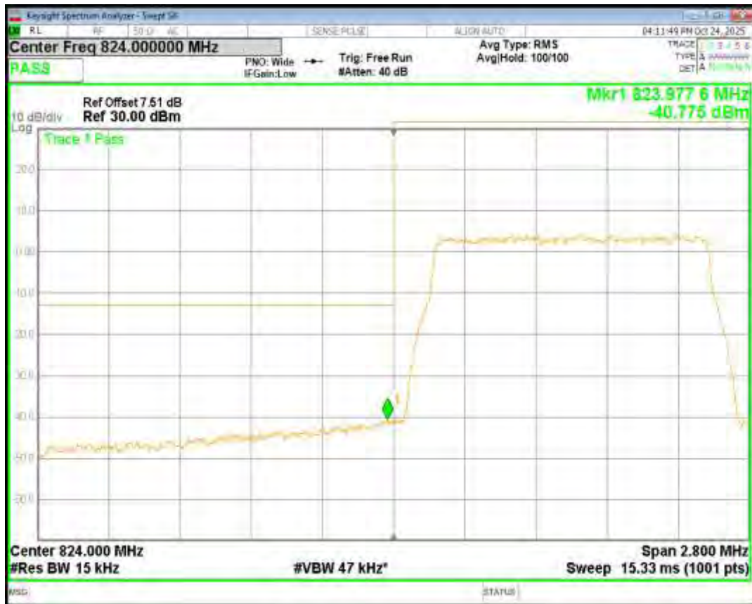
Band26(824-849) 16QAM BW=1.4MHz Channel=27033 RB Size=6 Position=#0
