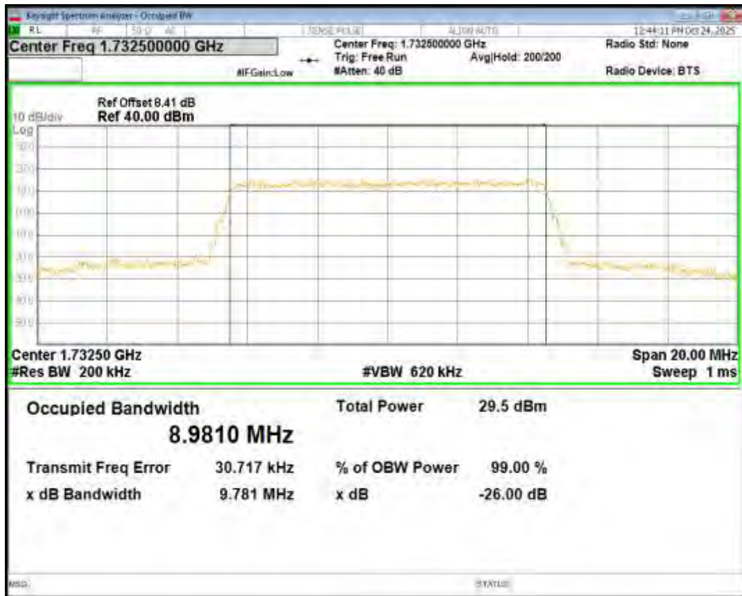
Band4 16QAM BW=10MHz Channel=20350 RB Size=50 Position=#0
