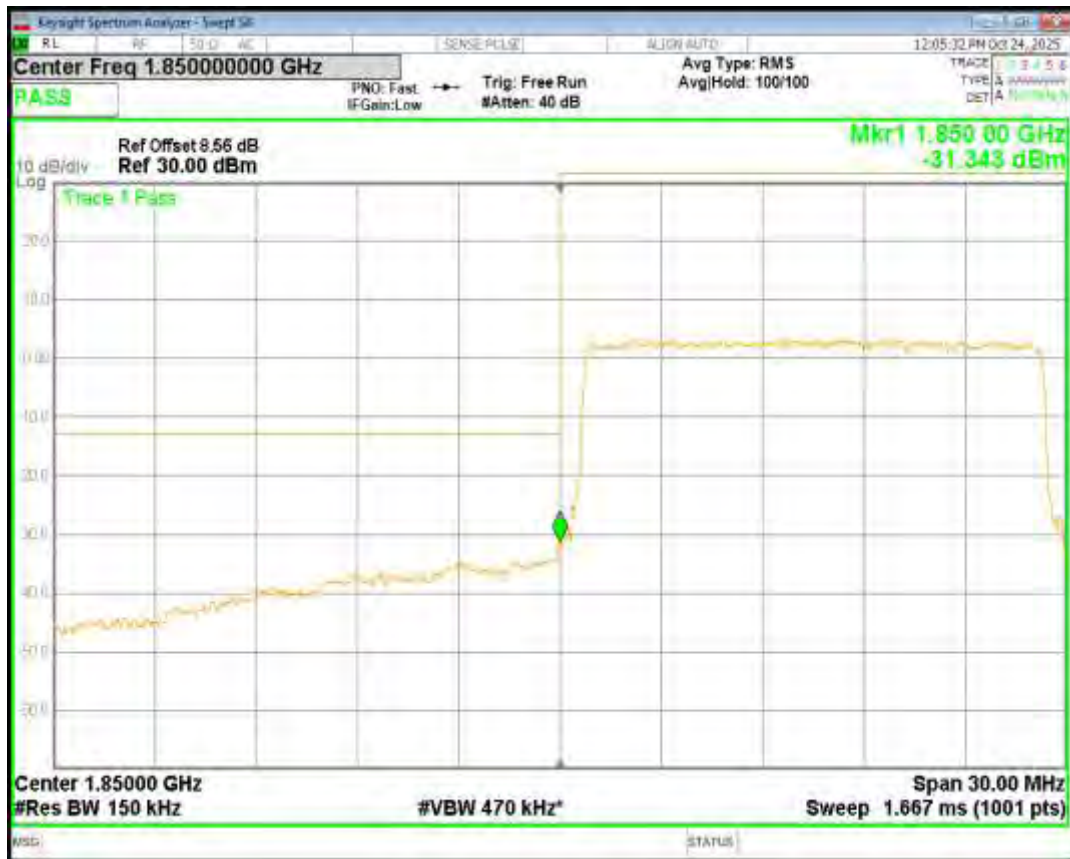
Band2 16QAM BW=15MHz Channel=19125 RB Size=75 Position=#0
