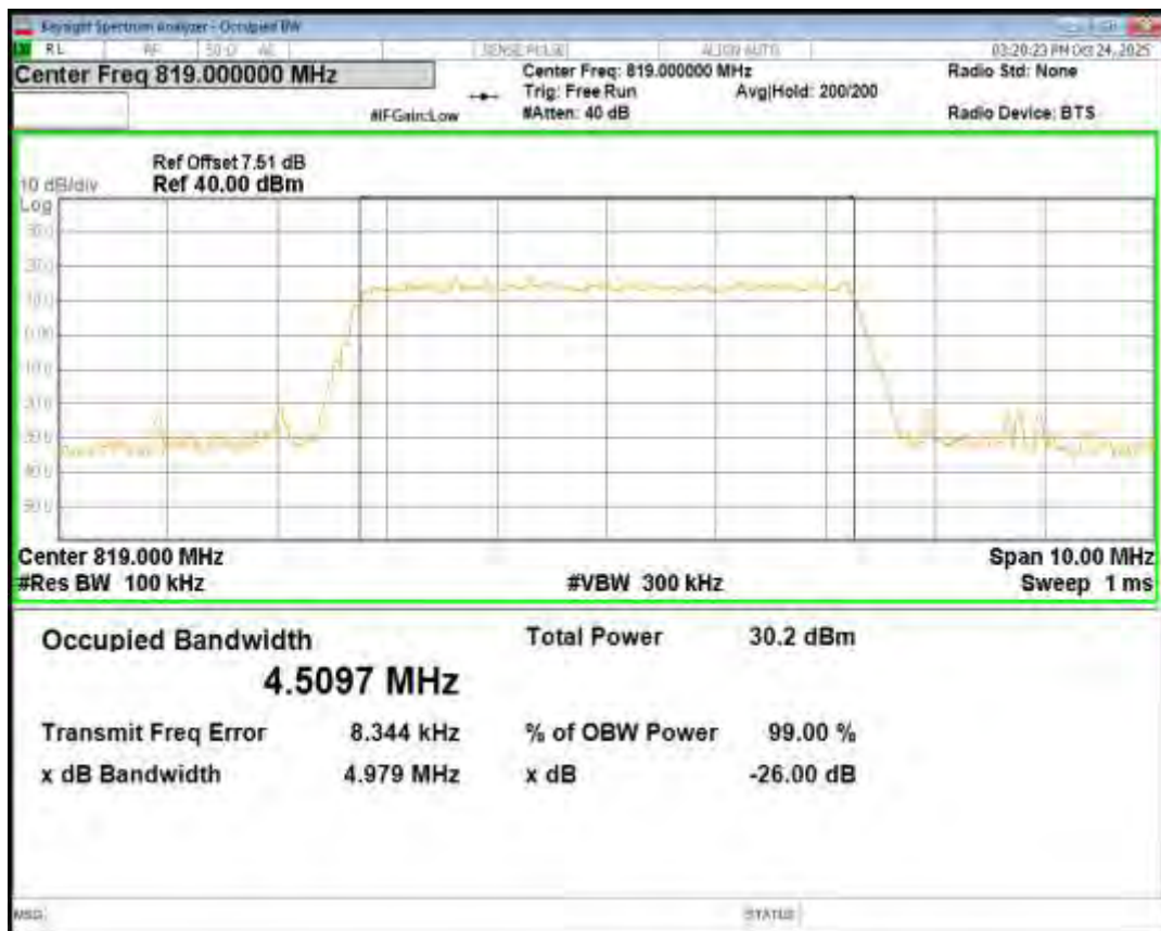
Band26(814-824) QPSK BW=5MHz Channel=26715 RB Size=25 Position=#0
