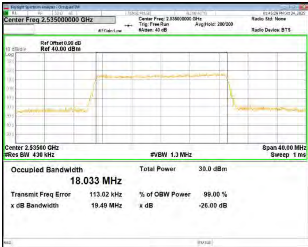
Band7 QPSK BW=20MHz Channel=21350 RB Size=100 Position=#0
