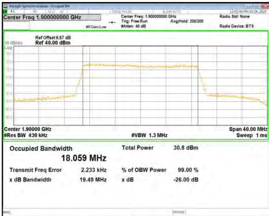
Band2 QPSK BW=3MHz Channel=18615 RB Size=15 Position=#0
