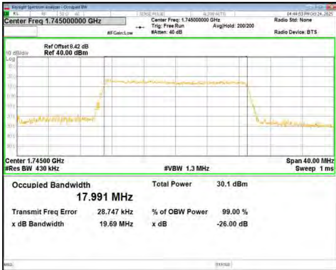
Band66 QPSK BW=20MHz Channel=132572 RB Size=100 Position=#0
