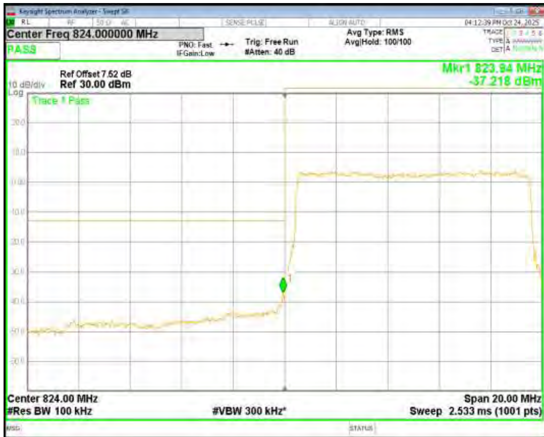
Band26(824-849) QPSK BW=10MHz Channel=26990 RB Size=50 Position=#0
