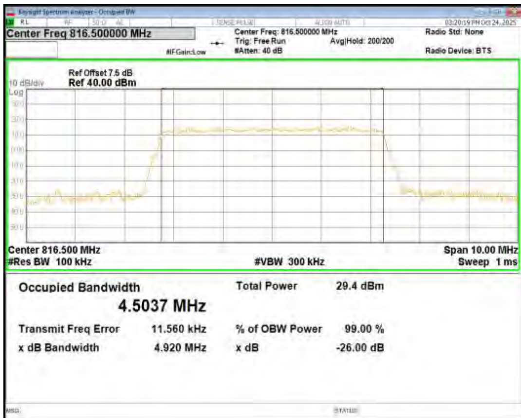
Band26(814-824) 16QAM BW=5MHz Channel=26740 RB Size=25 Position=#0
