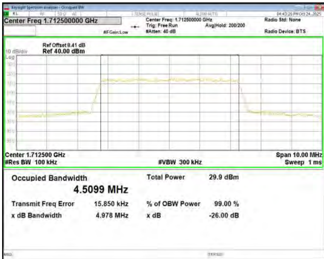
Band66 16QAM BW=5MHz Channel=132322 RB Size=25 Position=#0
