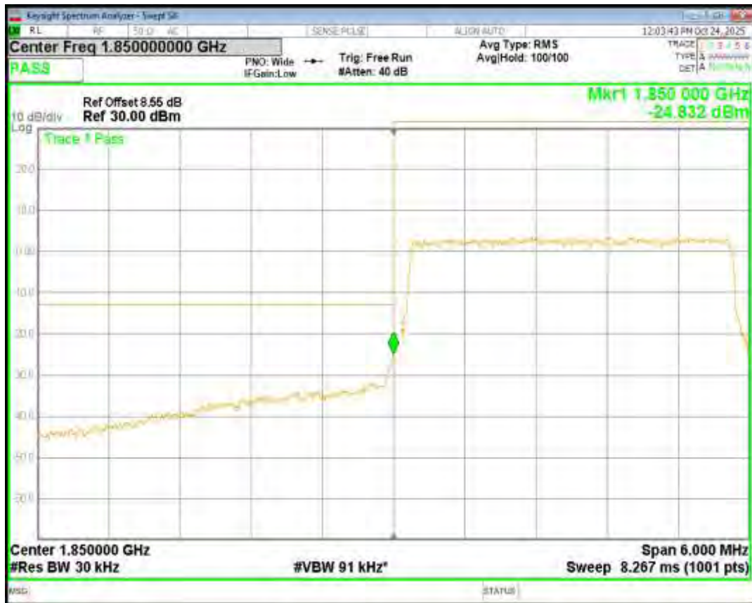
Band2 QPSK BW=1.4MHz Channel=18607 RB Size=6 Position=#0
