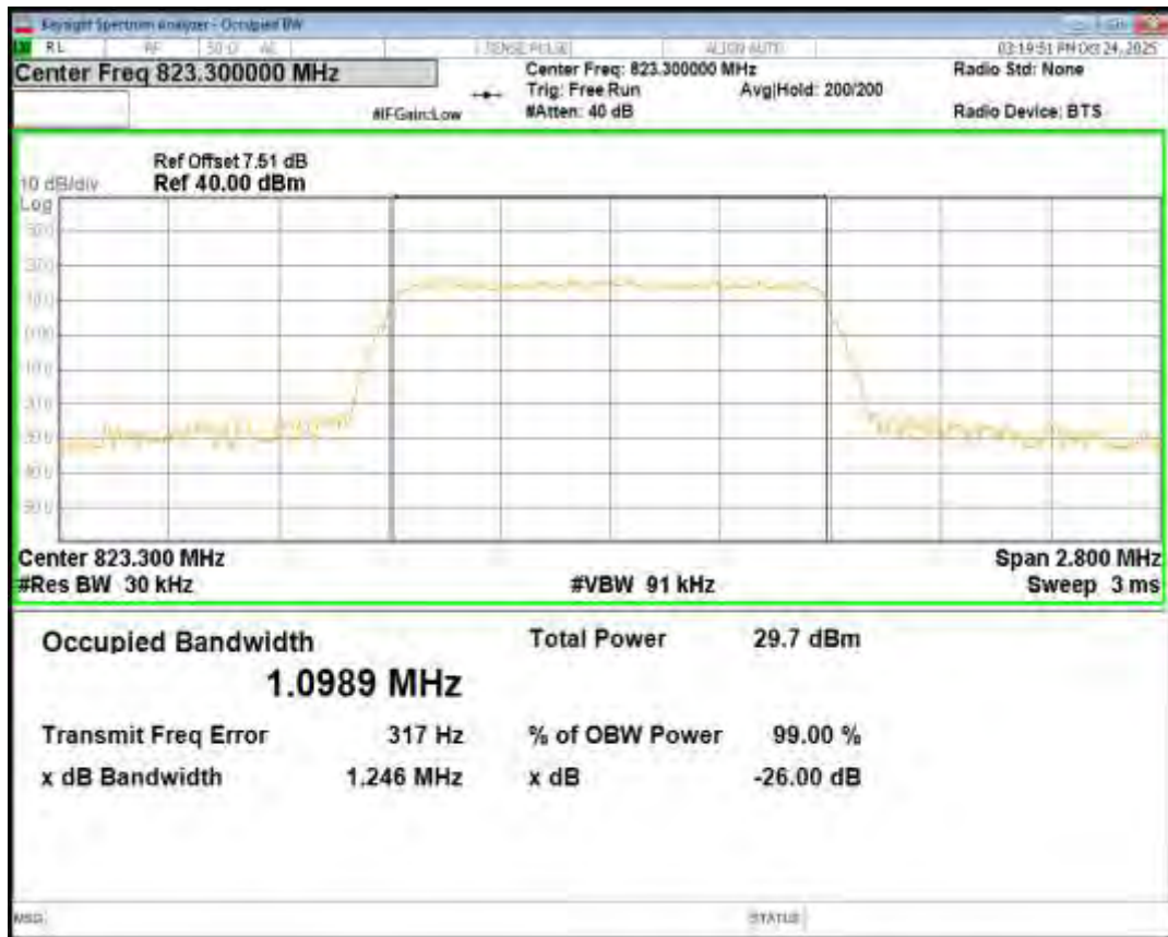
Band26(814-824) 16QAM BW=10MHz Channel=26740 RB Size=50 Position=#0
