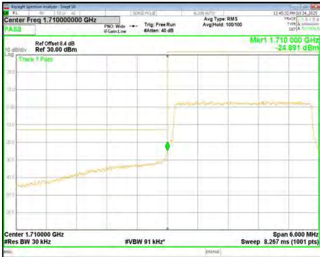
Band4 16QAM BW=3MHz Channel=20385 RB Size=15 Position=#0
