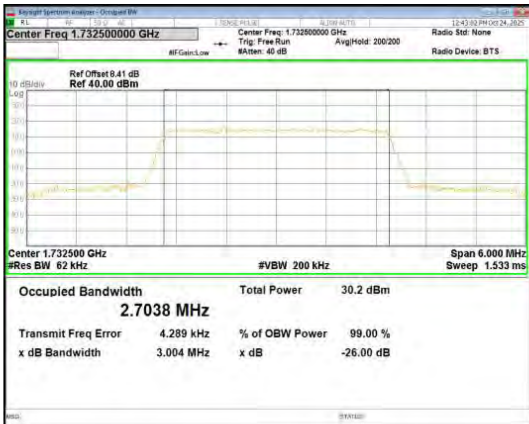
Band4 16QAM BW=3MHz Channel=20385 RB Size=15 Position=#0
