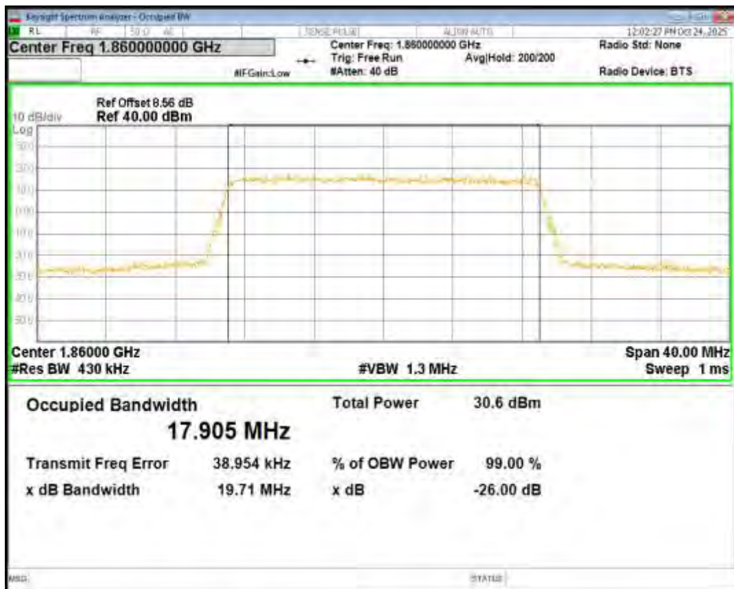
Band2 QPSK BW=20MHz Channel=18900 RB Size=100 Position=#0
