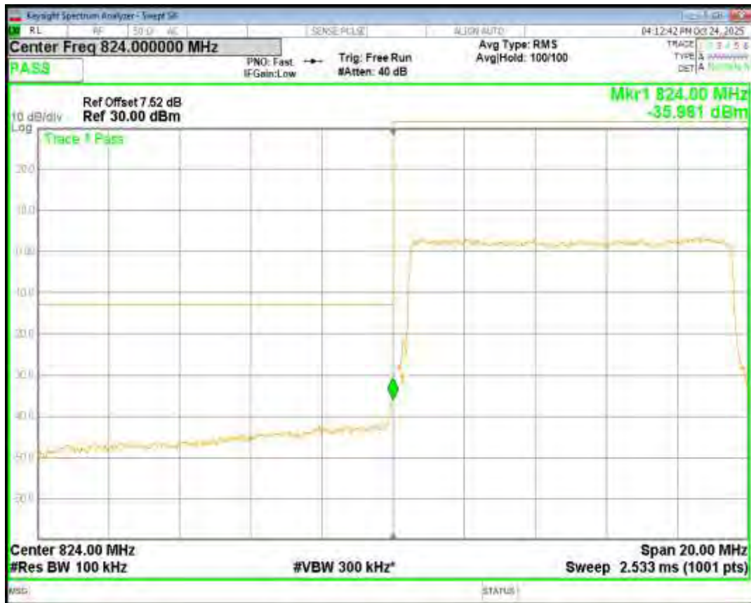
Band26(824-849) 16QAM BW=10MHz Channel=26990 RB Size=50 Position=#0
