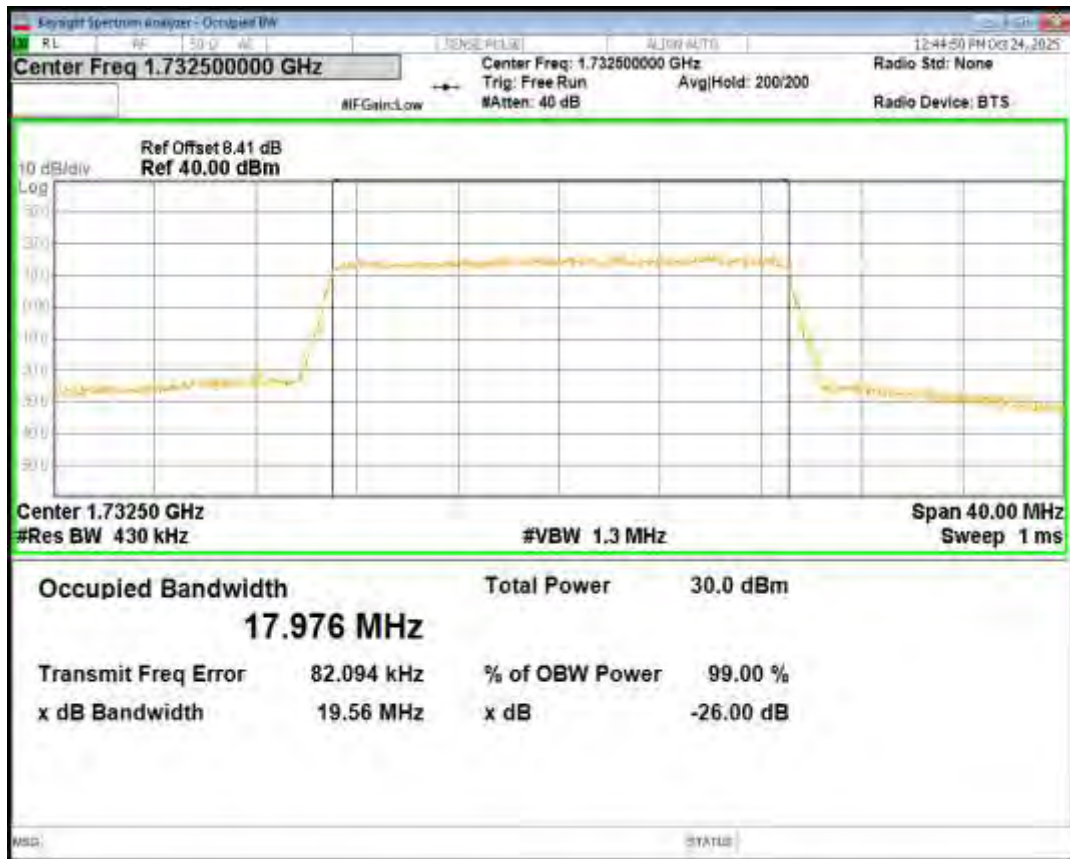
Band4 QPSK BW=3MHz Channel=20385 RB Size=15 Position=#0
