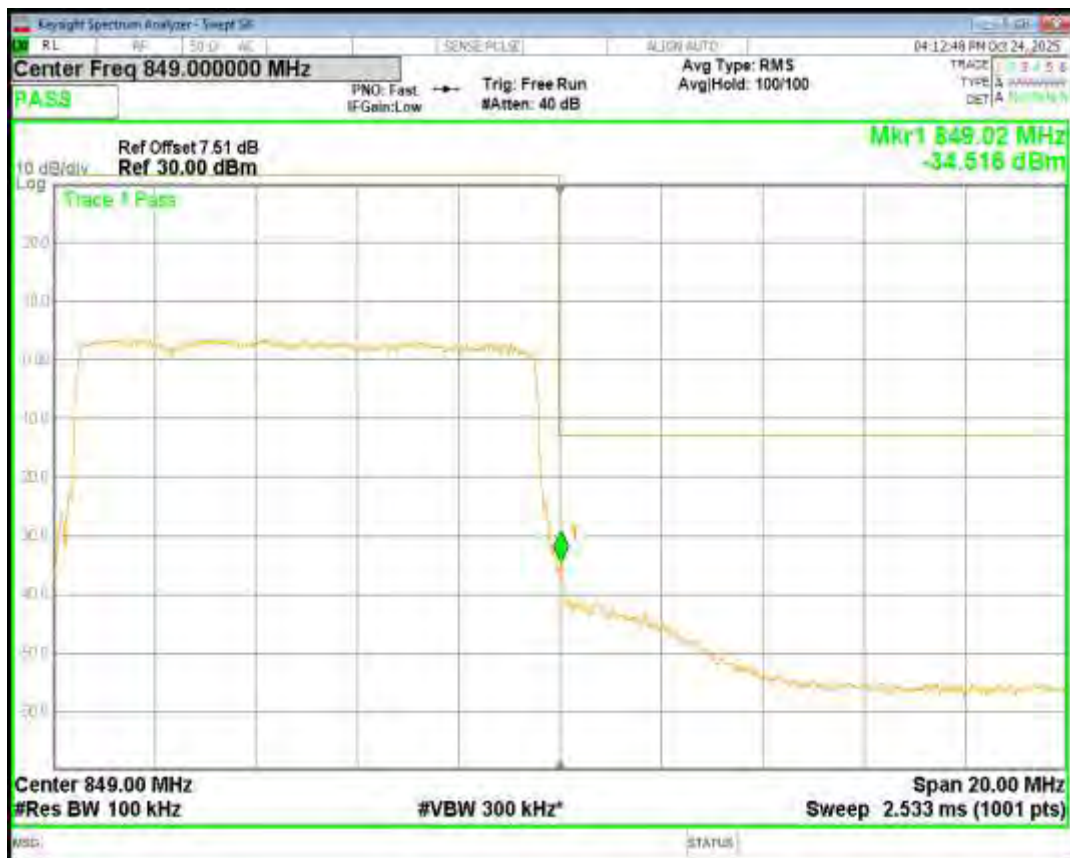
Band26(824-849) 16QAM BW=15MHz Channel=26865 RB Size=75 Position=#0
