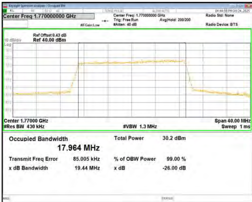
Band66 QPSK BW=3MHz Channel=131987 RB Size=15 Position=#0
