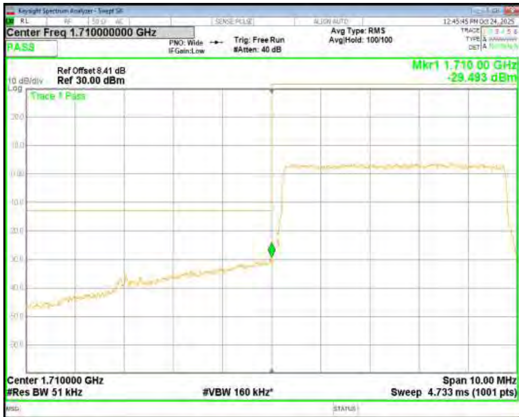
Band4 QPSK BW=5MHz Channel=20375 RB Size=25 Position=#0
