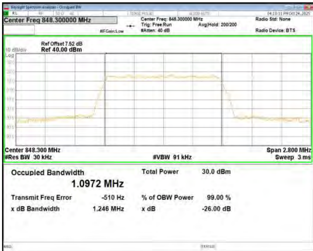
Band26(824-849) QPSK BW=10MHz Channel=26840 RB Size=50 Position=#0
