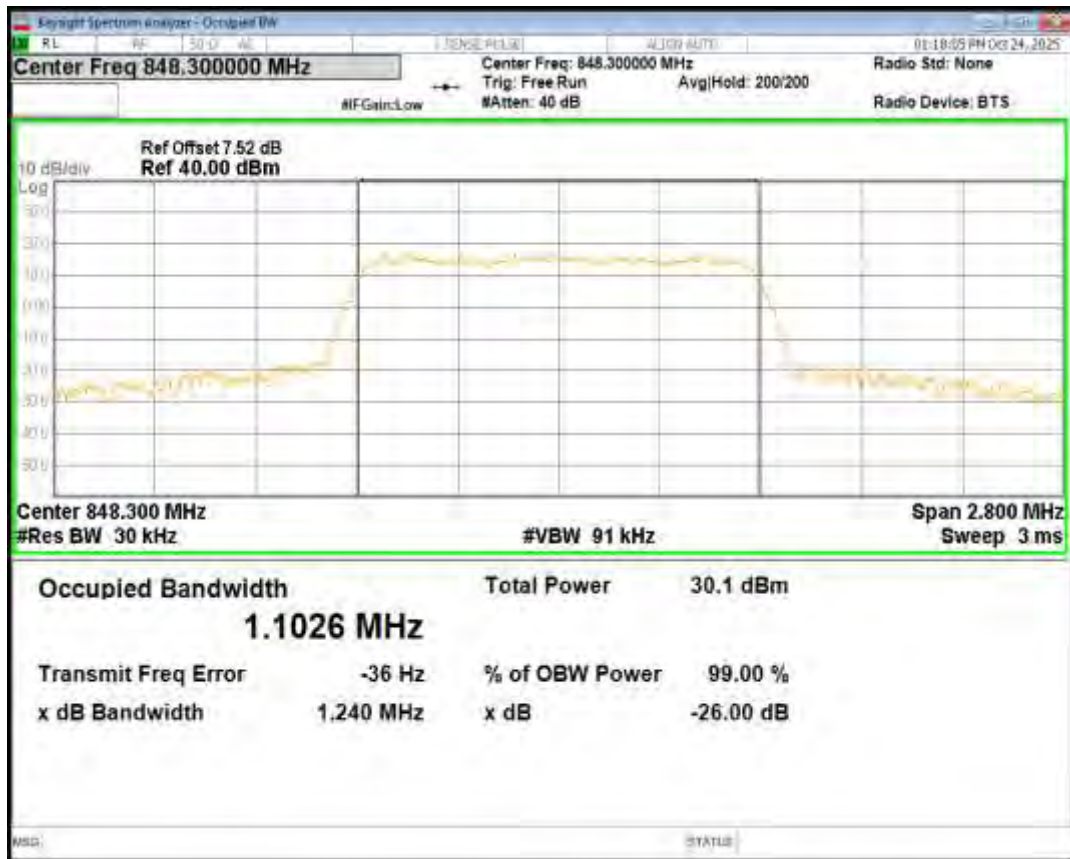
Band5 16QAM BW=10MHz Channel=20450 RB Size=50 Position=#0
