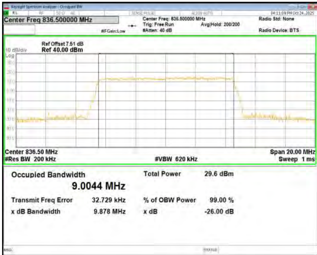
Band26(824-849) 16QAM BW=10MHz Channel=26990 RB Size=50 Position=#0
