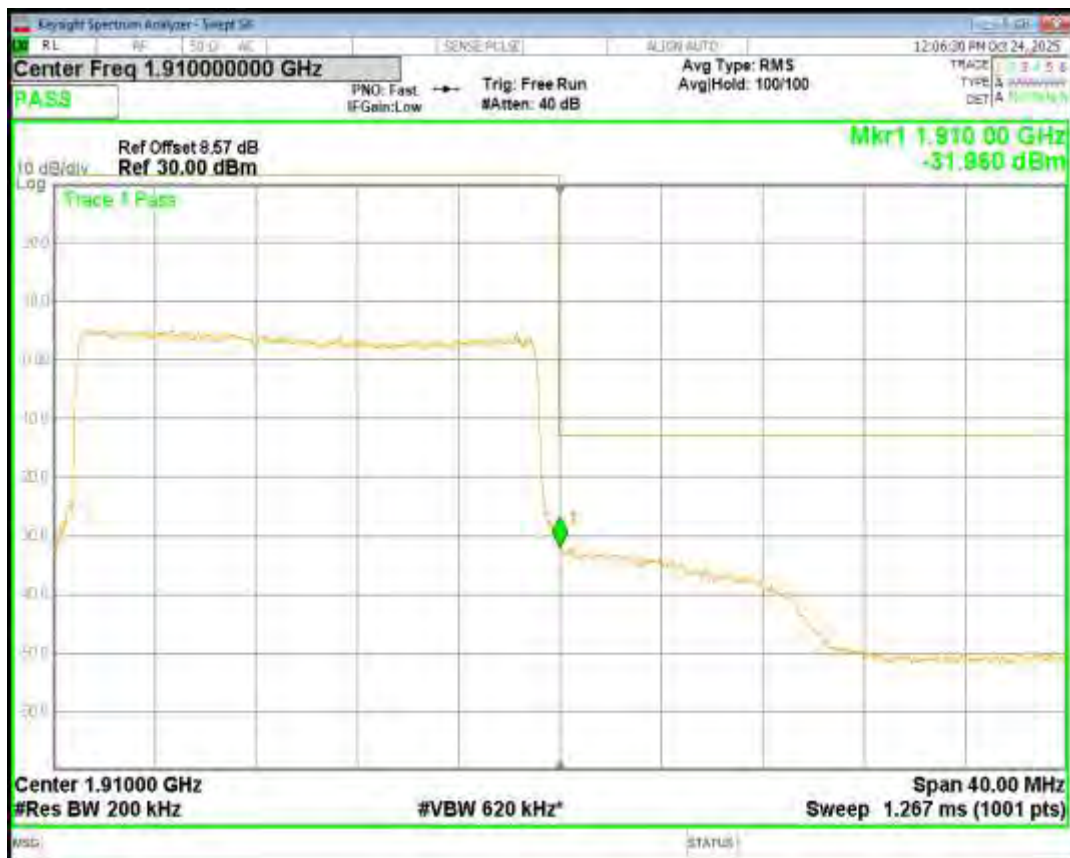
Band2 QPSK BW=3MHz Channel=18615 RB Size=15 Position=#0
