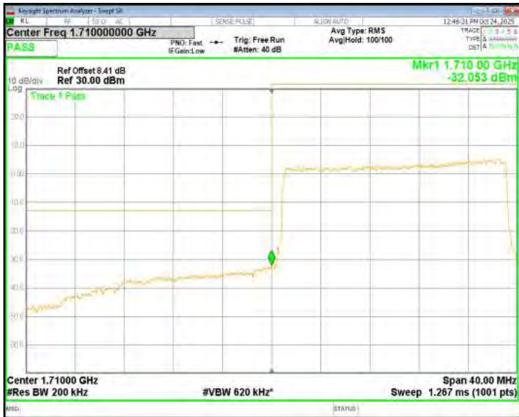
Band4 QPSK BW=20MHz Channel=20300 RB Size=100 Position=#0
