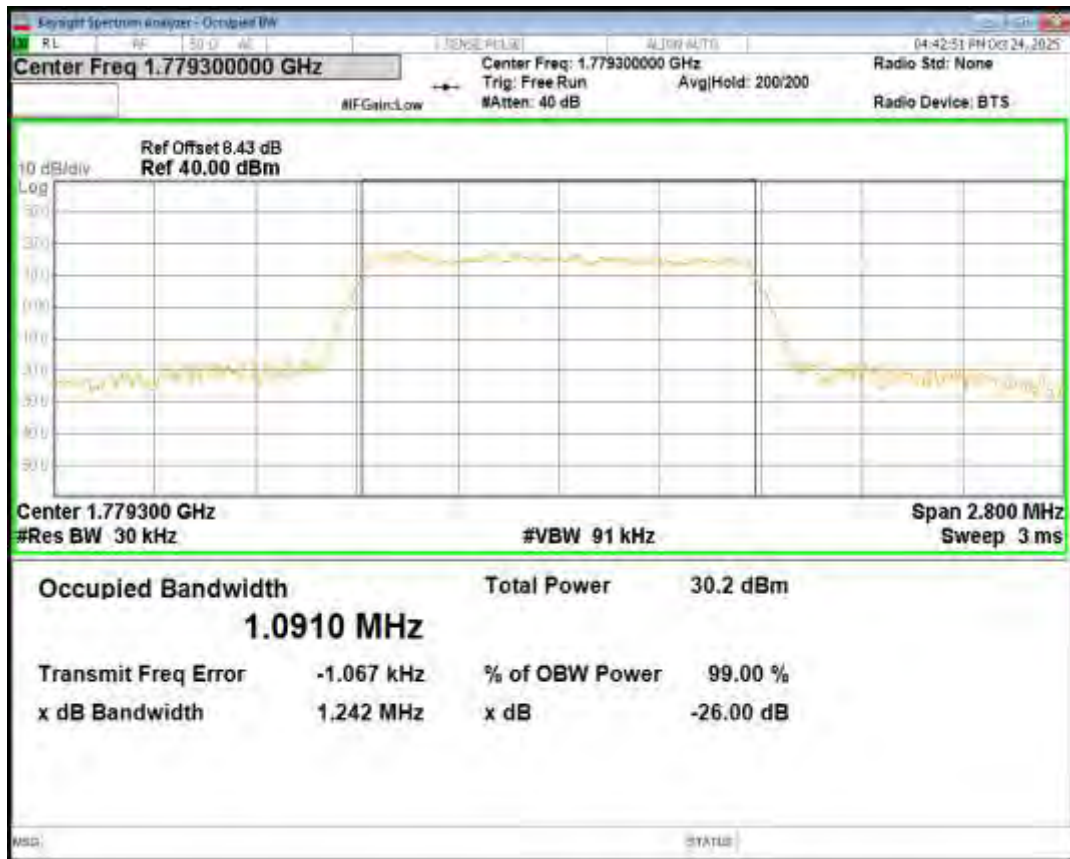
Band66 16QAM BW=10MHz Channel=132022 RB Size=50 Position=#0
