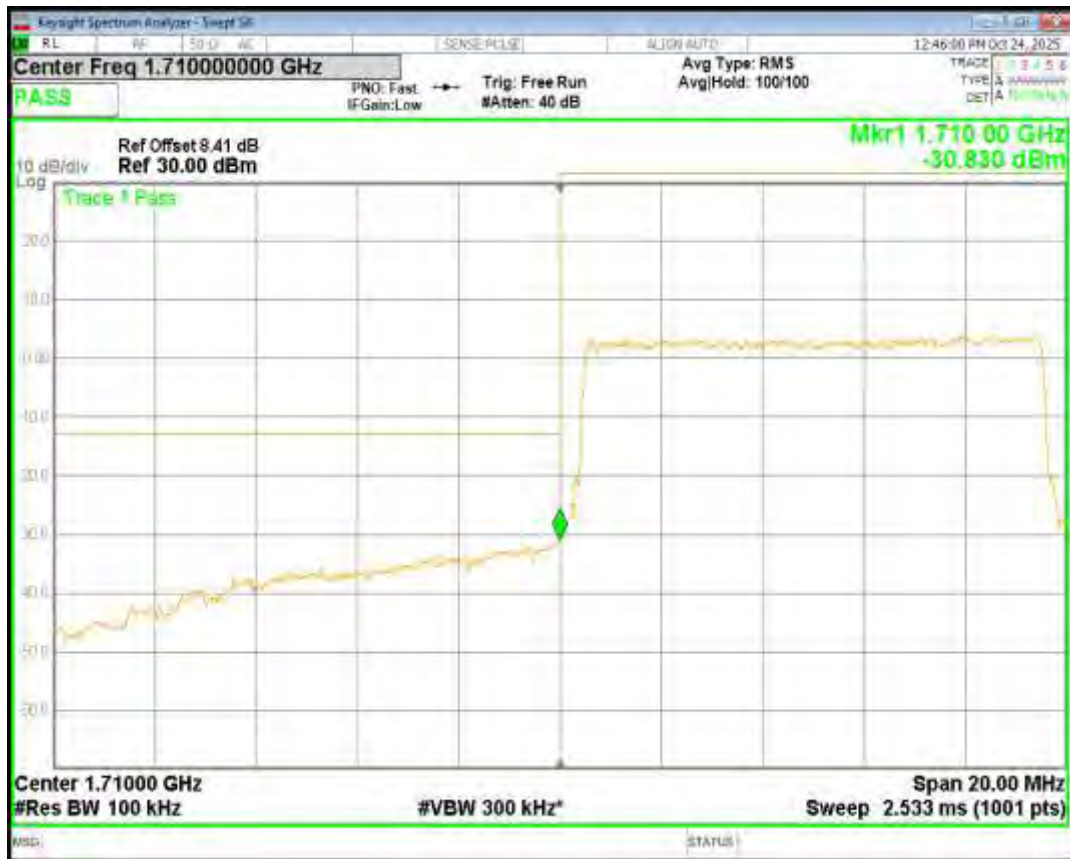
Band4 QPSK BW=10MHz Channel=20350 RB Size=50 Position=#0
