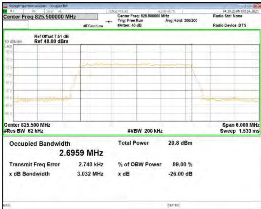
Band26(824-849) 16QAM BW=3MHz Channel=26915 RB Size=15 Position=#0
