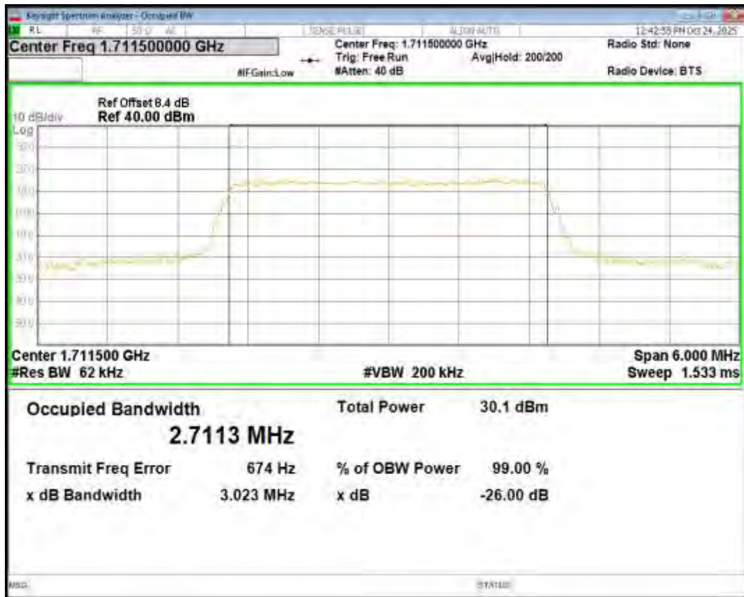
Band4 16QAM BW=3MHz Channel=20175 RB Size=15 Position=#0
