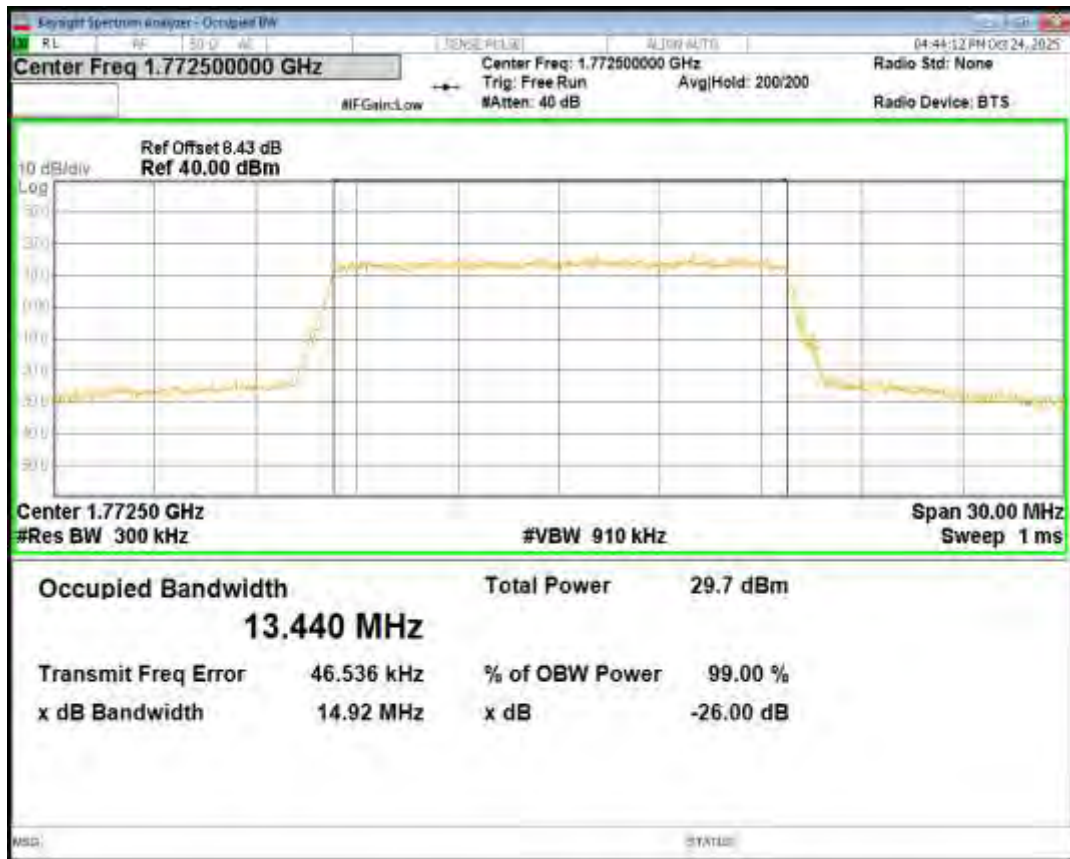
Band66 16QAM BW=20MHz Channel=132072 RB Size=100 Position=#0
