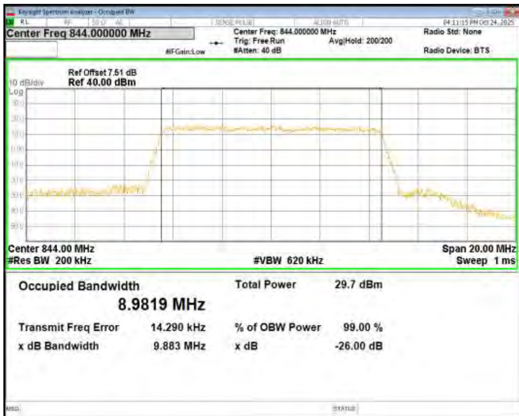
Band26(824-849) 16QAM BW=15MHz Channel=26865 RB Size=75 Position=#0
