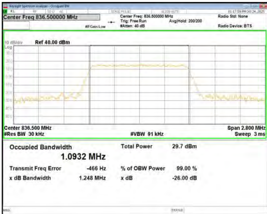
Band5 16QAM BW=1.4MHz Channel=20643 RB Size=6 Position=#0
