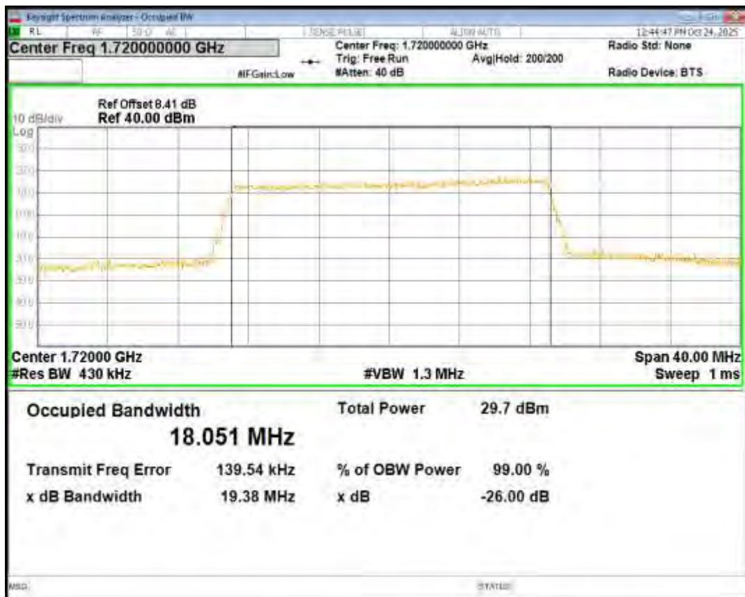
Band4 16QAM BW=20MHz Channel=20175 RB Size=100 Position=#0
