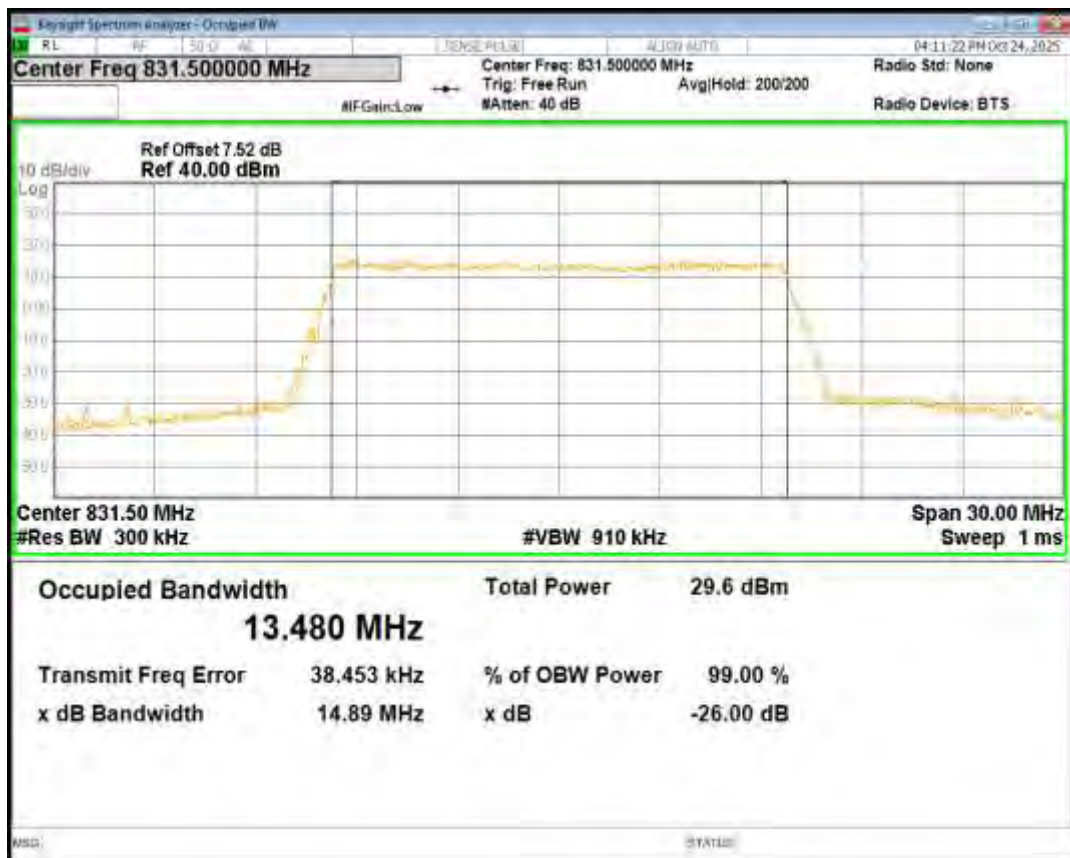
Band26(824-849) QPSK BW=15MHz Channel=26915 RB Size=75 Position=#0
