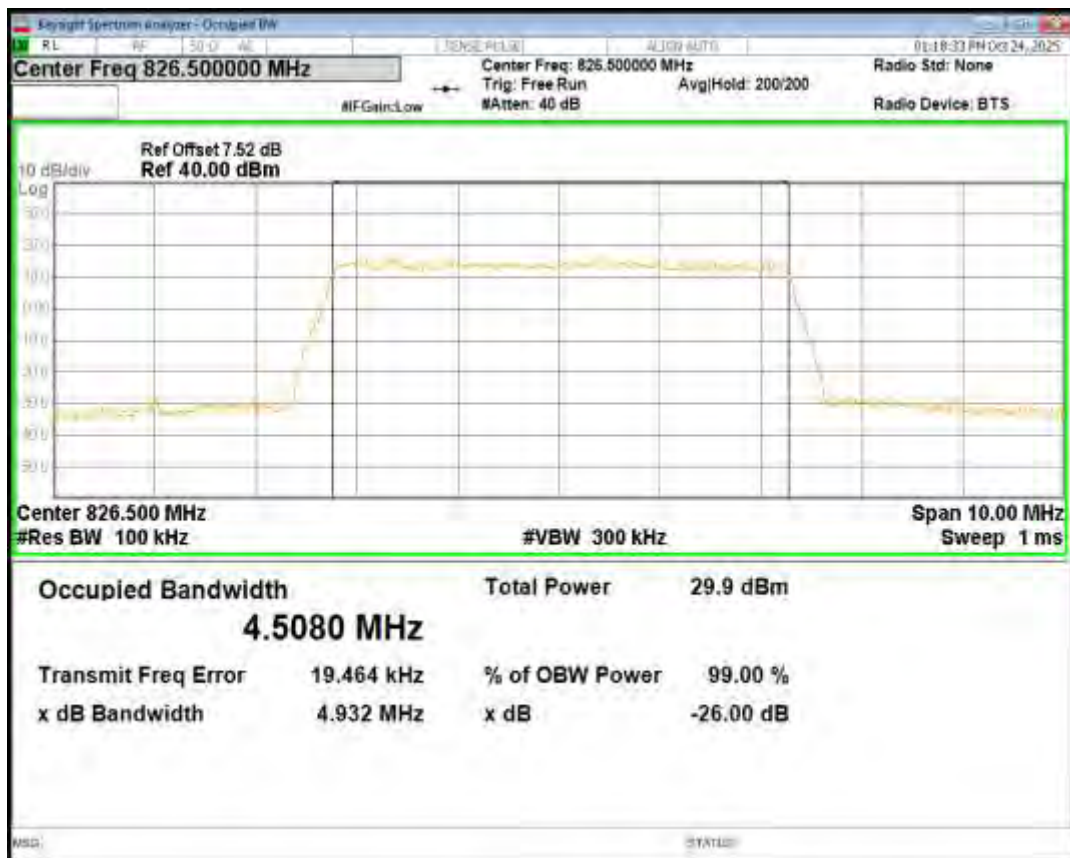
Band5 16QAM BW=5MHz Channel=20525 RB Size=25 Position=#0
