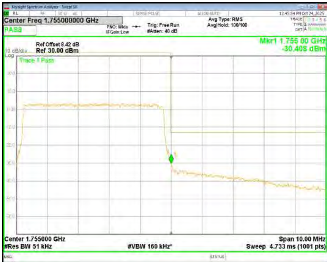
Band4 QPSK BW=1.4MHz Channel=19957 RB Size=6 Position=#0
