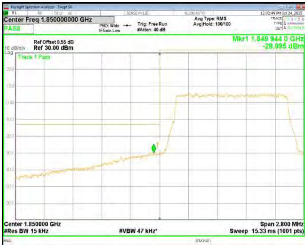
Band2 16QAM BW=5MHz Channel=19175 RB Size=25 Position=#0
