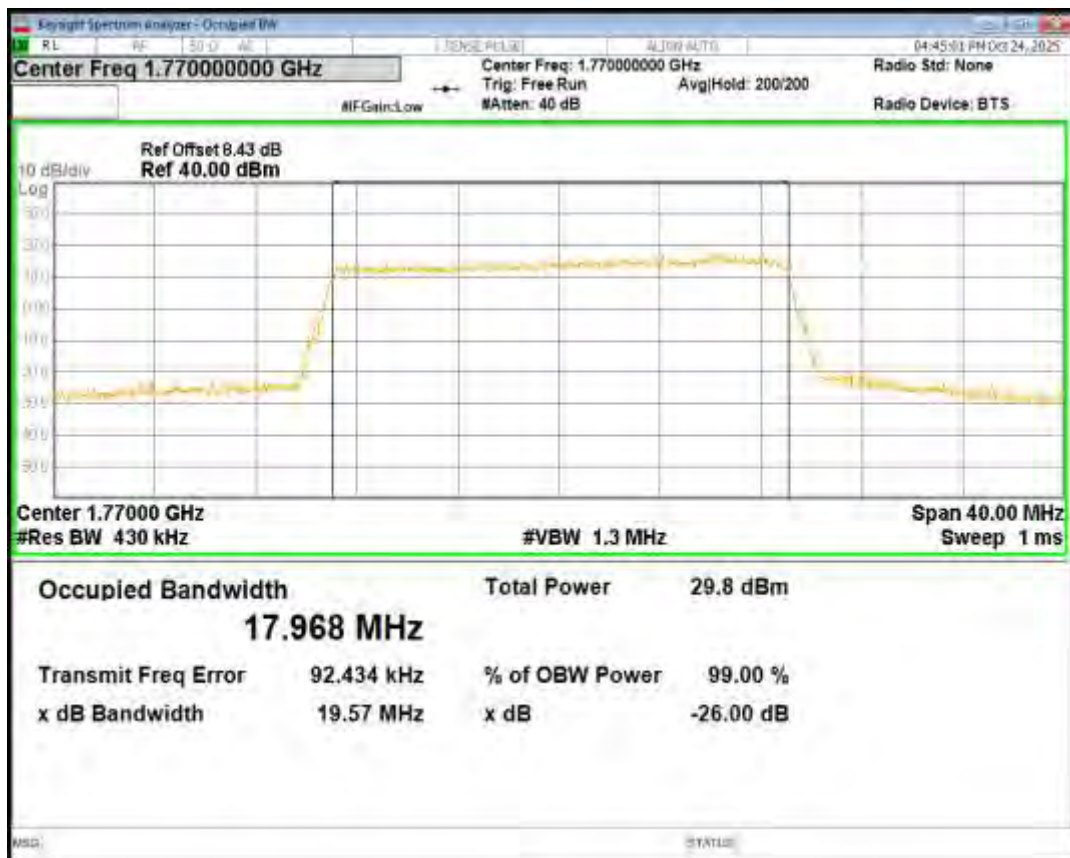
Band66 16QAM BW=3MHz Channel=131987 RB Size=15 Position=#0
