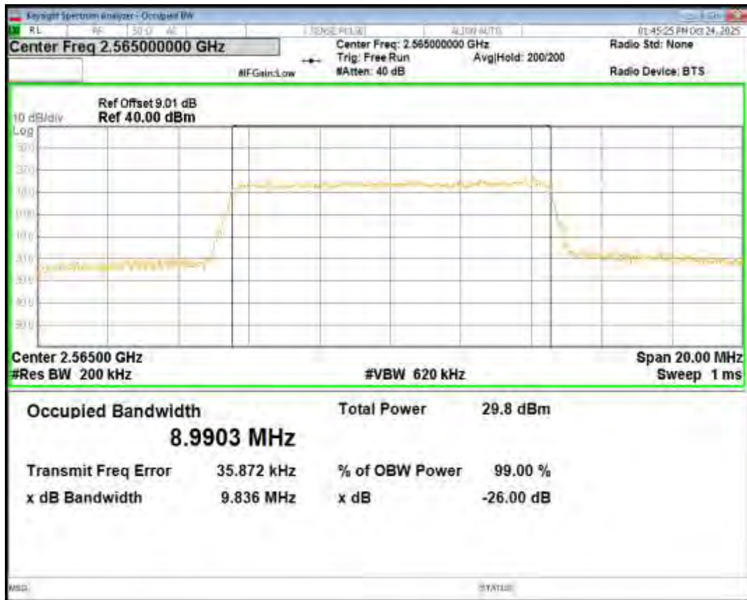
Band7 QPSK BW=15MHz Channel=20825 RB Size=75 Position=#0
