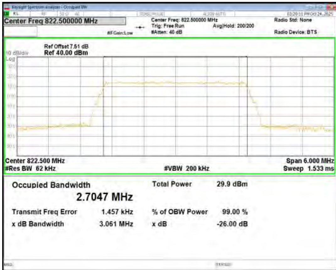
Band26(814-824) 16QAM BW=5MHz Channel=26715 RB Size=25 Position=#0
