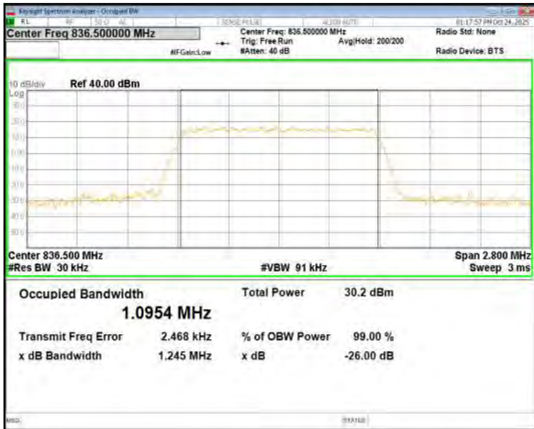
Band5 16QAM BW=5MHz Channel=20625 RB Size=25 Position=#0
