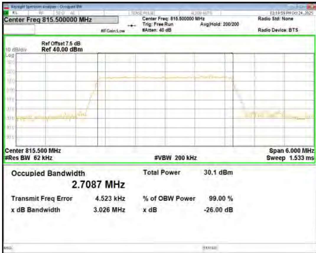
Band26(814-824) 16QAM BW=3MHz Channel=26740 RB Size=15 Position=#0
