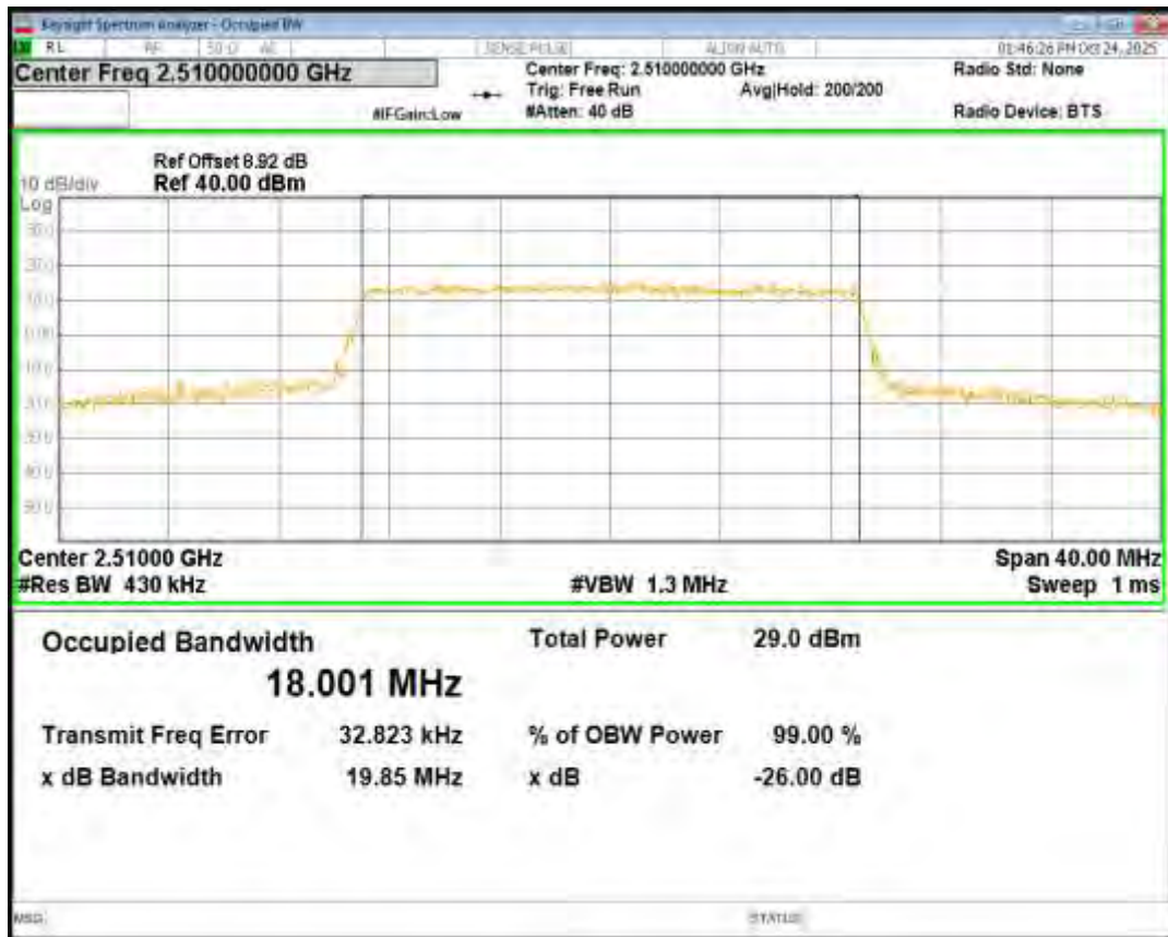
Band7 16QAM BW=20MHz Channel=21100 RB Size=100 Position=#0
