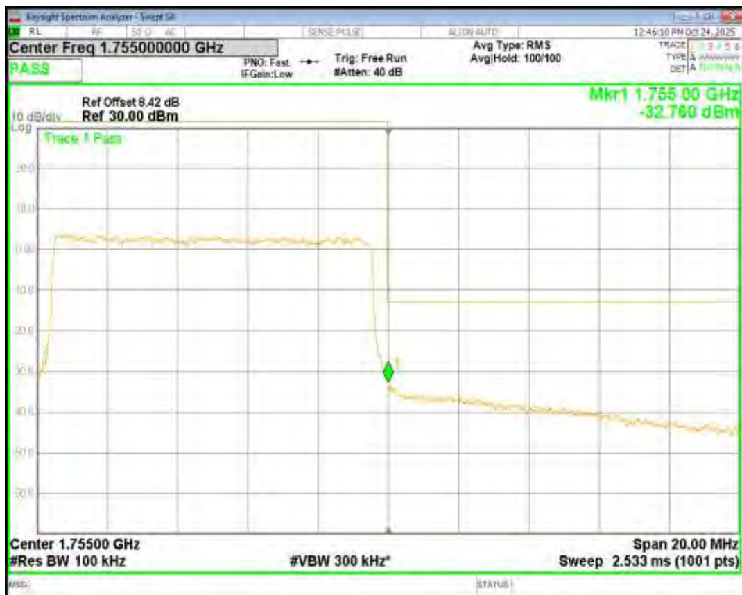
Band4 16QAM BW=15MHz Channel=20025 RB Size=75 Position=#0
