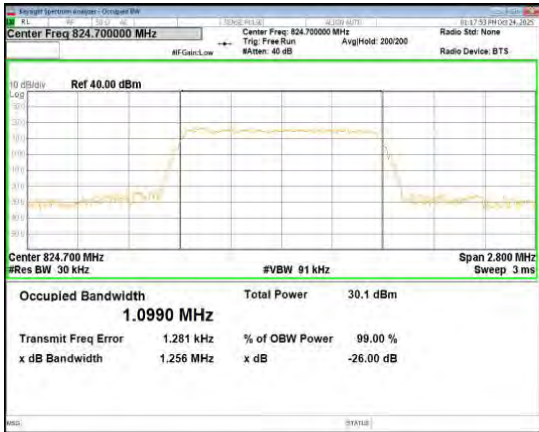
Band5 16QAM BW=1.4MHz Channel=20525 RB Size=6 Position=#0
