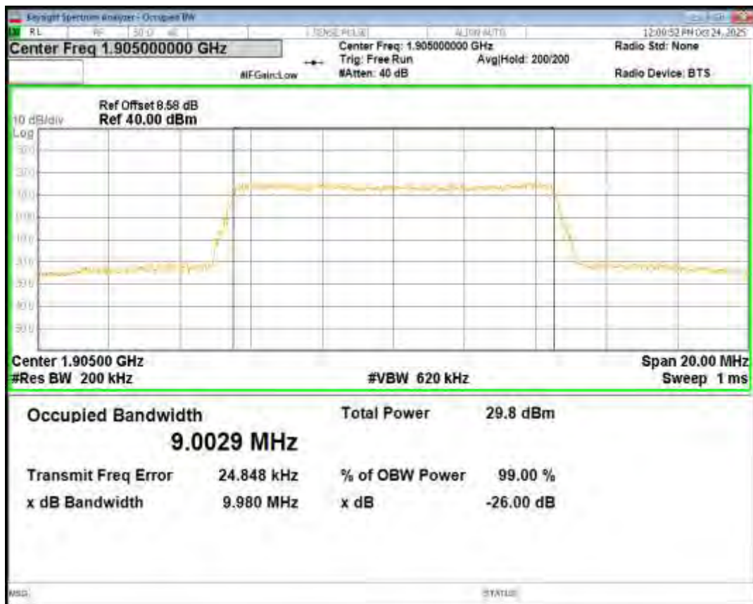
Band2 16QAM BW=15MHz Channel=18675 RB Size=75 Position=#0
