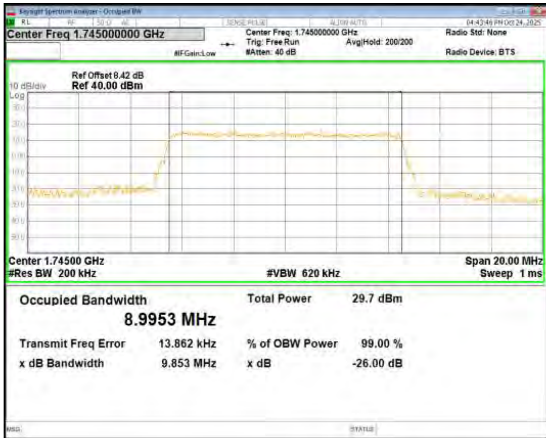
Band66 16QAM BW=10MHz Channel=132622 RB Size=50 Position=#0
