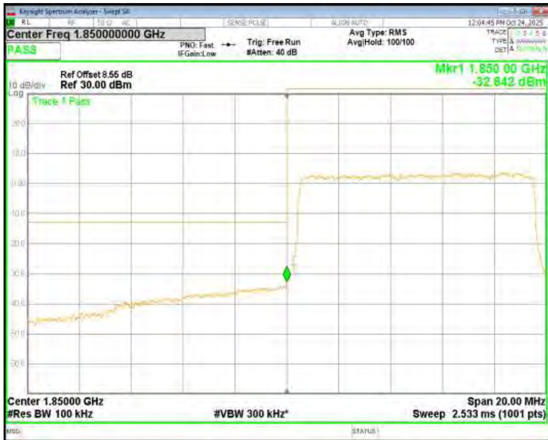
Band2 16QAM BW=10MHz Channel=19150 RB Size=50 Position=#0
