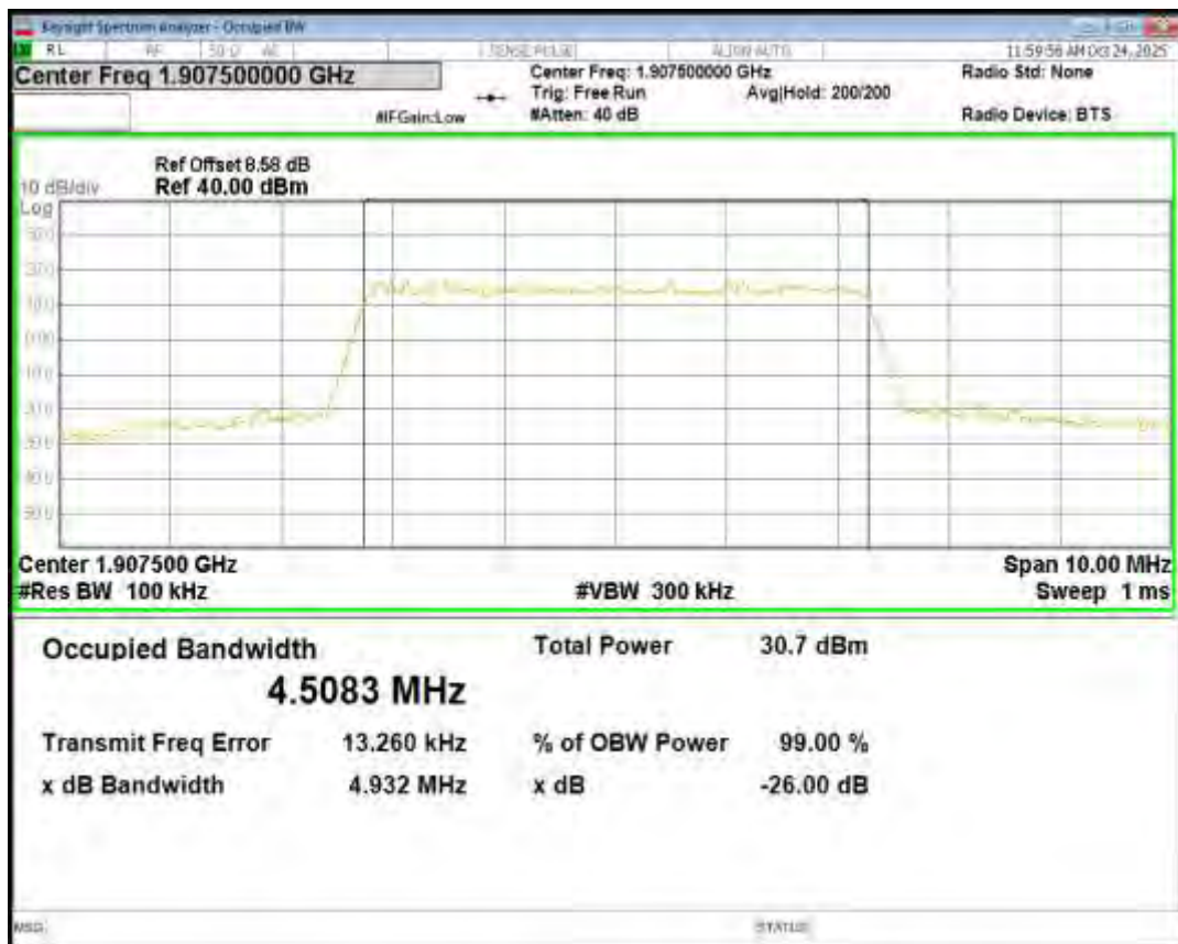
Band26(814-824) 16QAM BW=1.4MHz Channel=26697 RB Size=6 Position=#0
