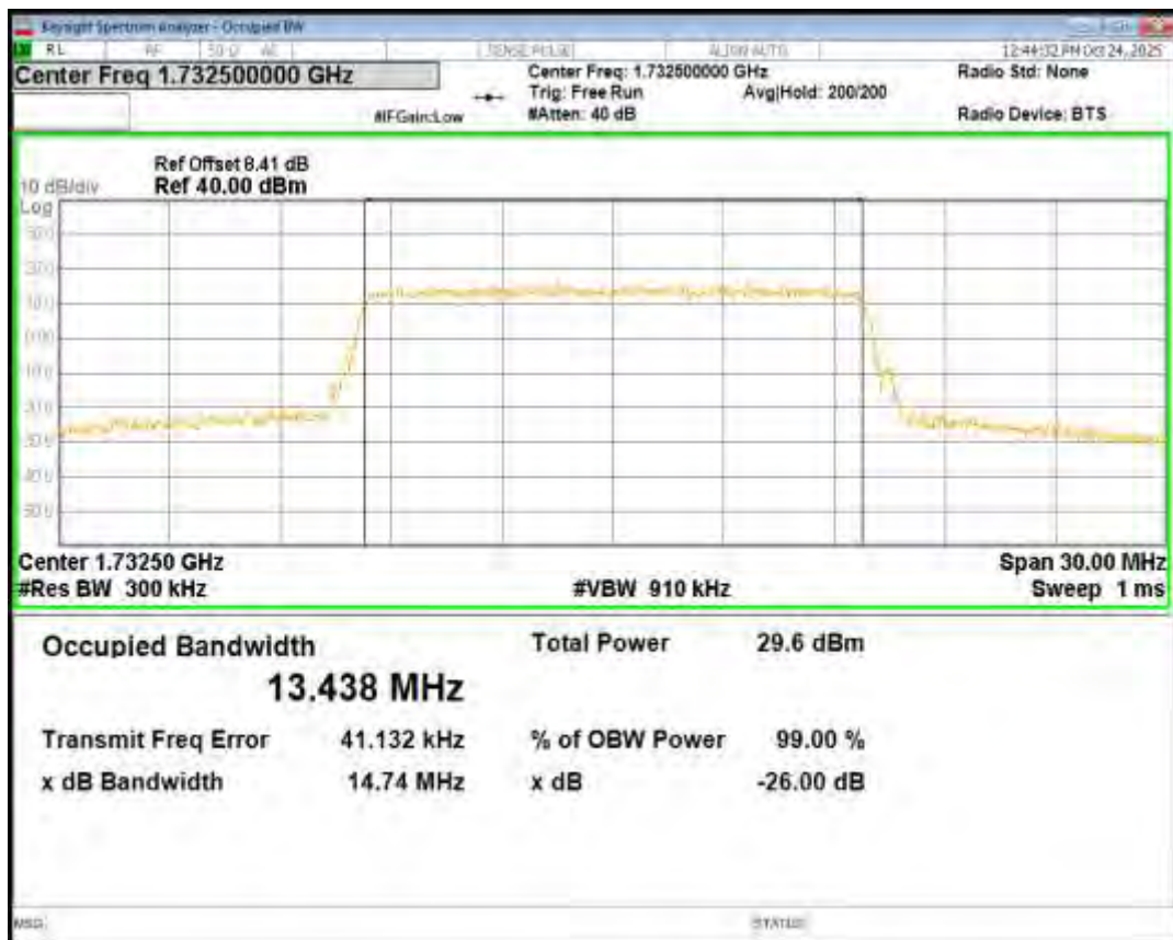
Band4 16QAM BW=15MHz Channel=20325 RB Size=75 Position=#0
