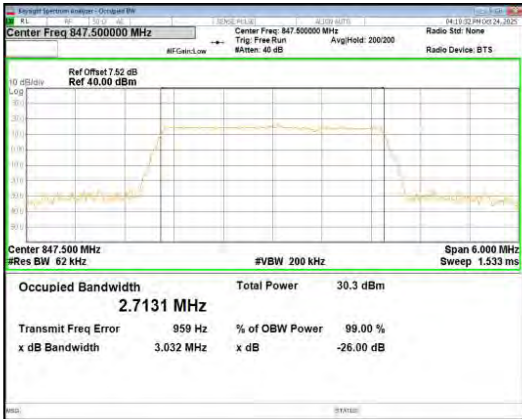
Band26(824-849) QPSK BW=5MHz Channel=26815 RB Size=25 Position=#0
