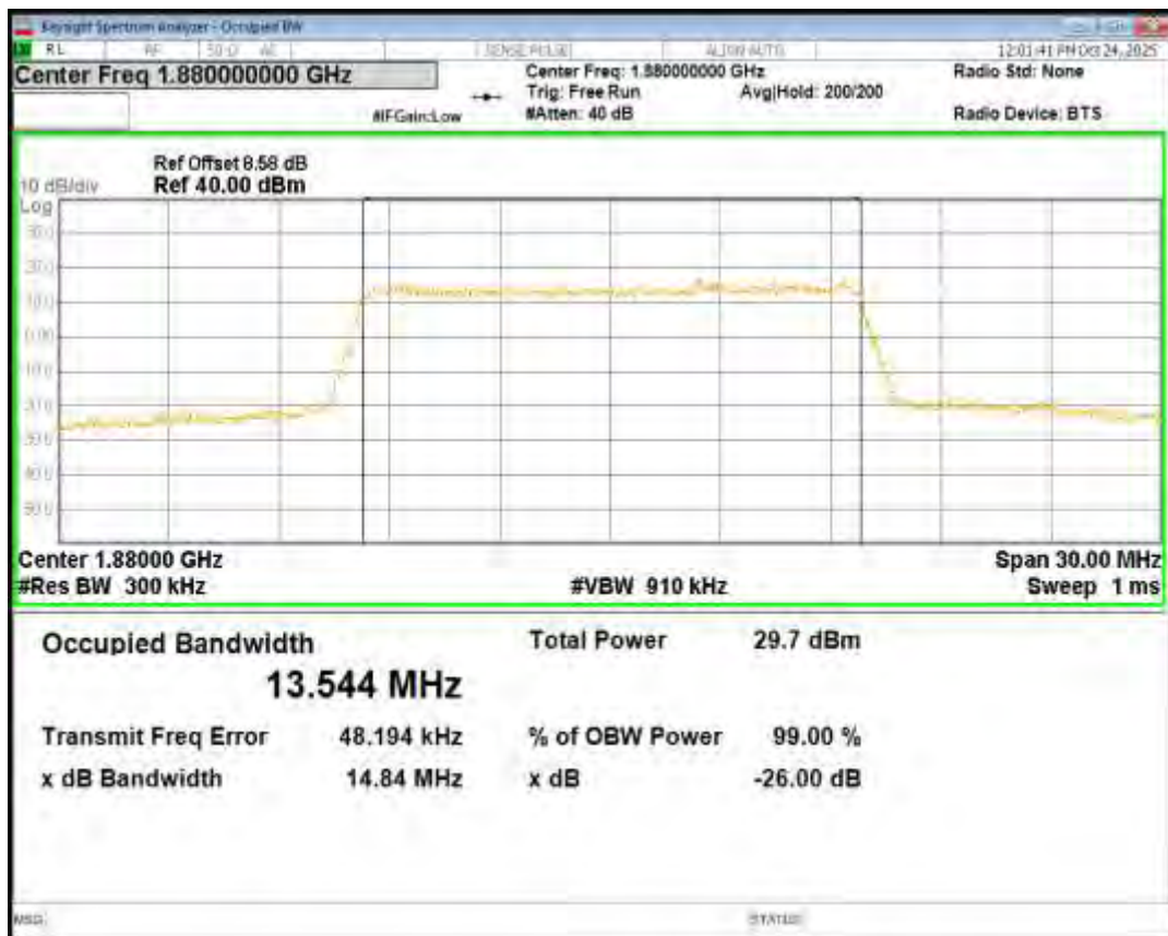
Band2 16QAM BW=15MHz Channel=19125 RB Size=75 Position=#0
