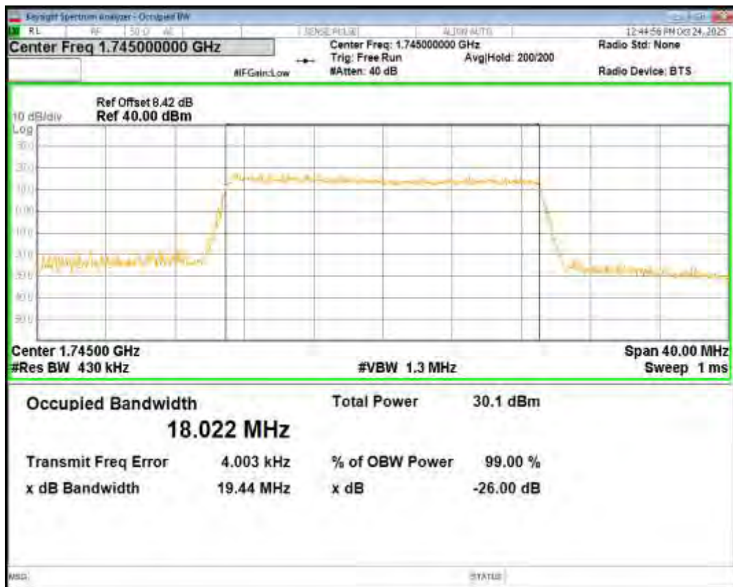
Band4 QPSK BW=15MHz Channel=20325 RB Size=75 Position=#0
