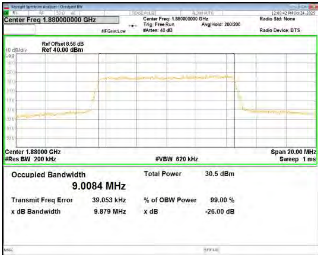
Band2 QPSK BW=10MHz Channel=19150 RB Size=50 Position=#0
