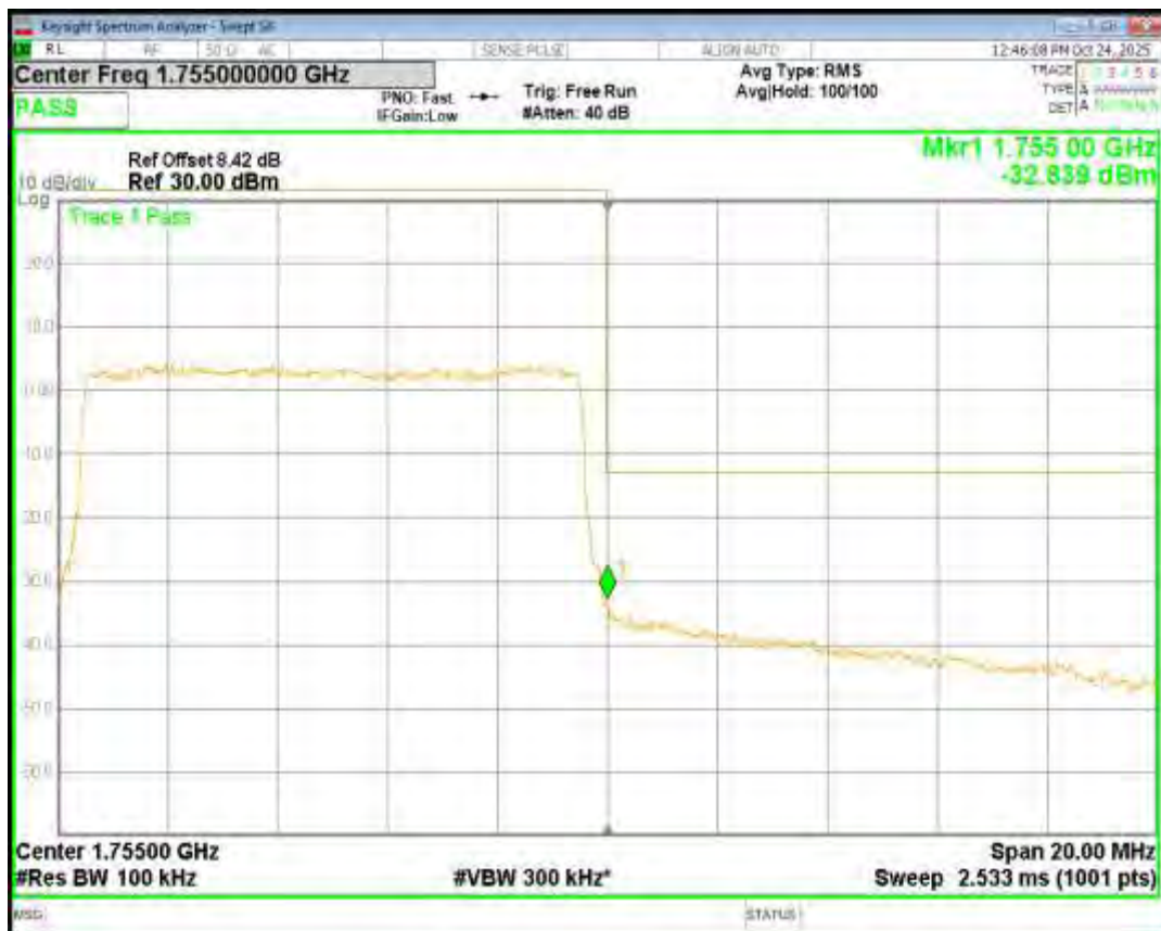
Band4 QPSK BW=15MHz Channel=20025 RB Size=75 Position=#0
