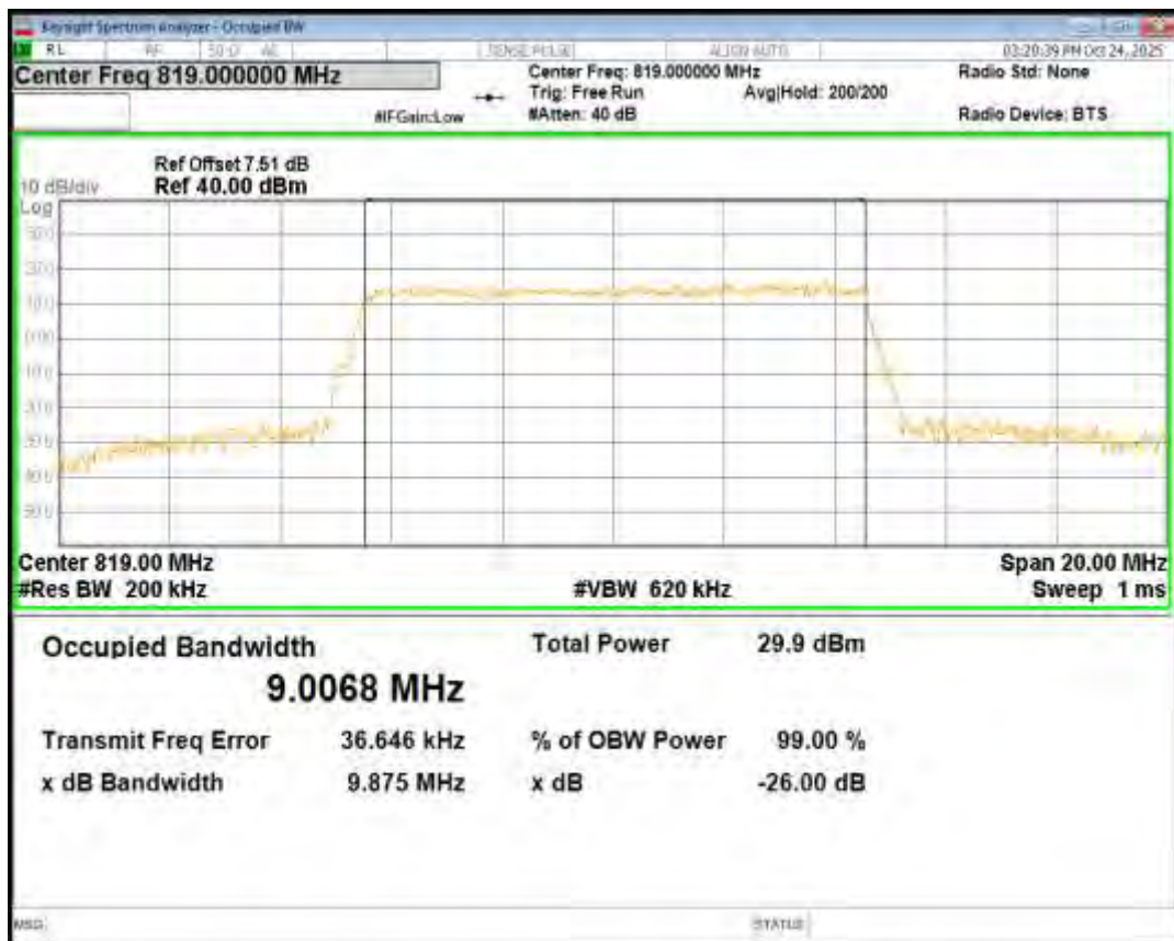
Band26(814-824) 16QAM BW=3MHz Channel=26705 RB Size=15 Position=#0
