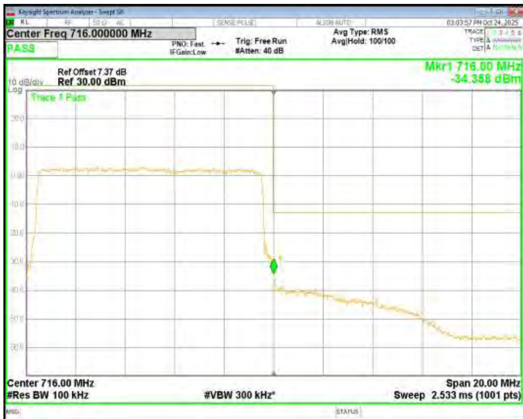
Band17 16QAM BW=5MHz Channel=23755 RB Size=25 Position=#0
