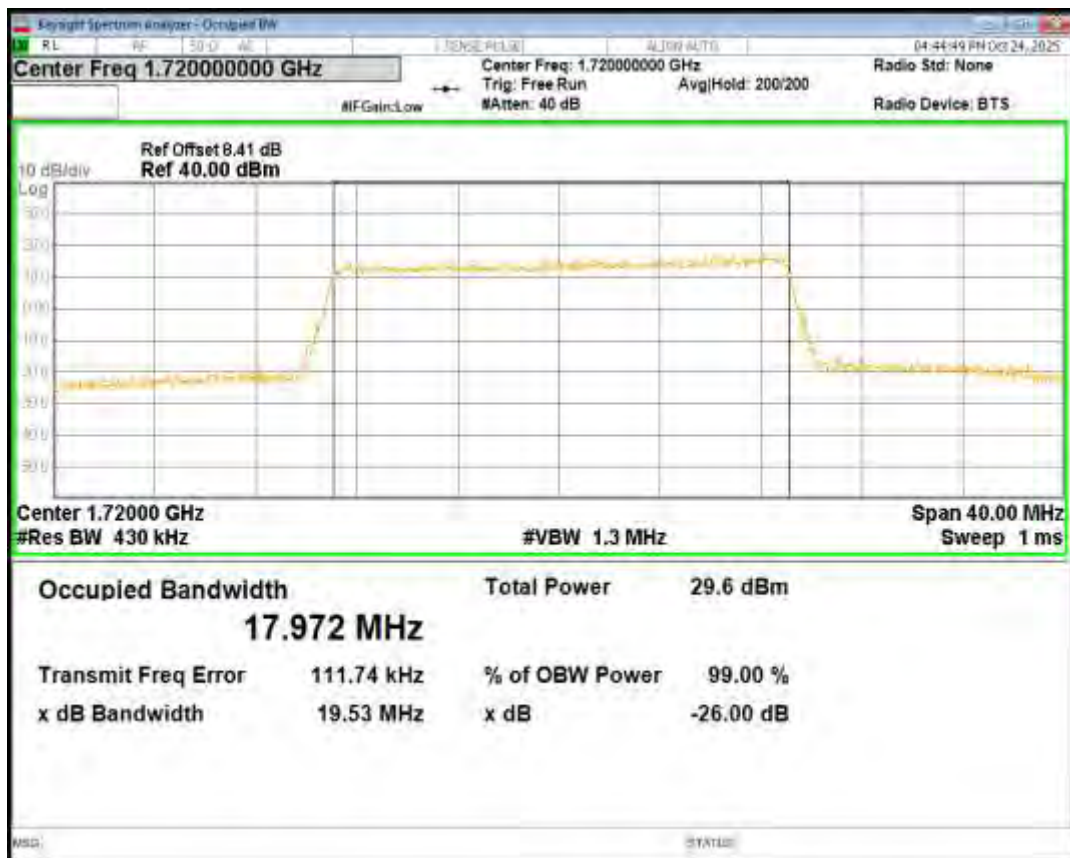
Band66 16QAM BW=20MHz Channel=132322 RB Size=100 Position=#0
