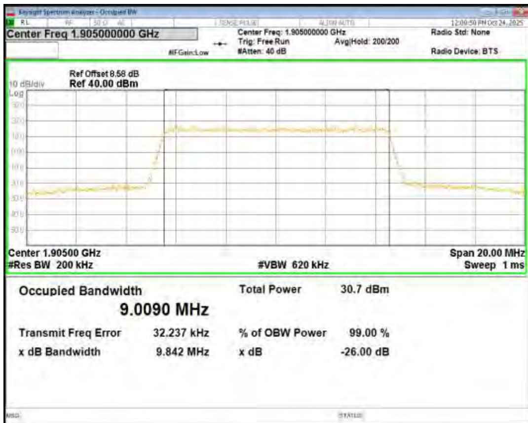
Band2 QPSK BW=15MHz Channel=18675 RB Size=75 Position=#0
