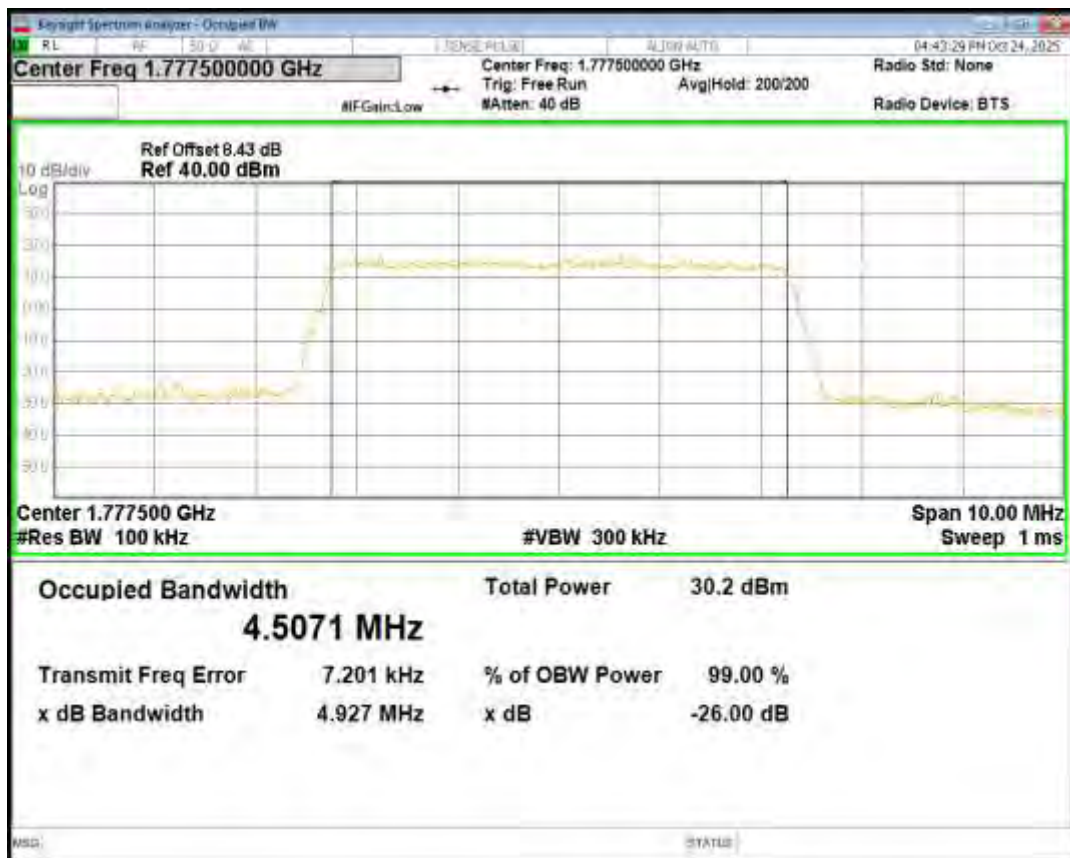
Band7 16QAM BW=10MHz Channel=20800 RB Size=50 Position=#0
