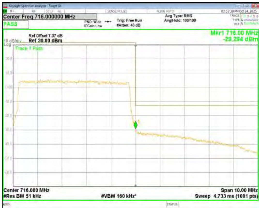
Band2 16QAM BW=1.4MHz Channel=18607 RB Size=6 Position=#0
