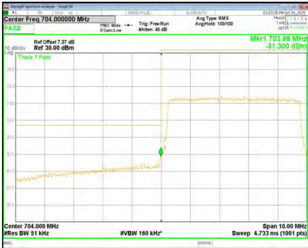
Band17 16QAM BW=5MHz Channel=23825 RB Size=25 Position=#0
