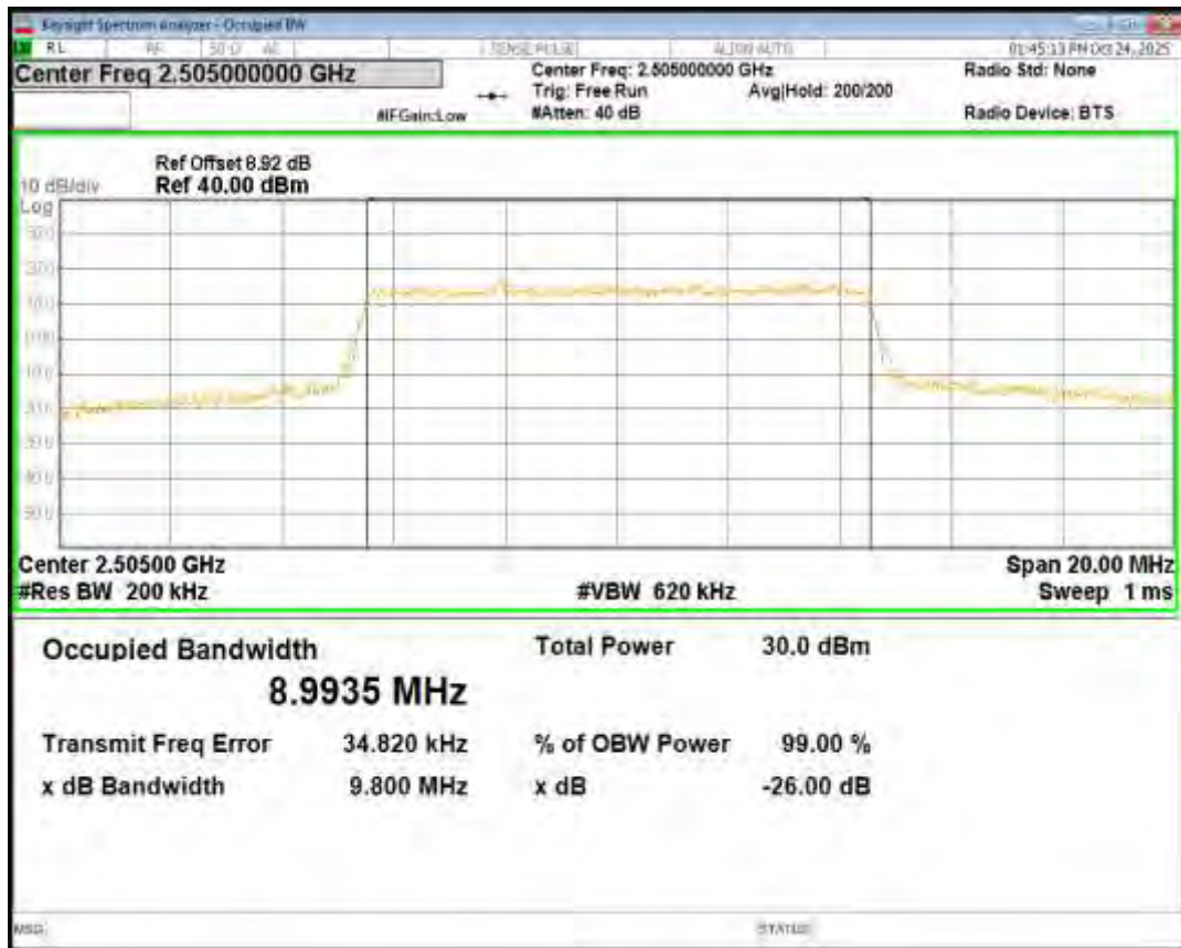
Band7 QPSK BW=10MHz Channel=21100 RB Size=50 Position=#0
