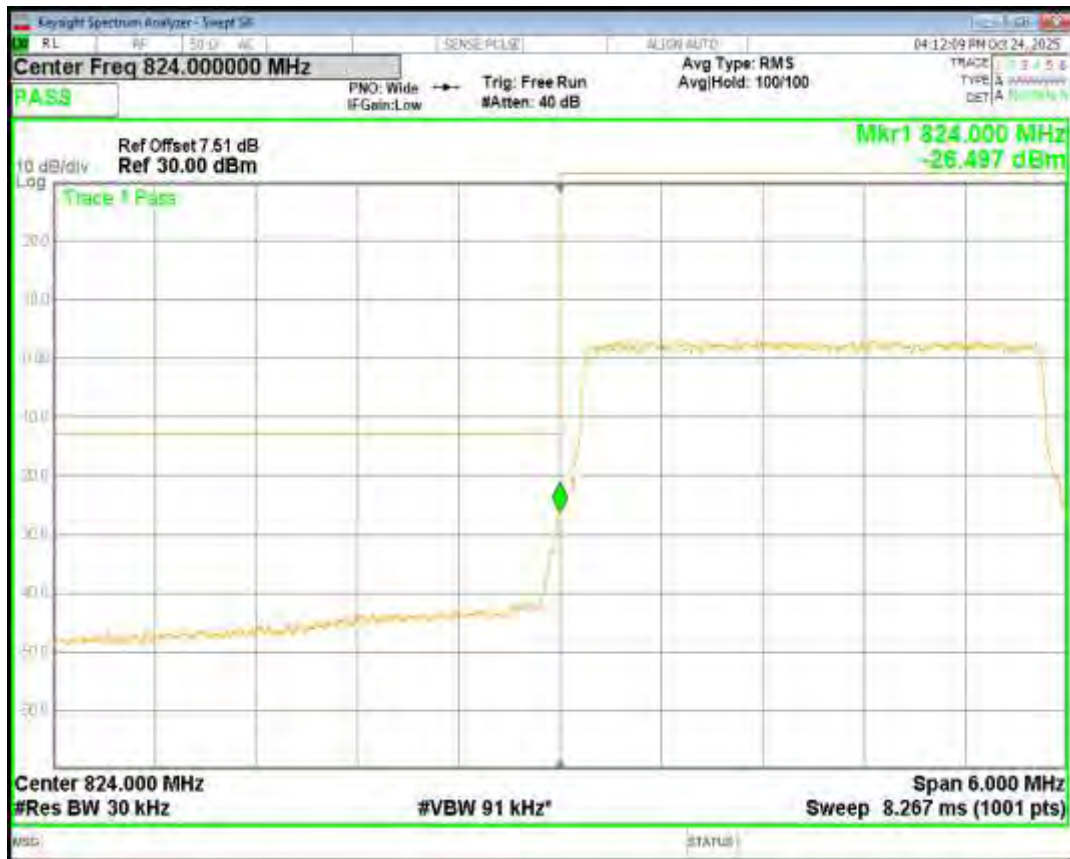
Band26(824-849) 16QAM BW=5MHz Channel=26815 RB Size=25 Position=#0
