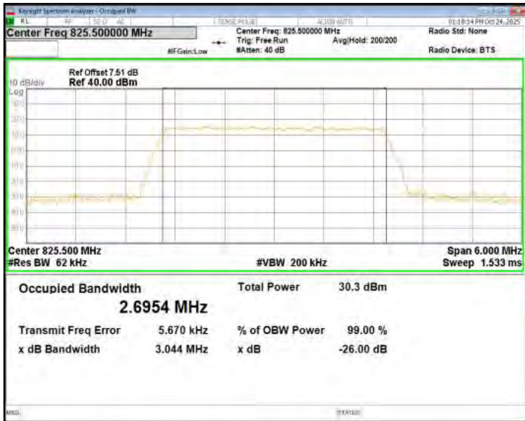
Band5 16QAM BW=3MHz Channel=20525 RB Size=15 Position=#0
