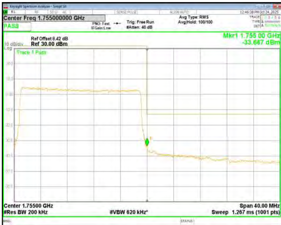
Band4 QPSK BW=3MHz Channel=19965 RB Size=15 Position=#0
