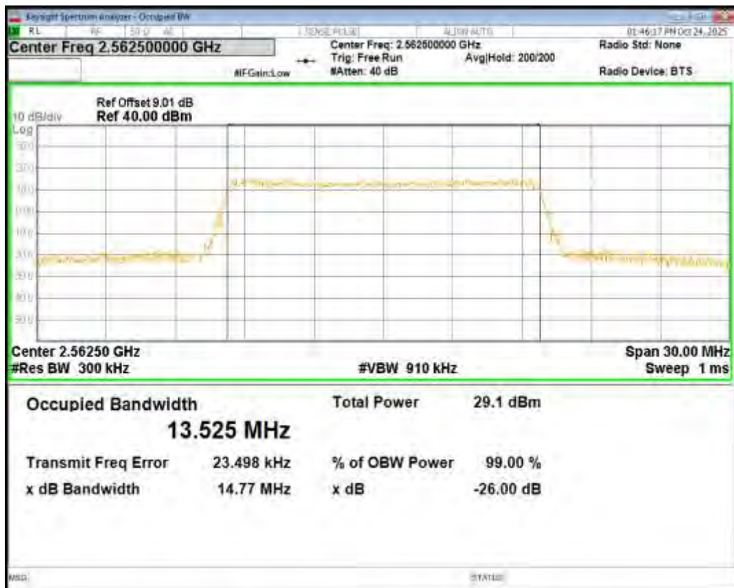
Band7 16QAM BW=20MHz Channel=20850 RB Size=100 Position=#0
