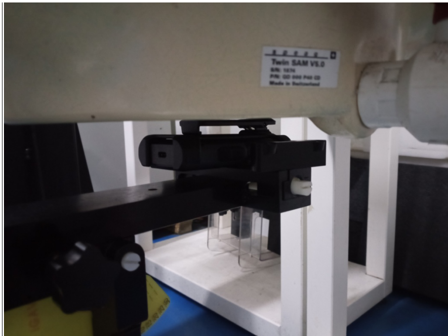
Body Back With Belt Clip Setup Photo(0mm)
