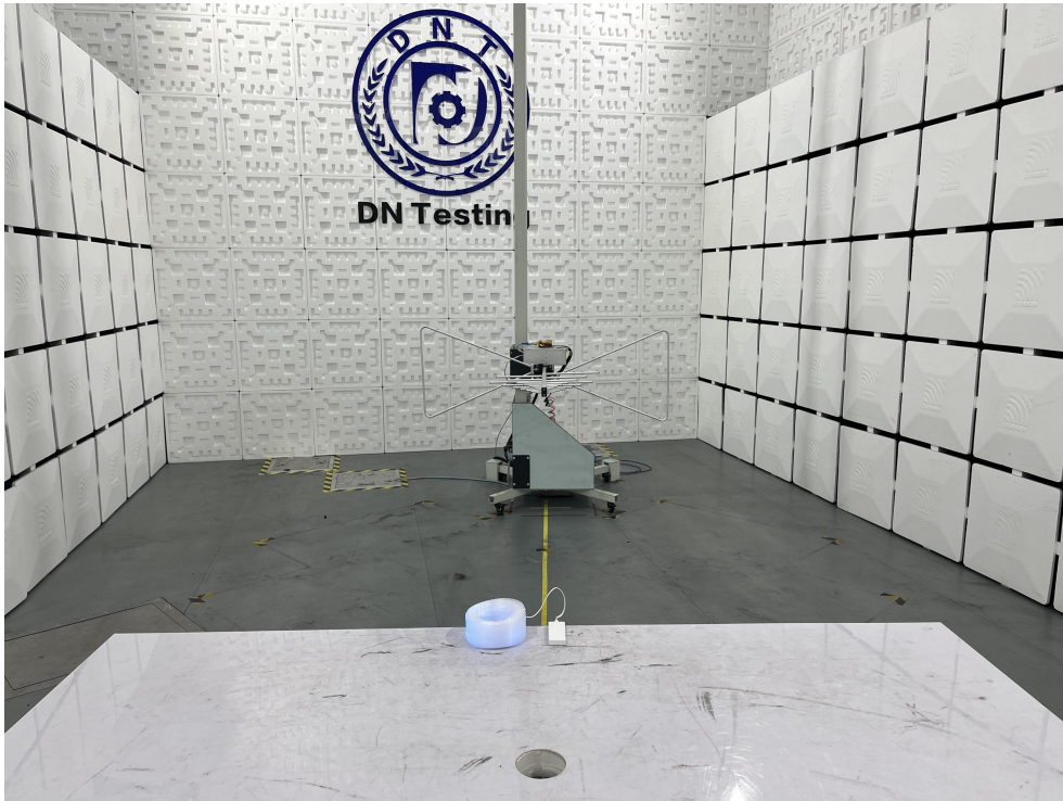
Radiated Emission Test View[(Below 1G)
