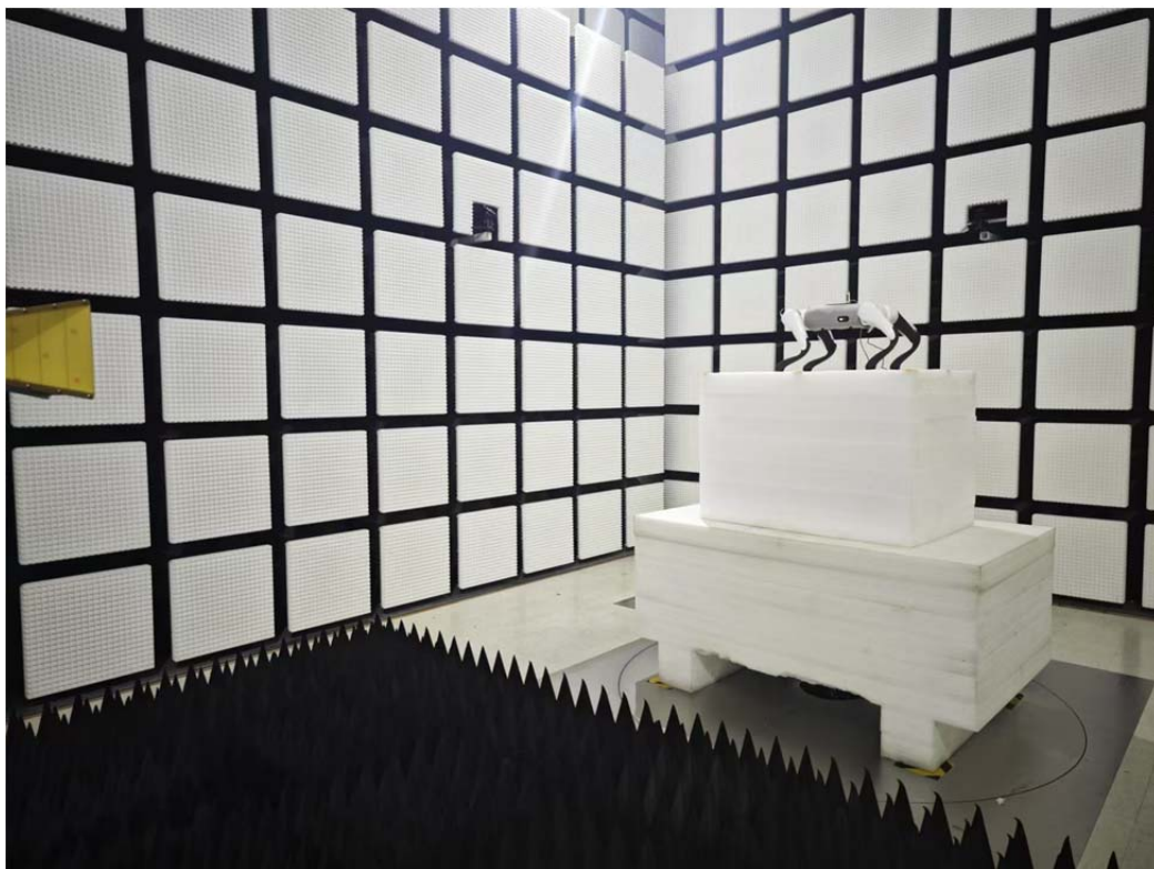
Radiated Emission Above 1-18GHz View
