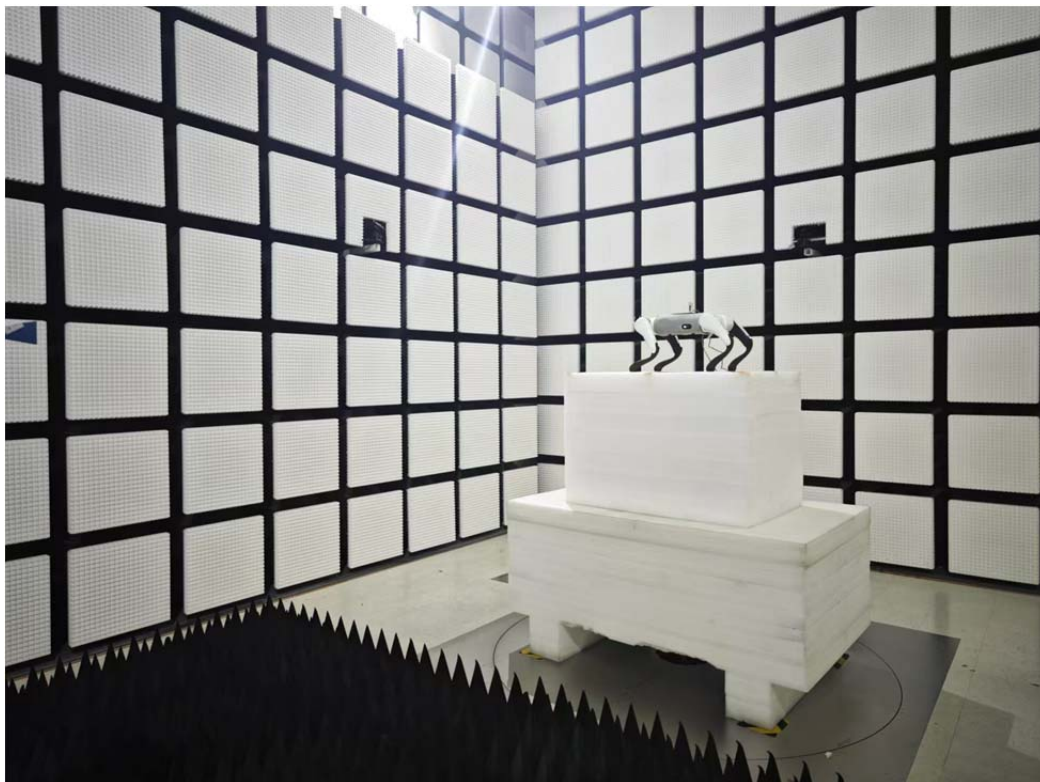
Radiated Emission Above 18-25GHz View
