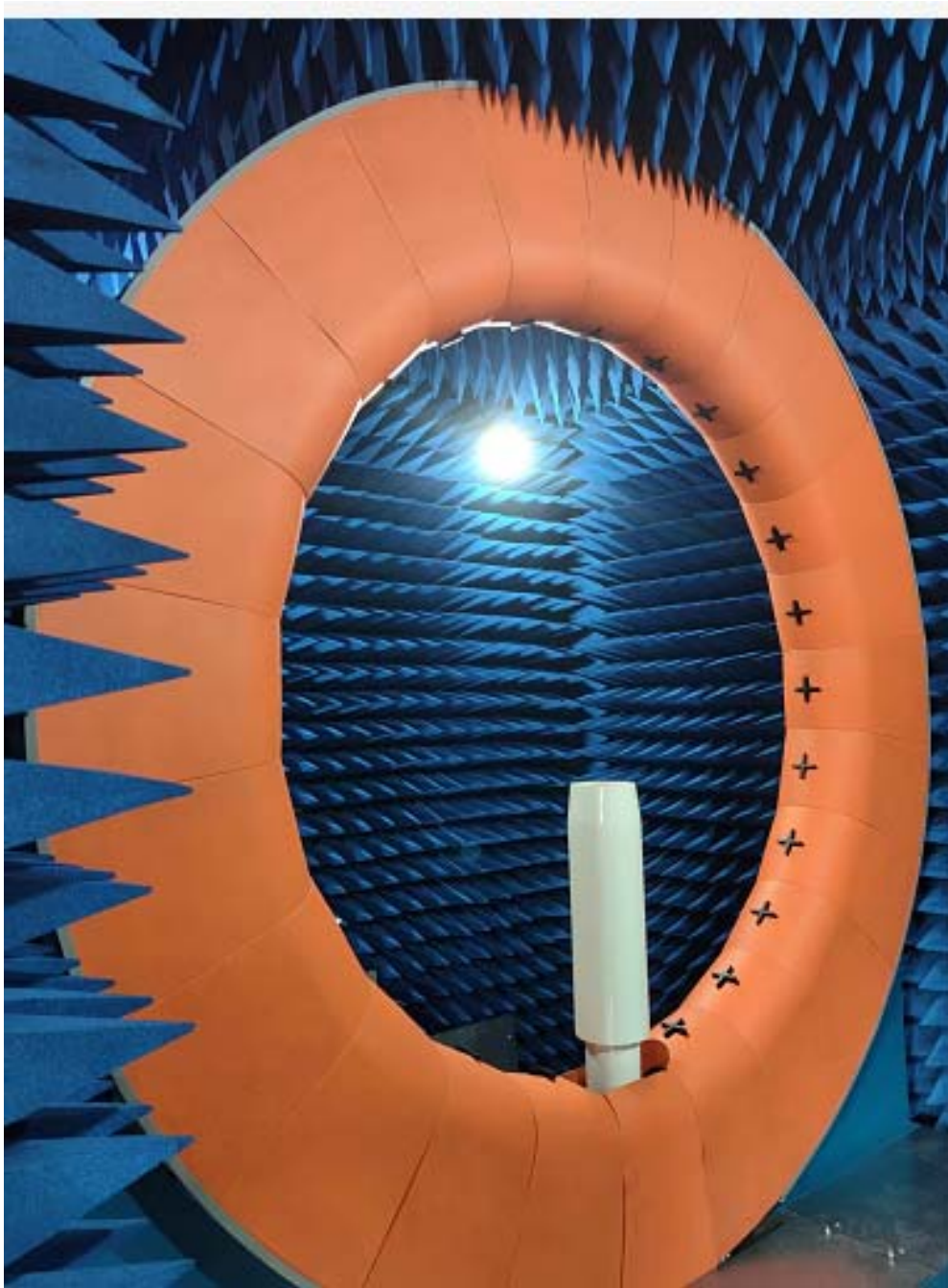
24 probe microwave darkroom testing equipment
