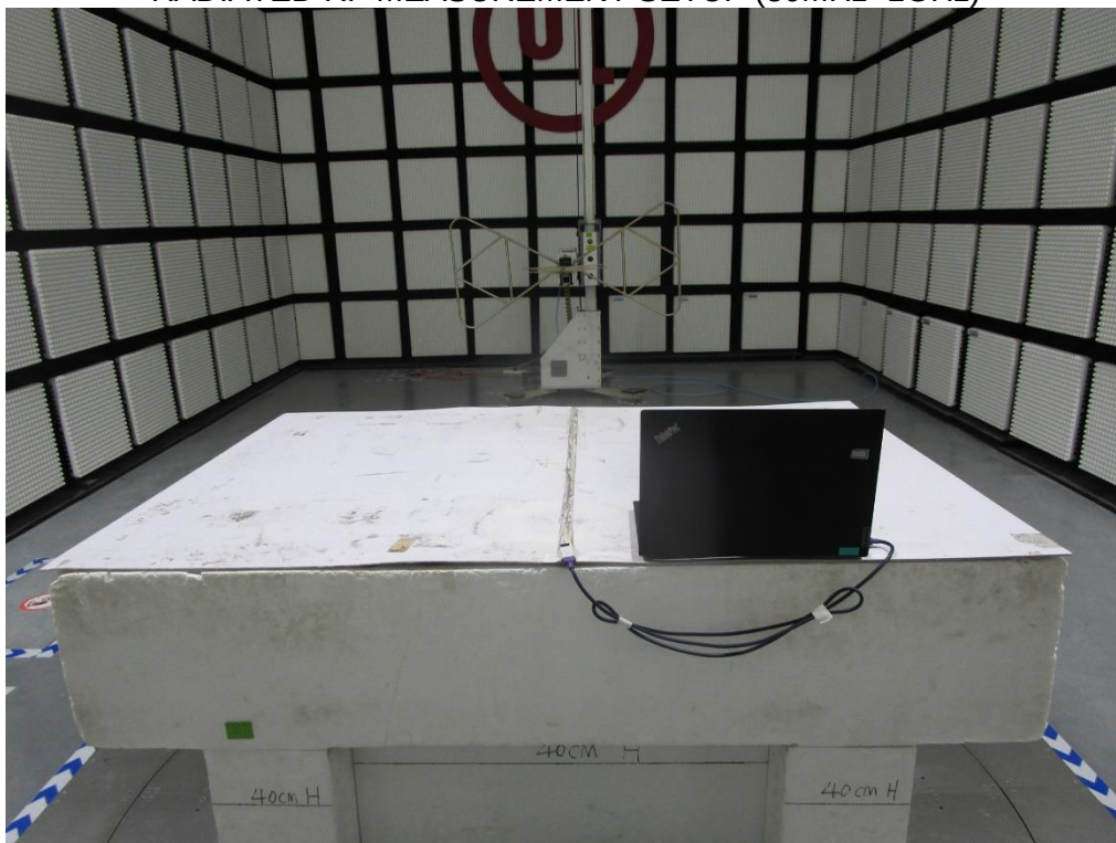
RADIATED RF MEASUREMENT SETUP (Below 30MHz)
