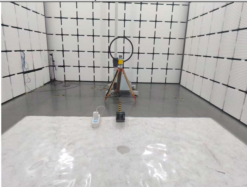
Radiated Spurious Emission, 9KHz~30MHz
