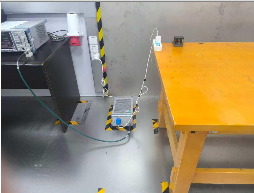
Radiated Spurious Emission, 9KHz~30MHz
