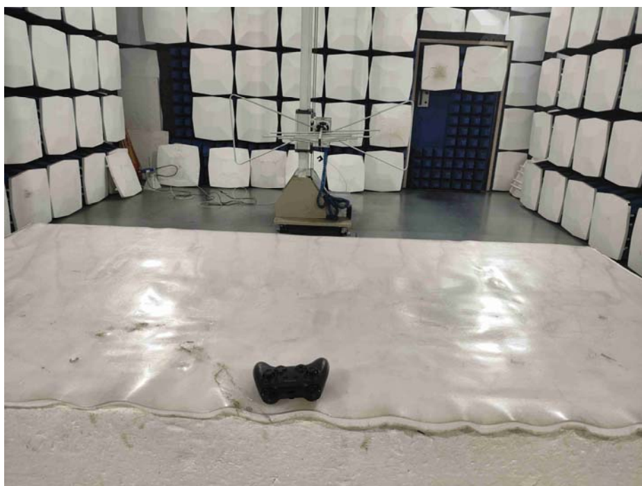
Radiated Emission Test Setup:
