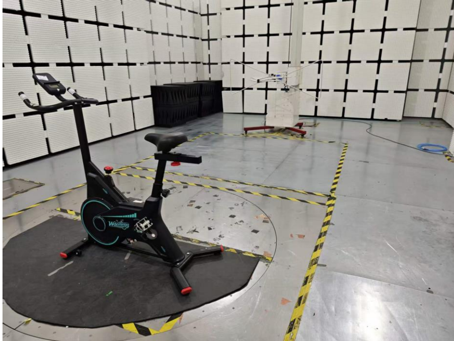
Set-up for Radiated Spurious Emission, Above 1GHz
