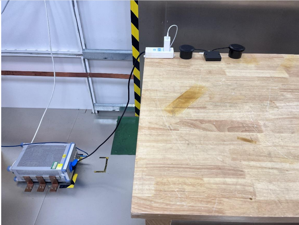
AC Power Line Conducted Emission
