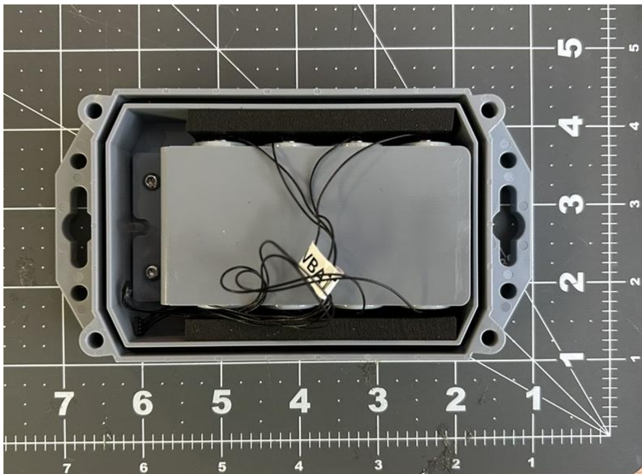
Battery Bank Only, No PCB components reside here.
