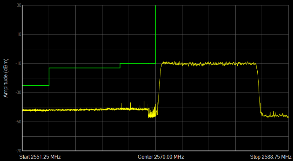
Band38 16QAM BW=15MHz Channel=37825 RB Size=75 Position=#0
