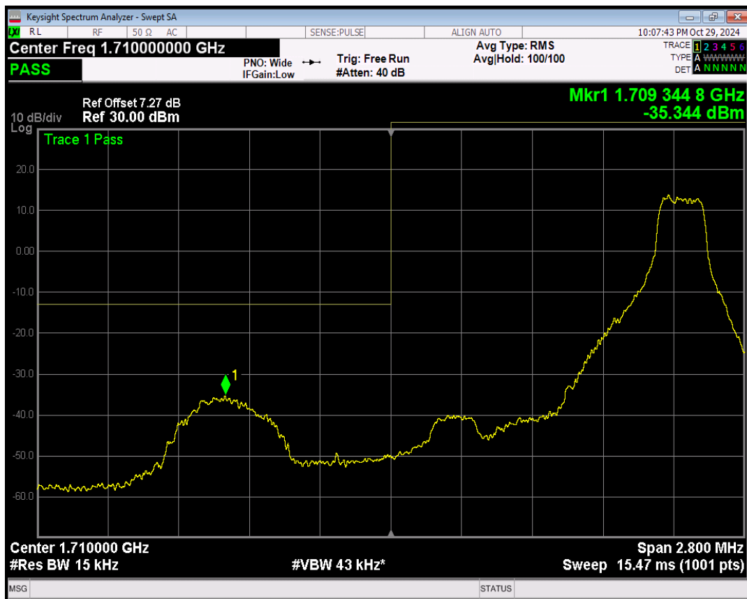
Band4 QPSK BW=1.4MHz Channel=19957 RB Size=6 Position=#0
