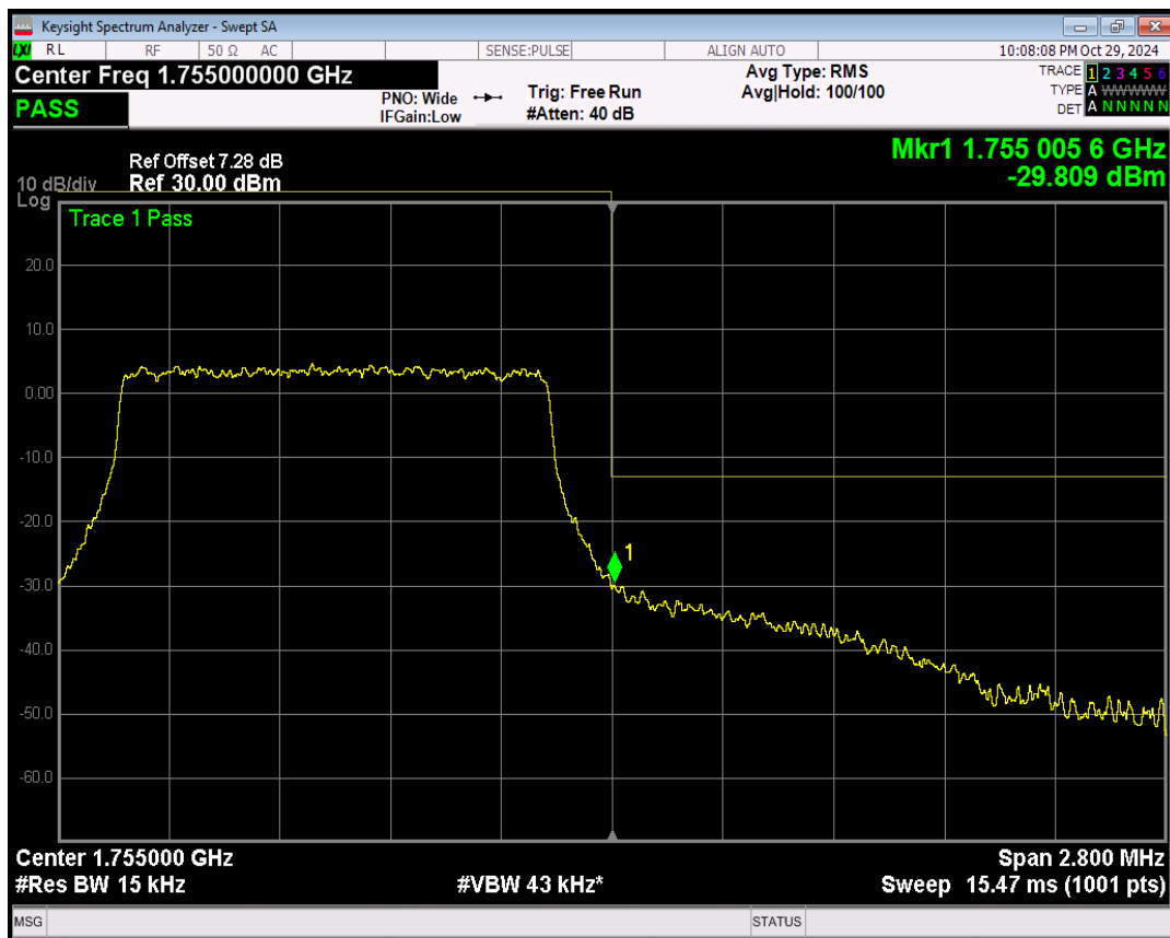
Band4 16QAM BW=1.4MHz Channel=20393 RB Size=1 Position=#Max
