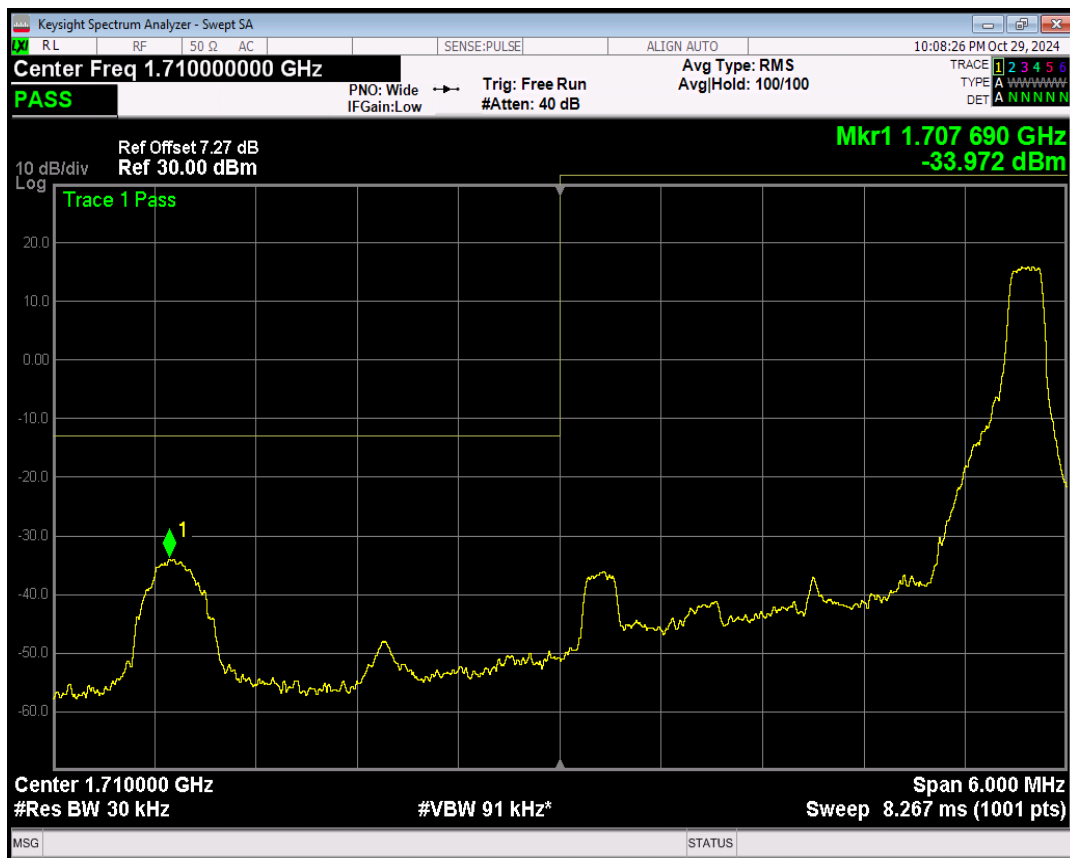
Band4 QPSK BW=3MHz Channel=19965 RB Size=15 Position=#0
