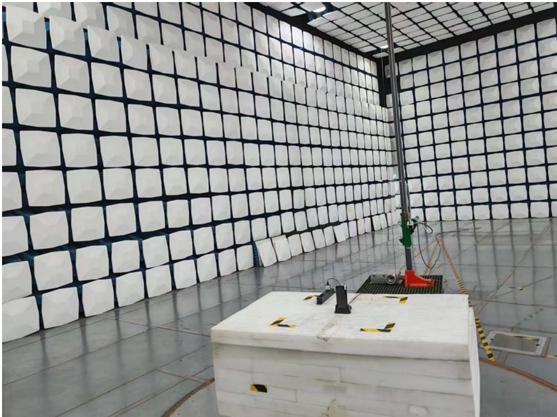
Radiated Emission 9k-30MHz Perpendicular View
