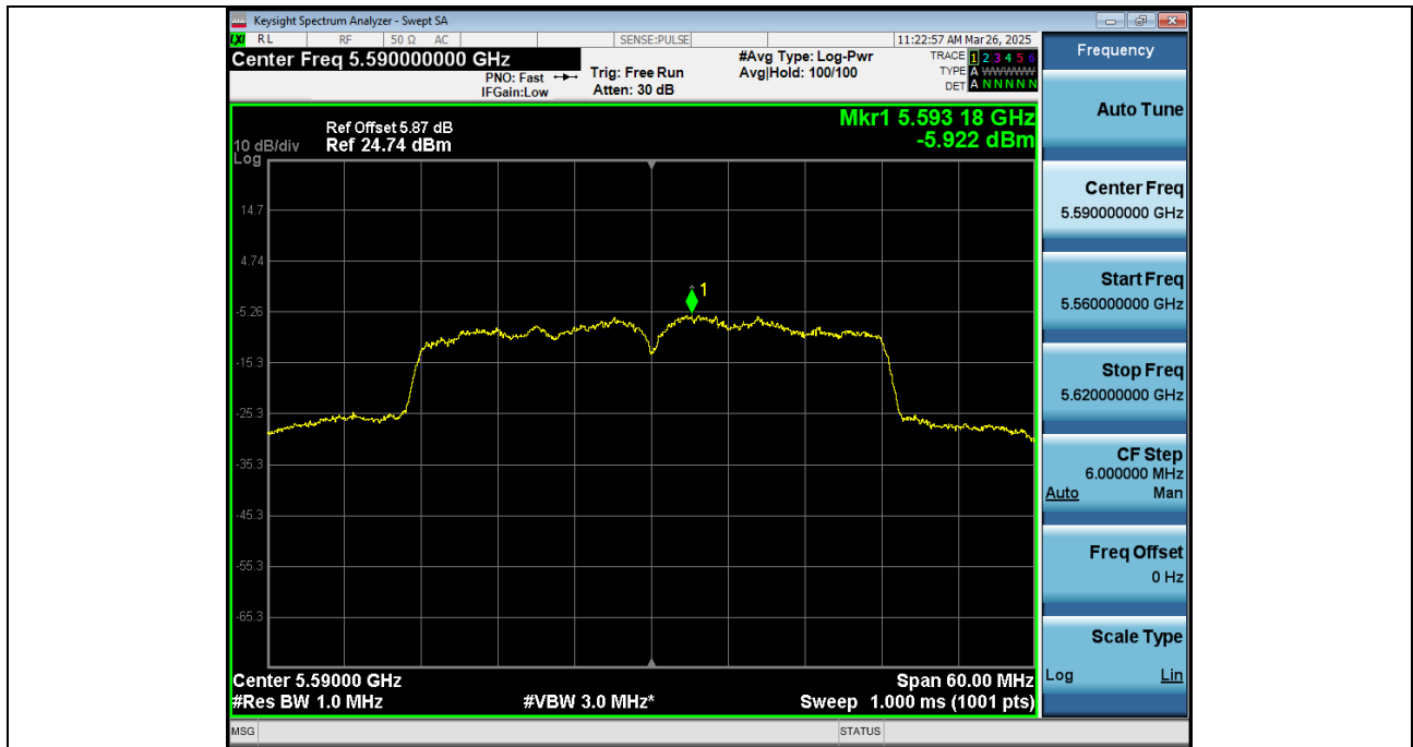
Power Spectral Density NVNT_ANT1_802_11n(HT40)_5670
