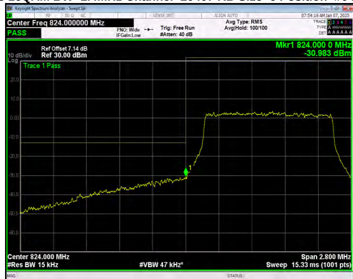
Band5 16QAM BW=1.4MHz Channel=20407 RB Size=6 Position=#0 Normal
