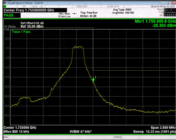
Band4 16QAM BW=1.4MHz Channel=20393 RB Size=6 Position=#0 Extended
