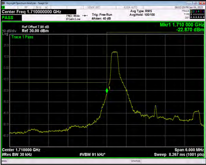
Band4 16QAM BW=3MHz Channel=19965 RB Size=1 Position=#Max Extended
