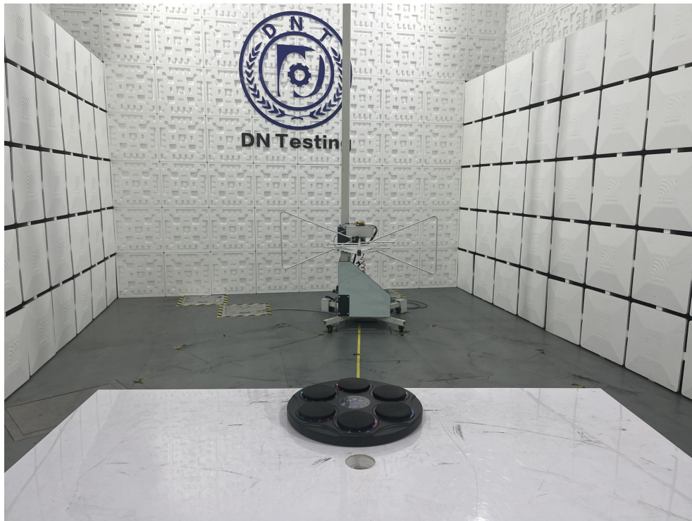
Radiated Emission Test View|(Below 1G)
