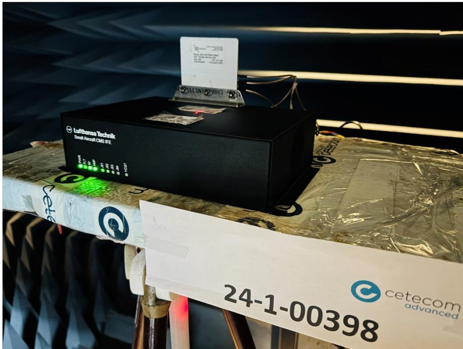
Photograph 7: EUT test setup in the fully anechoic chamber 2, close up view_EUT elevation 0°
