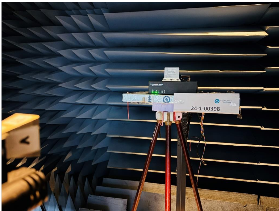
Photograph 8: EUT test setup in the fully anechoic chamber 2, overview_EUT elevation 0°
