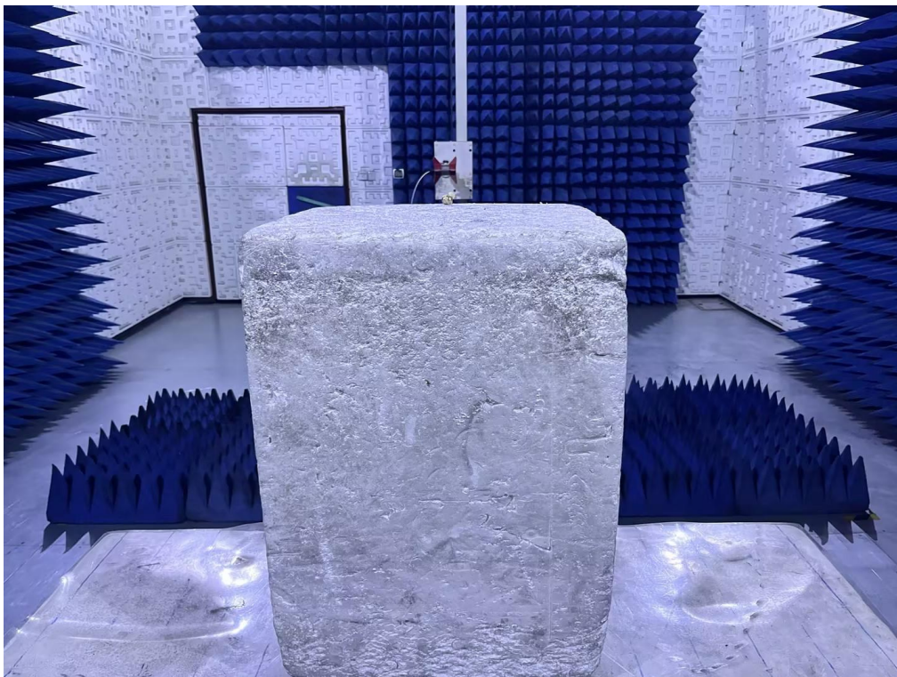
Radiated Emission Test Setup Above 1GHz-Right earphone
