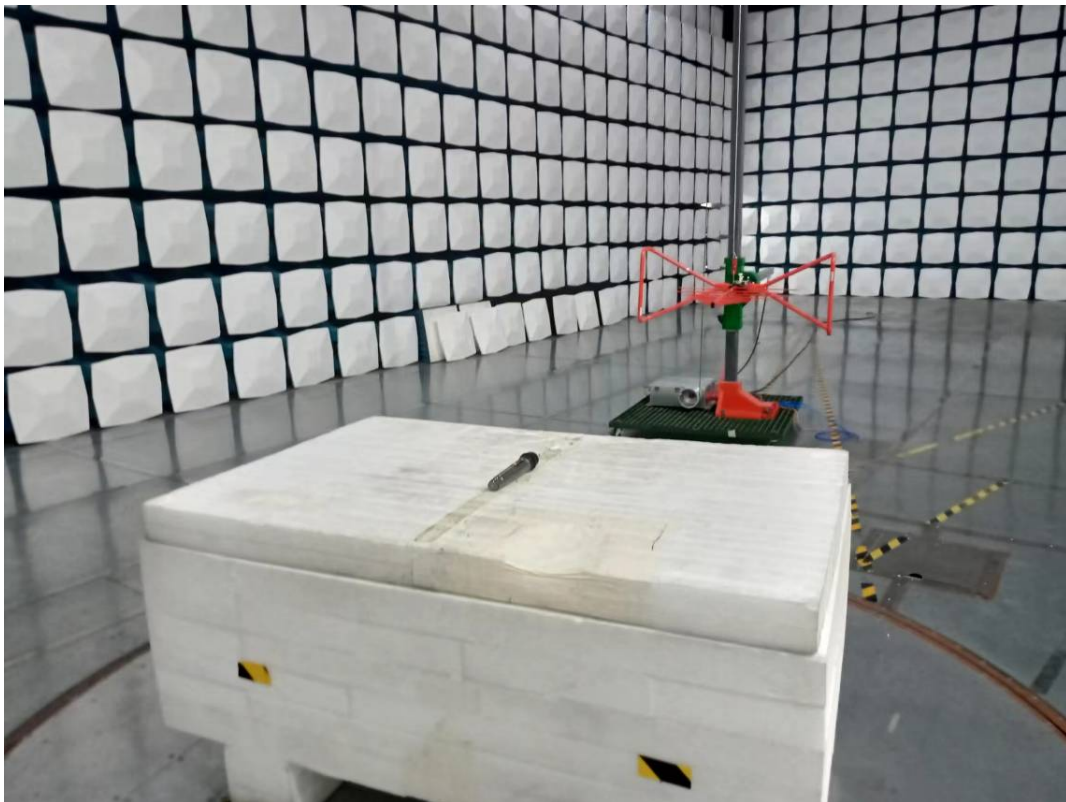
Radiated Emission 30M-1GHz View
