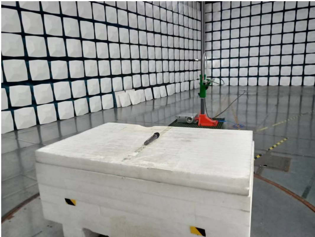
Radiated Emission 9k-30MHz Perpendicular View
