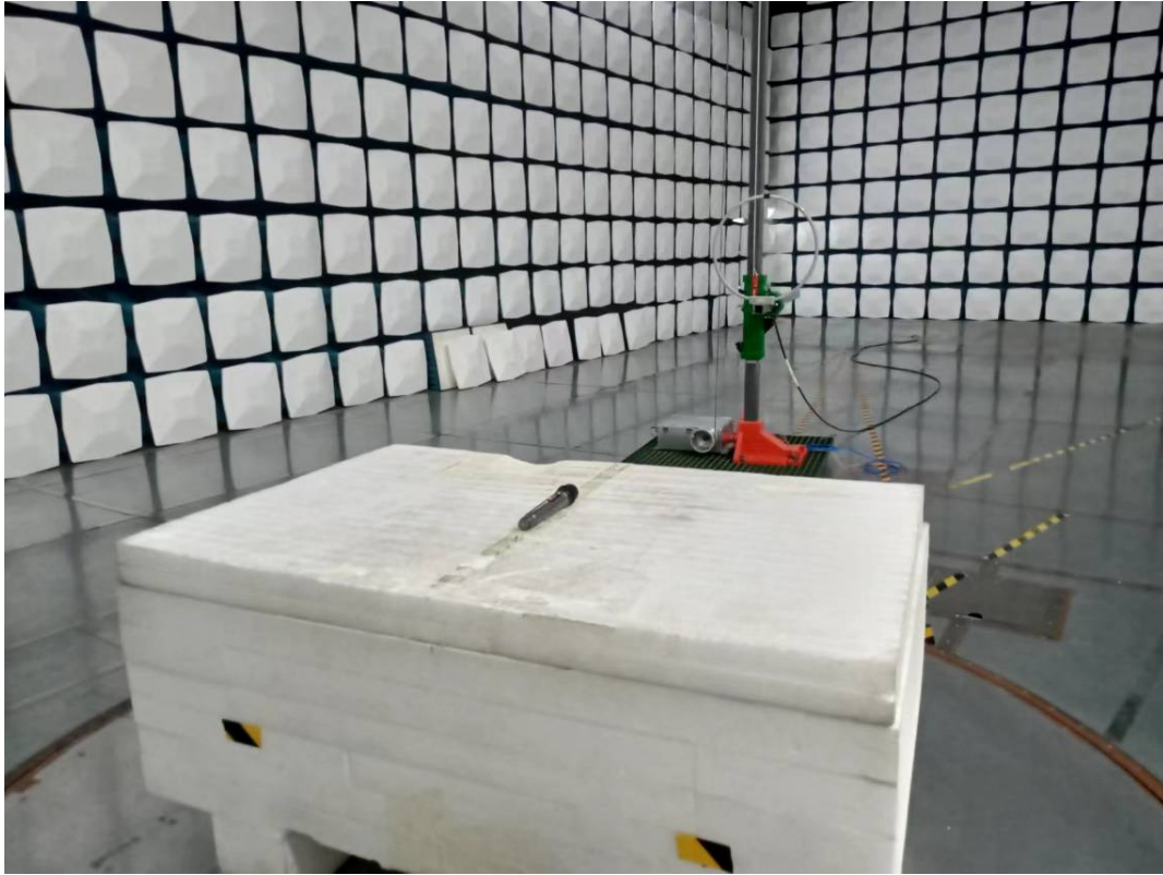
Radiated Emission 9k-30MHz Perpendicular View
