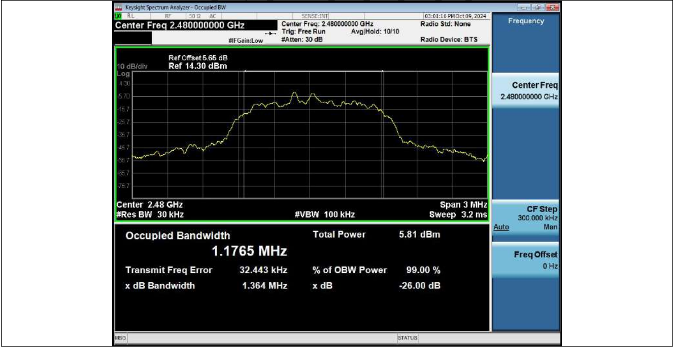
99% Occupied Bandwidth NVNT_ANT1_2-DH1_2480_00
