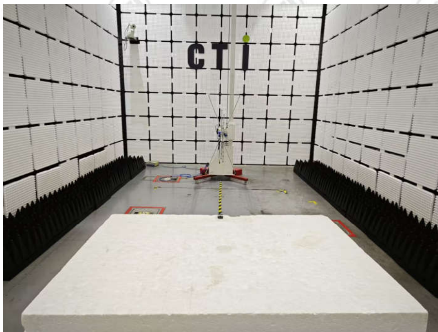
Radiated emission Test Setup-2 (30MHz~1GHz)
