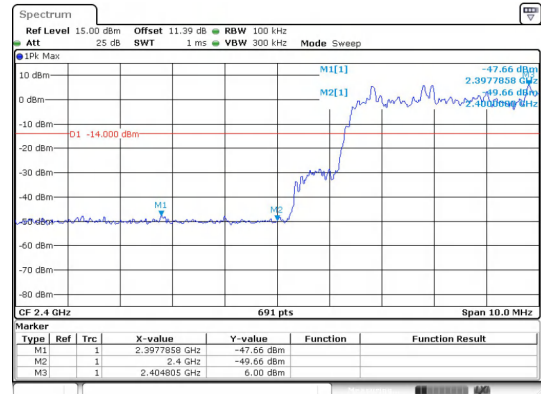
Out Of Band Emission(Left) \pi/4 DQPSK_2-DH5_Channel Hopping
