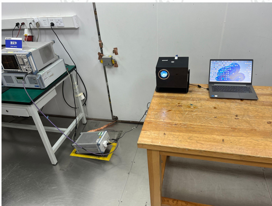
Conducted Emissions Test Setup
