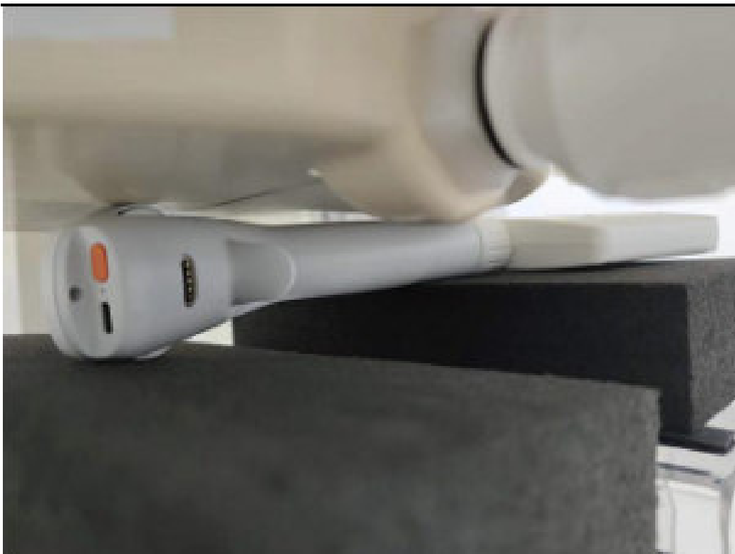
Picture 4: Left Edge2, the distance from EUT to the bottom of the Phantom is 0mm
