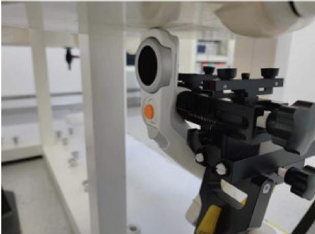
Picture 7: Top Edge, the distance from EUT to the bottom of the Phantom is 0mm
