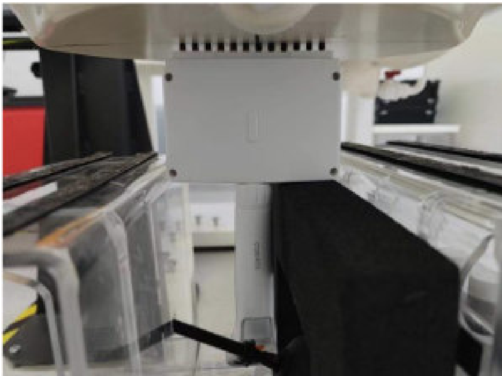
Picture 8: Bottom Edge1, the distance from EUT to the bottom of the Phantom is 0mm
