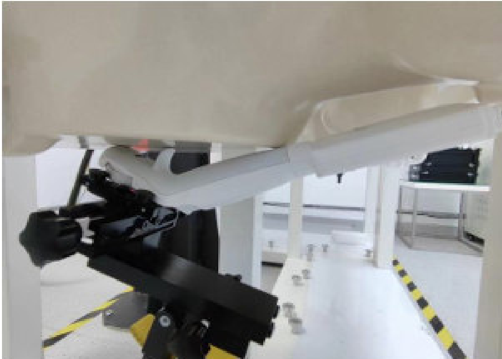
Picture 1: Back Side, the distance from EUT to the bottom of the Phantom is 0mm
