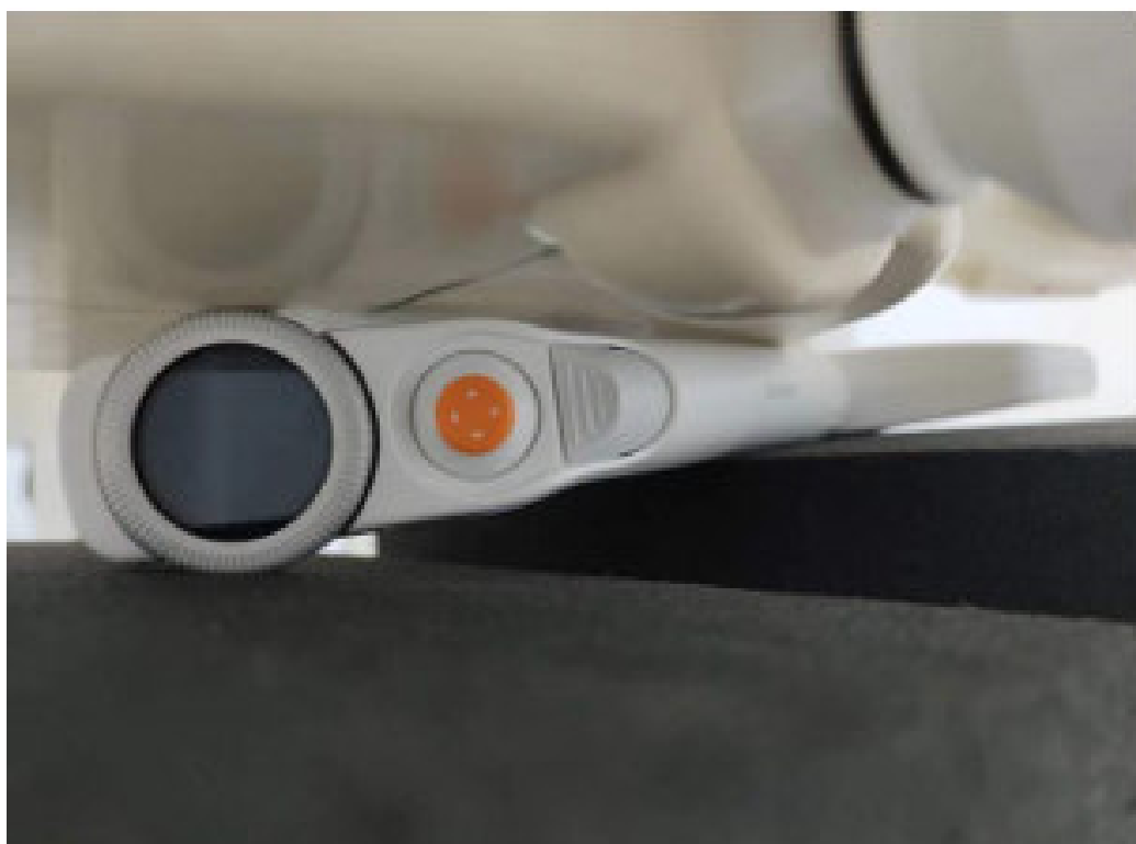
Picture 6: Right Edge, the distance from EUT to the bottom of the Phantom is 10mm
