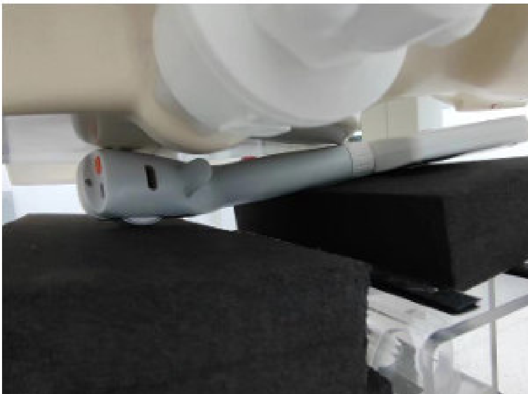
Picture 5: Left Edge3, the distance from EUT to the bottom of the Phantom is 0mm
