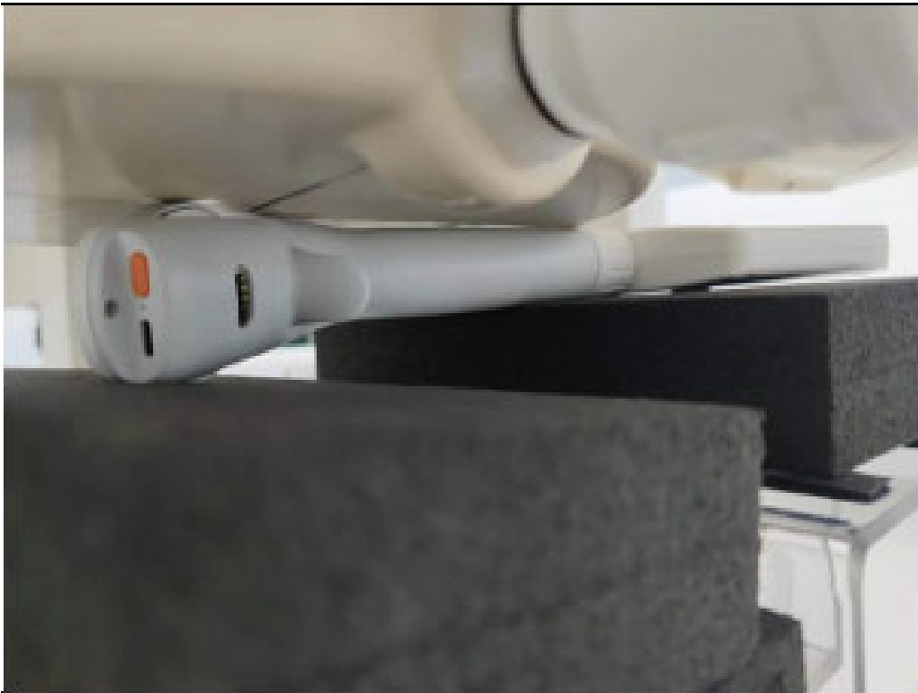
Picture 3: Left Edge1, the distance from EUT to the bottom of the Phantom is 0mm
