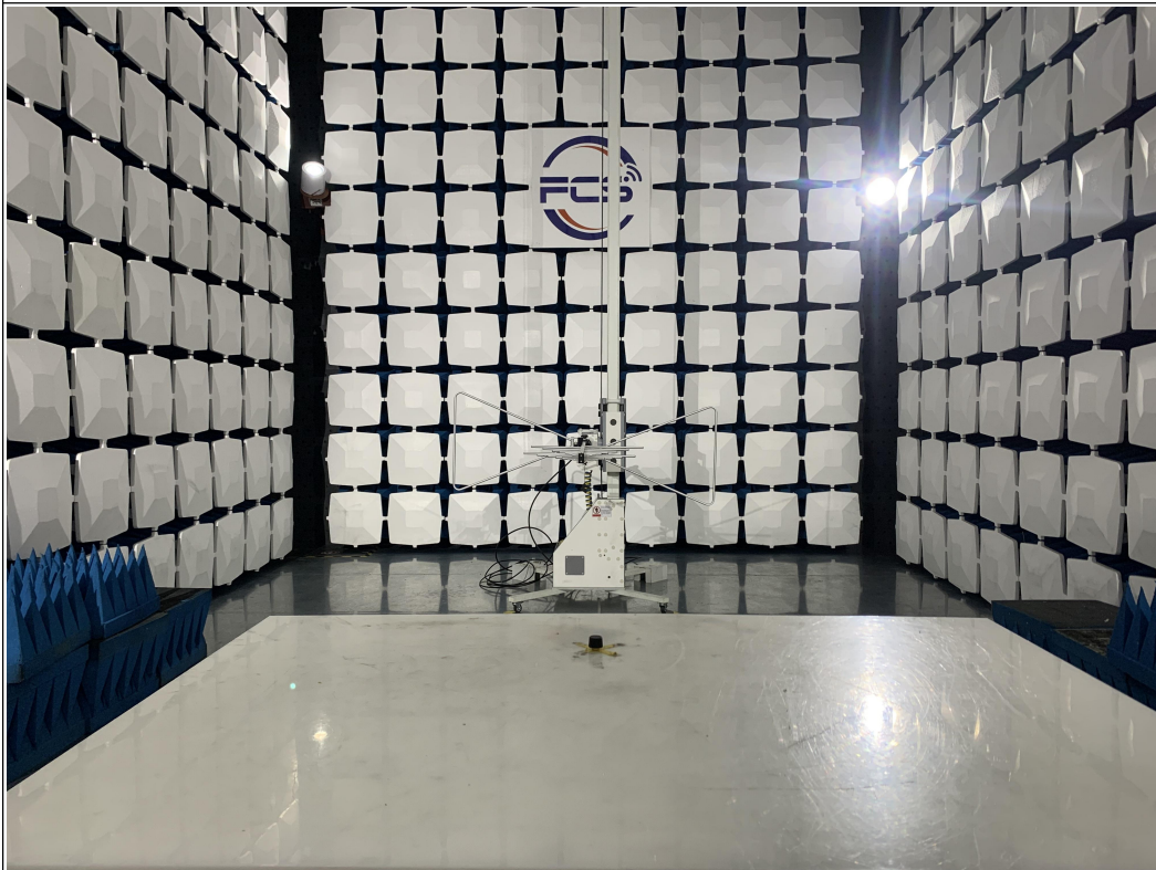
Above 1GHz for radiated emission test setup
