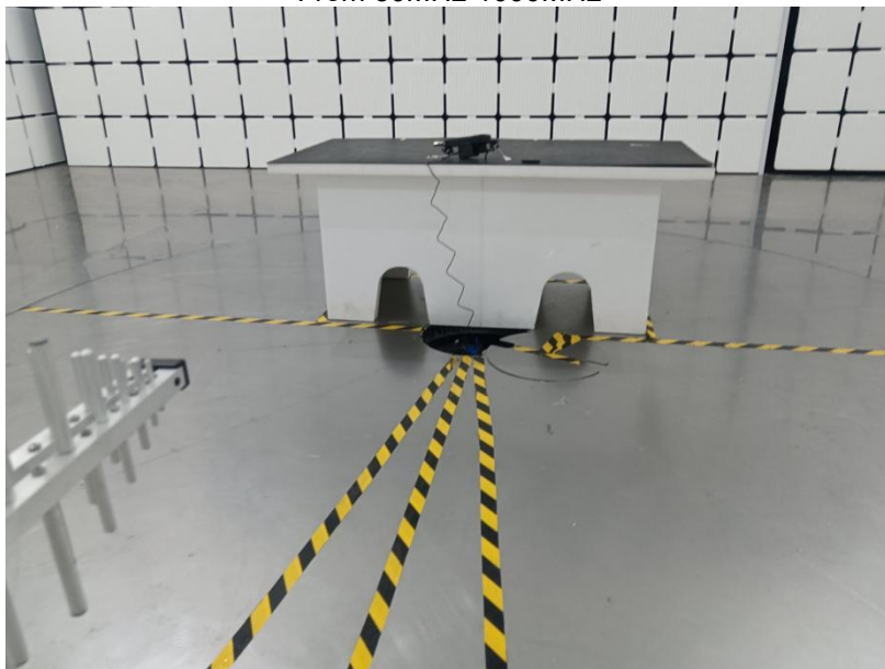
Radiated Spurious Emissions From 30MHz-1000MHz
