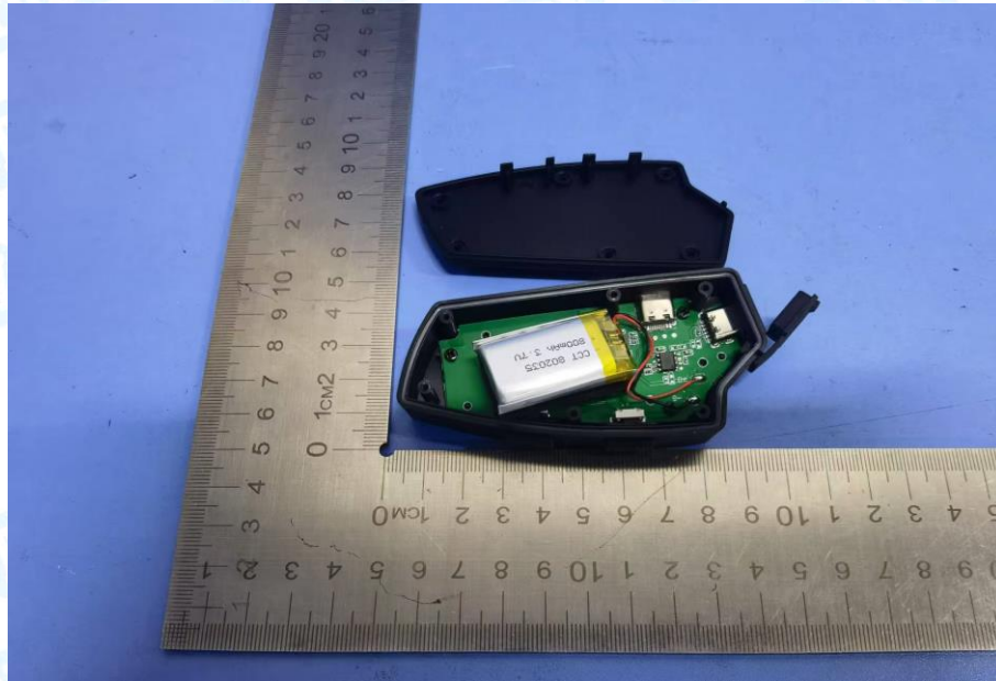
Photo 8 Appearance of PCB & Battery
