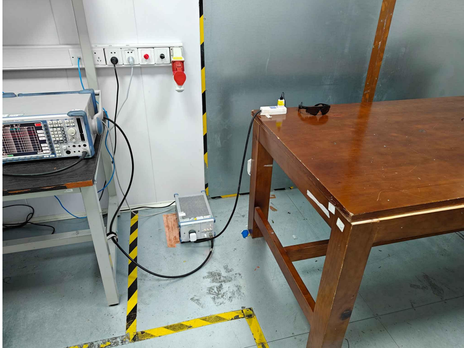
Conducted emissions at AC power line (150kHz-30MHz)
