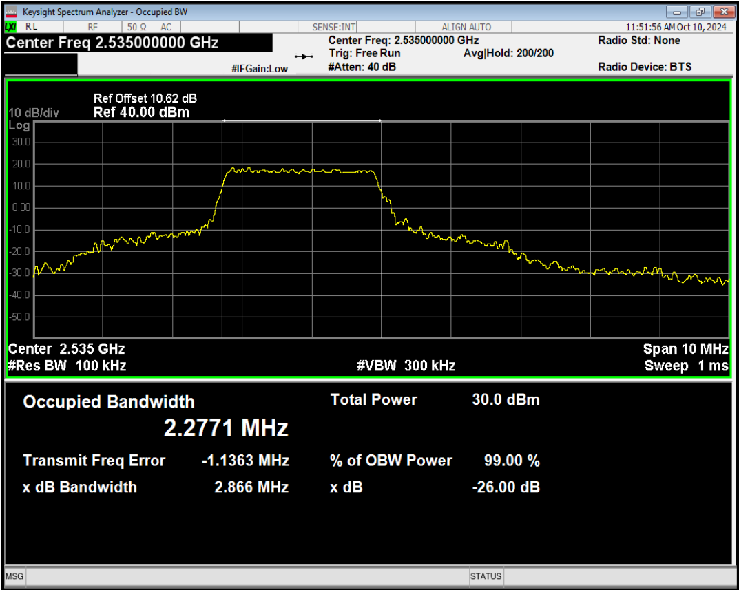
Band7 QPSK BW=5MHz Channel=21100 RB Size=12 Position=#0
