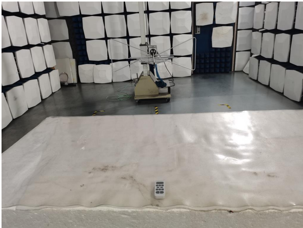
Radiated Emission Test Setup:
