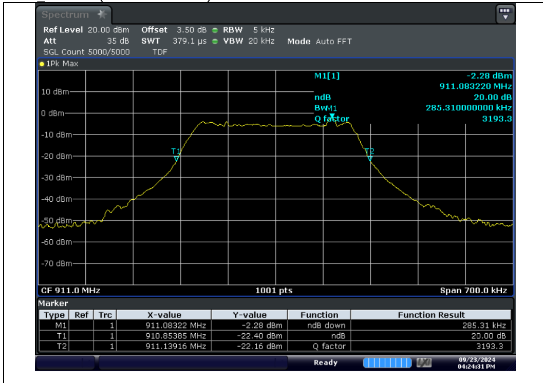
FSK 911 MHz(20 dB Bandwidth)
