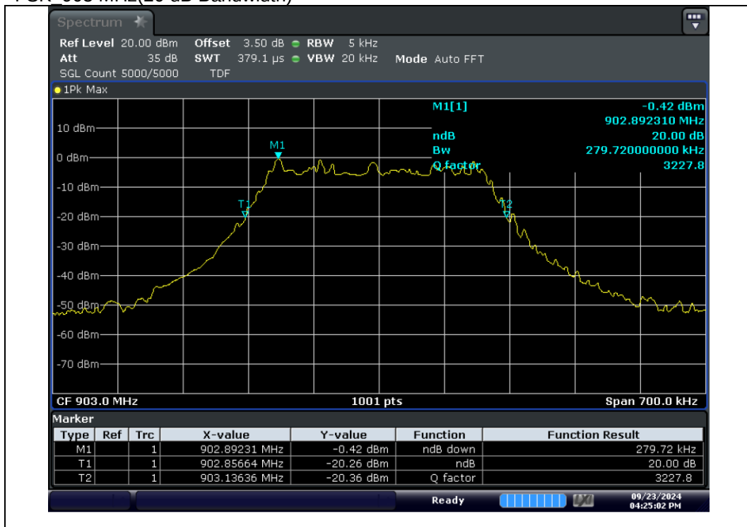
FSK 903 MHz(20 dB Bandwidth)
