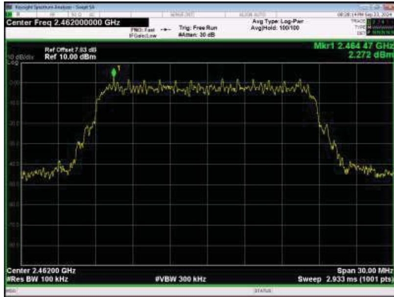
Tx. Spurious NVNT 802.11n(HT20) 2462MHz Ant1 Emission
