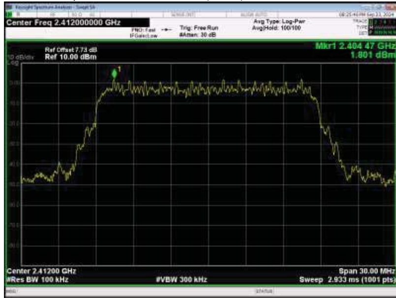
Tx. Spurious NVNT 802.11n(HT20) 2412MHz Ant1 Ref
