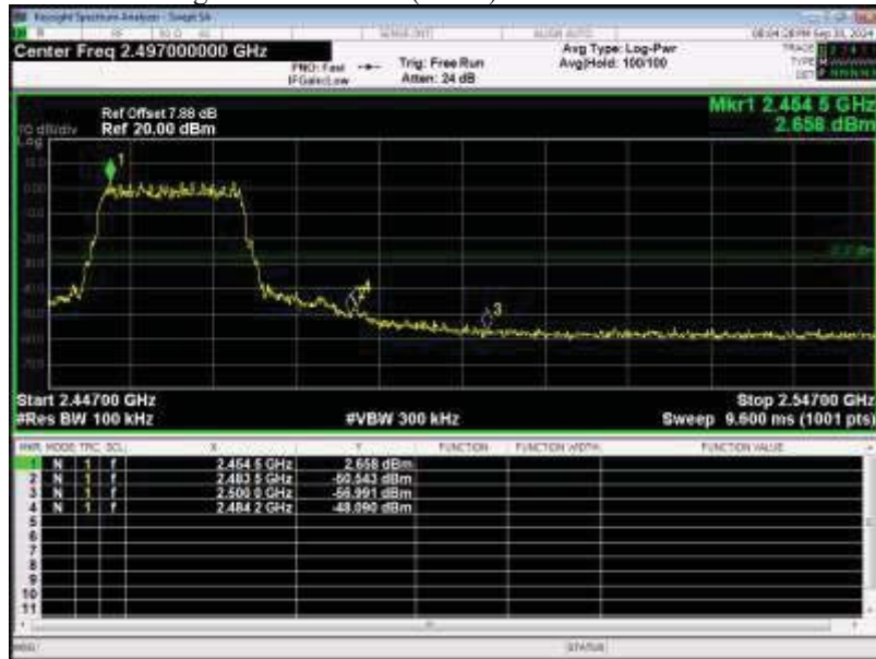
Band Edge NVNT 802.11n(HT20) 2462MHz Ant1 Emission
