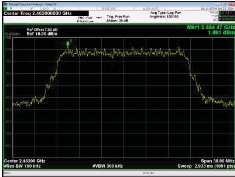
Tx. Spurious NVNT 802.11b 1Mbps 2462MHz Ant1 Emission
