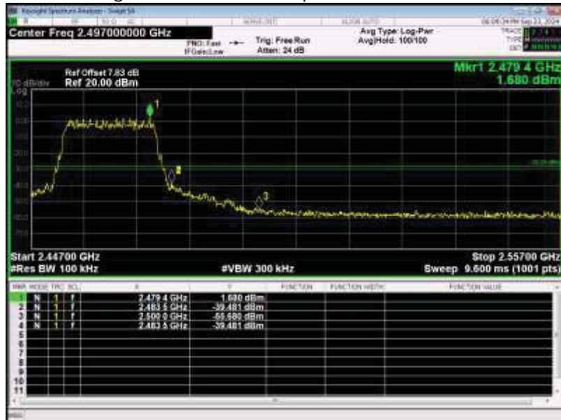
Band Edge NVNT 802.11b 1Mbps 2462MHz Ant1 Emission
