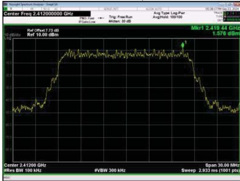
Tx. Spurious NVNT 802.11b 1Mbps 2412MHz Ant1 Emission
