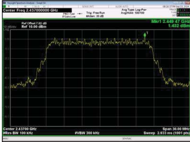
Tx. Spurious NVNT 802.11n(HT20) 2437MHz Ant1 Emission
