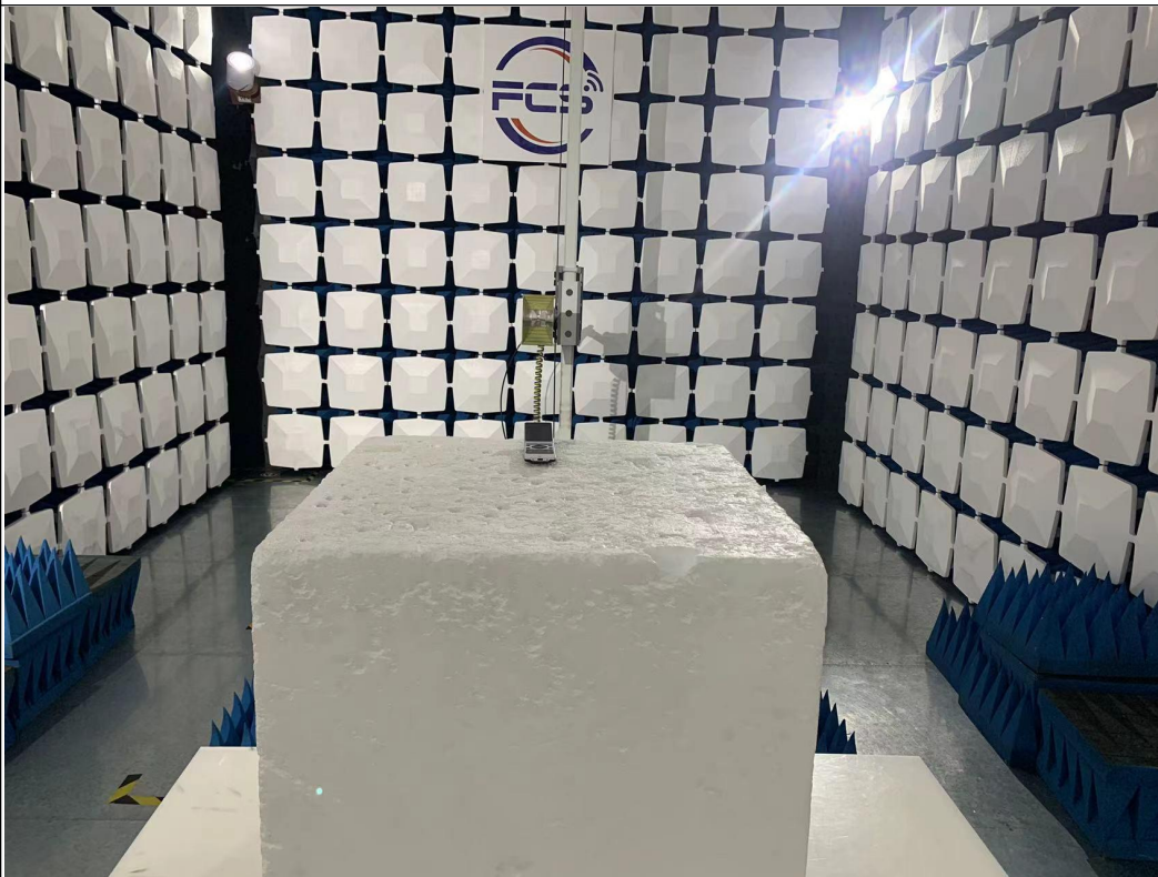
Above 1GHz for radiated emission test setup
