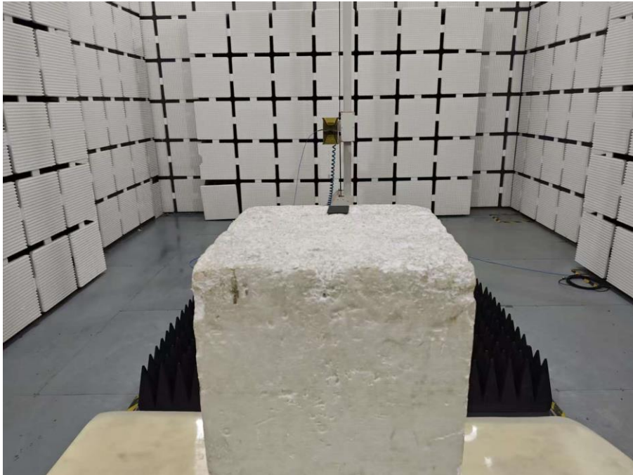
Set-up for Radiated Spurious Emission, Above 1GHz
