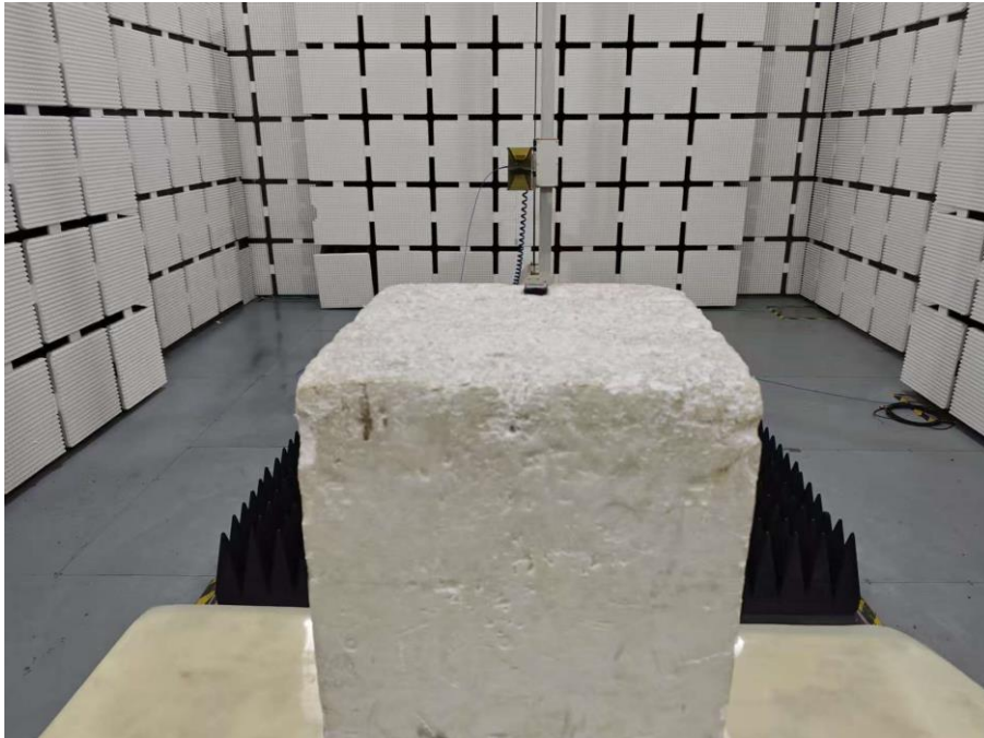
Set-up for Radiated Spurious Emission, Above 1GHz
