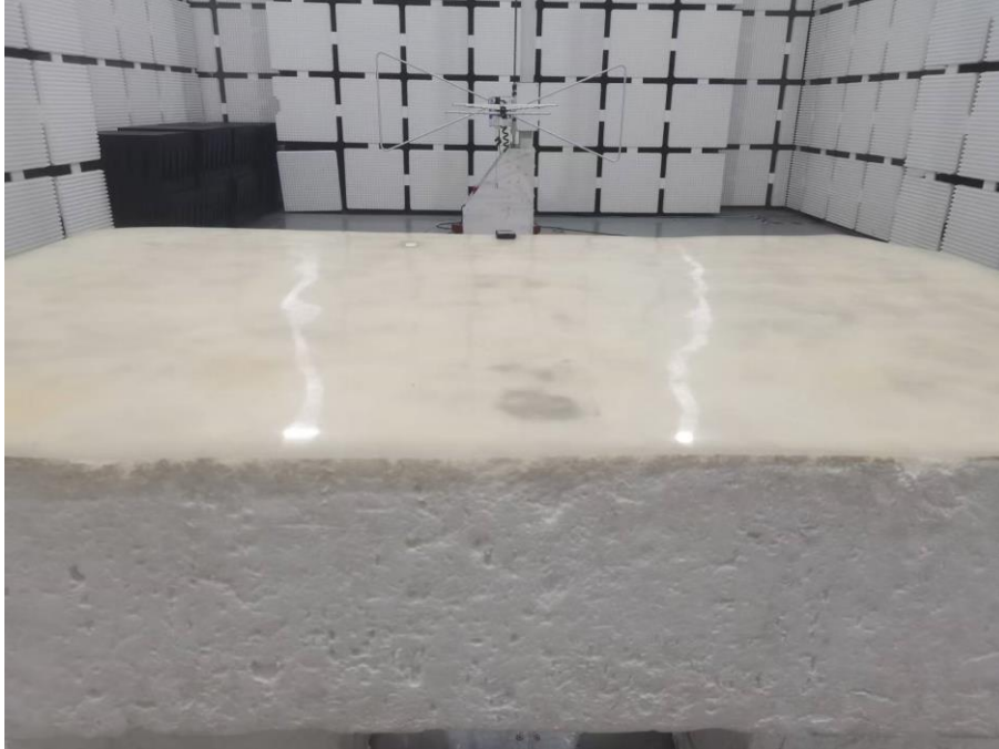
Set-up for Radiated Spurious Emission, Above 1GHz
