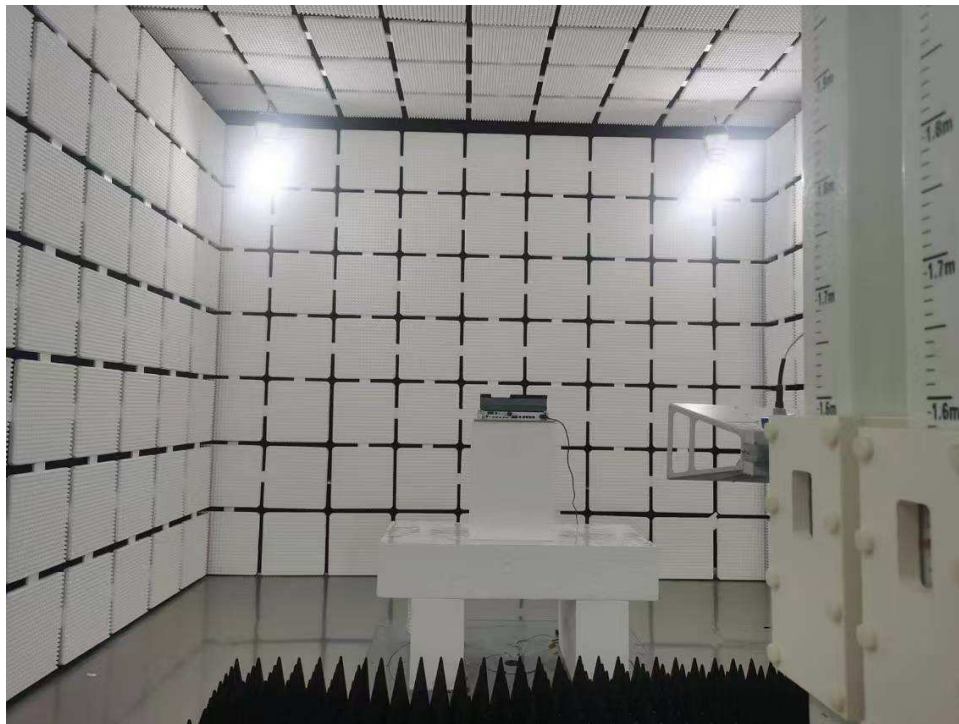
Photograph 1: Set-up photo for Radiated Spurious Emission
