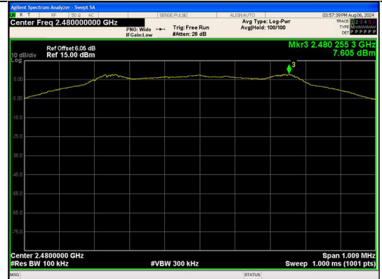
In-Band Reference Level BLE 1M_Channel 39
